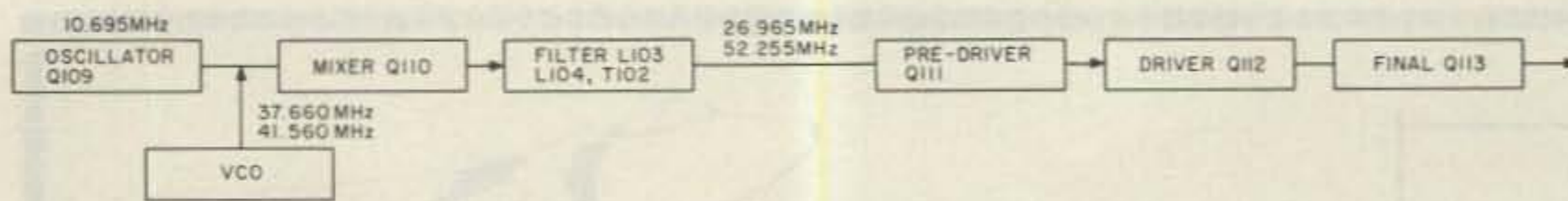
Fig. 4. Hy-Gain transmitter block diagram.
