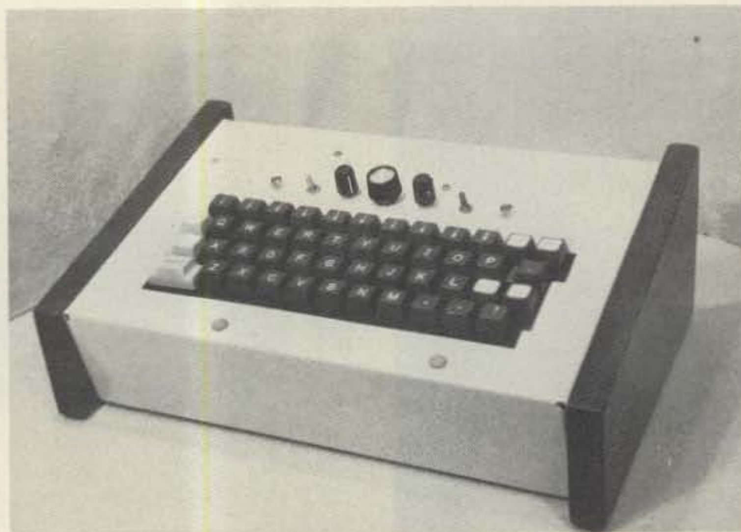
Photo E. A hybrid cabinet using a chassis base and wood end pieces to support a home-brew CW keyboard.
