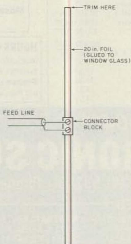
Fig. 1. Half-wave two-meter foil antenna.
