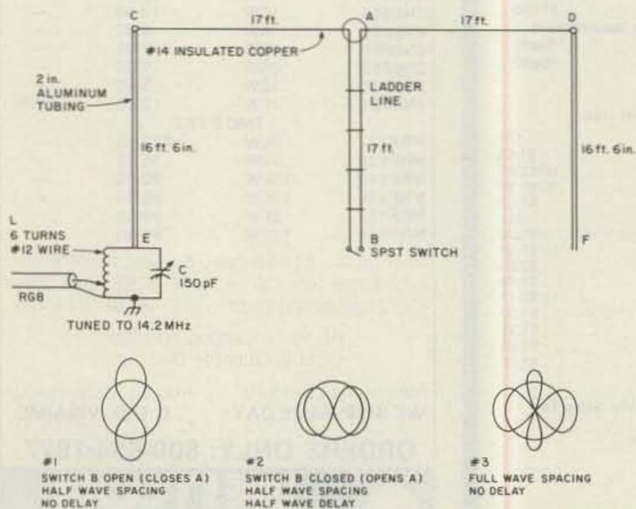
Fig. 1. Switching diagram.
