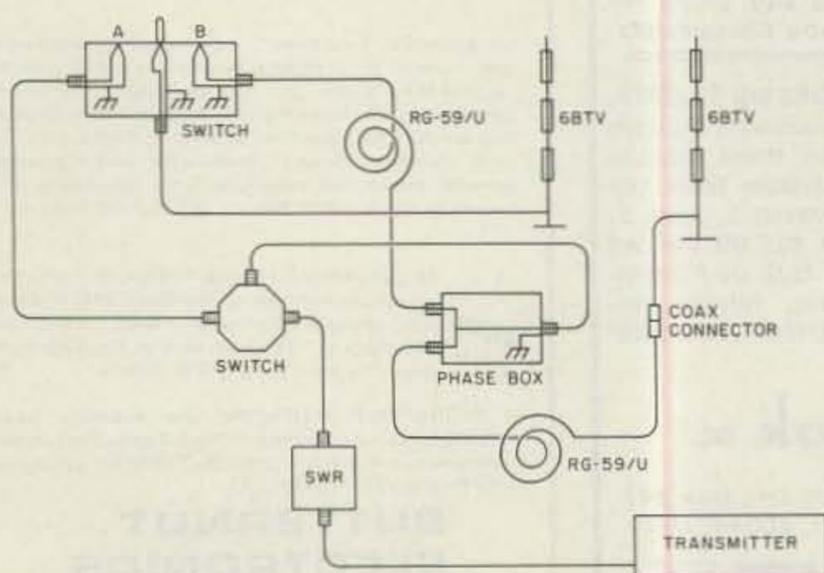
Fig. 1. Phased-vertical system diagram.
