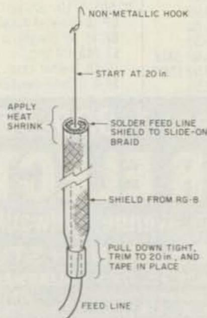
Fig. 2. Half-wave two-meter flexible antenna.
