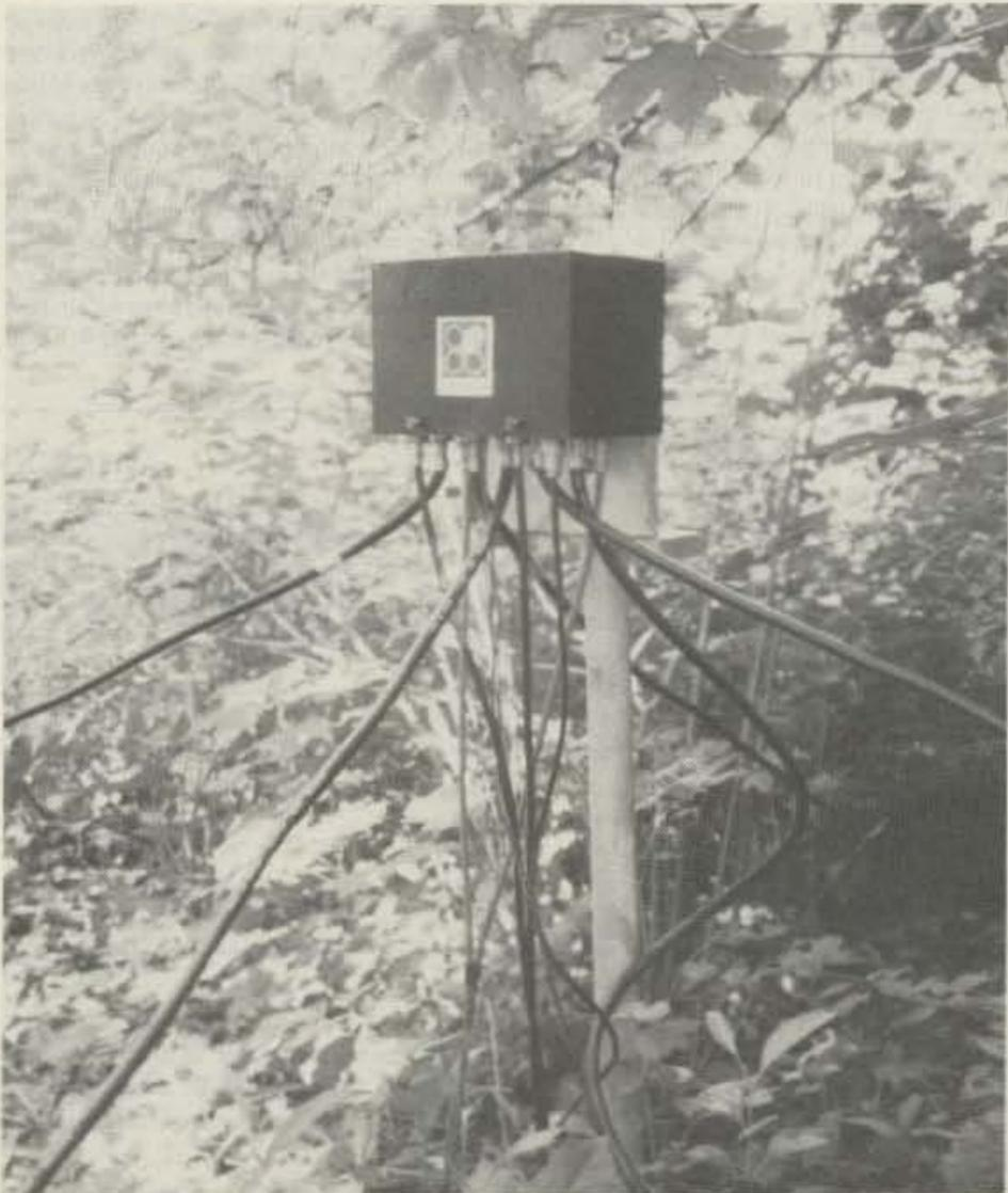
Photo B. Outdoor relay box mounted on owner-supplied pipe. SO-239 connectors are protected from the weather, but ColAtchCo recommends a plastic trash can, too. Phasing lines came pre-cut. No dummy load is evident because I ran an RG-58 line back into my cellar where I put a Heathkit Antenna.
