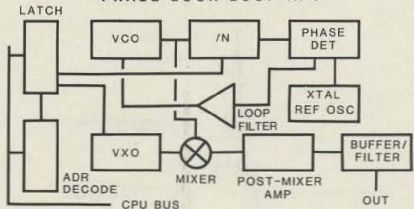
THE DFS-1 CAN BE USED AS THE HEART OF A HF SYNTHESIZED TRANSCEIVER DESIGN OR AS A SECOND VFO FOR EXISTING RIGS
