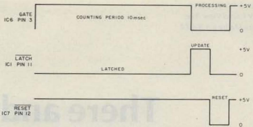
Fig. 5. Control timing diagram.
