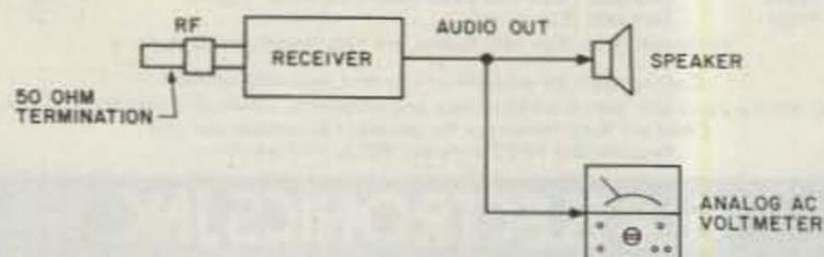
Fig. 1. Basic noise test setup.
