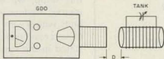
Fig. 1. Typical setup for finding resonant frequency of unknown tank circuit. Meter suddenly "dips" as circuit is tuned to oscillator frequency.
