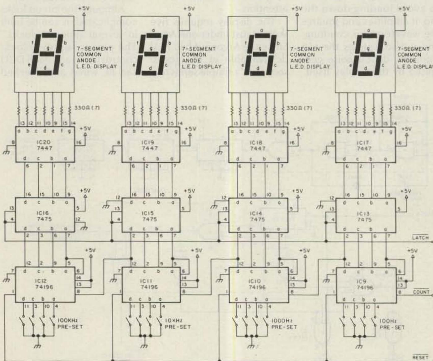
Fig. 4. Counter and display logic.
