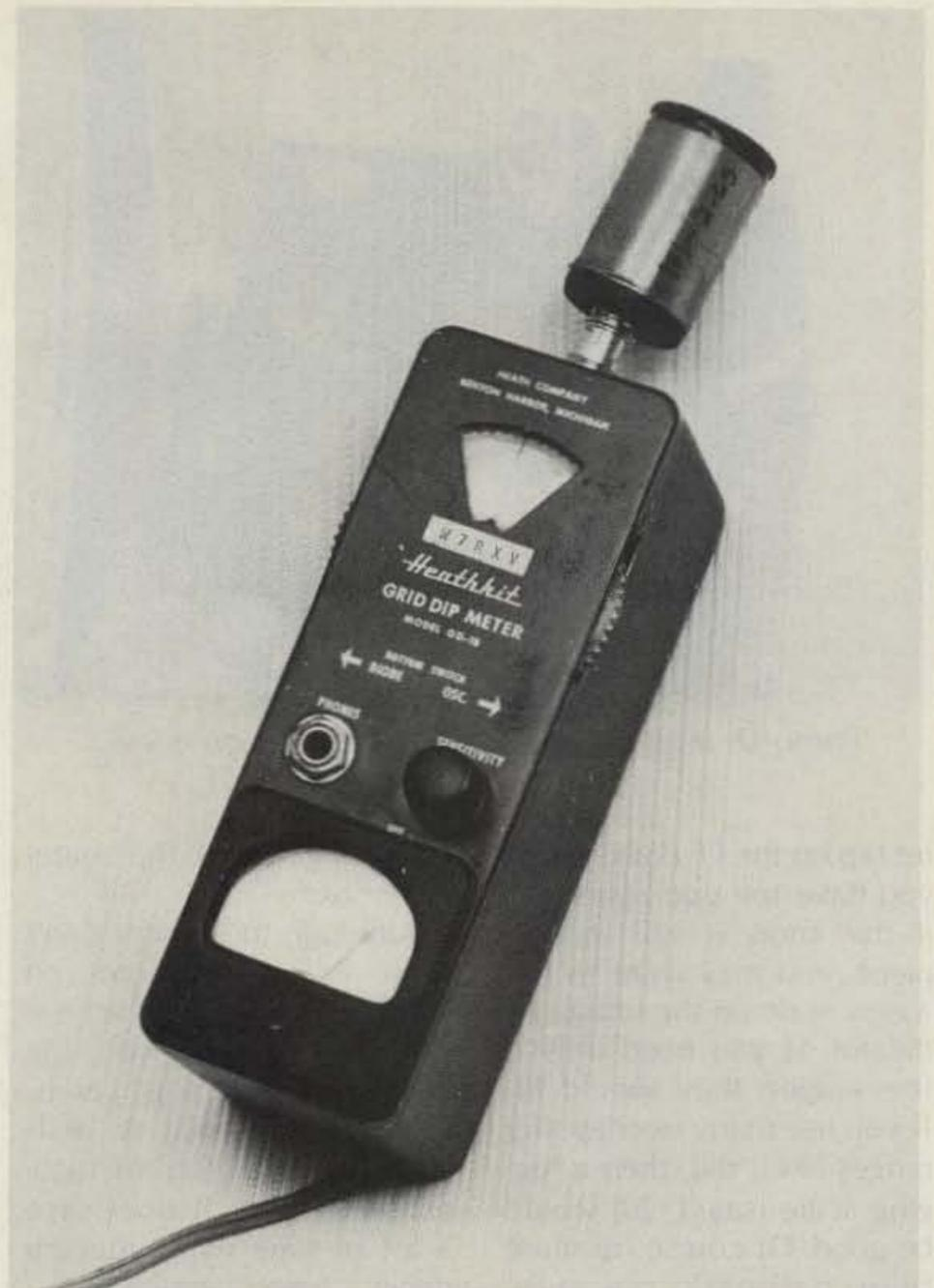
Photo A. By adding an F connector and winding coils on plastic film cans you can recycle older grid-dip meters when you can't get the original coils.
