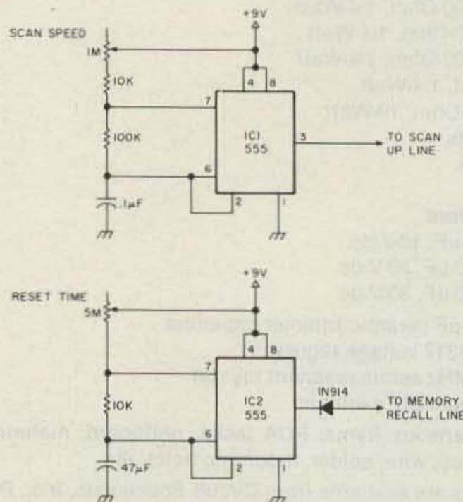
Fig. 2. Simple scan and reset circuit.
