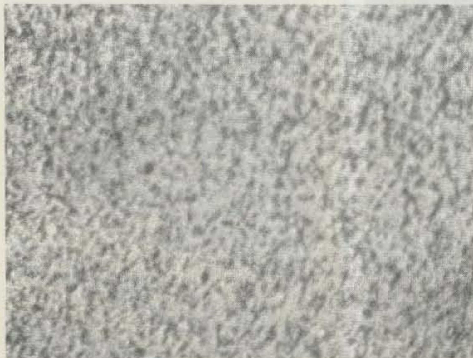
Plane polarized light at 100× magnification. A well-polished disk with good oxide distribution.
