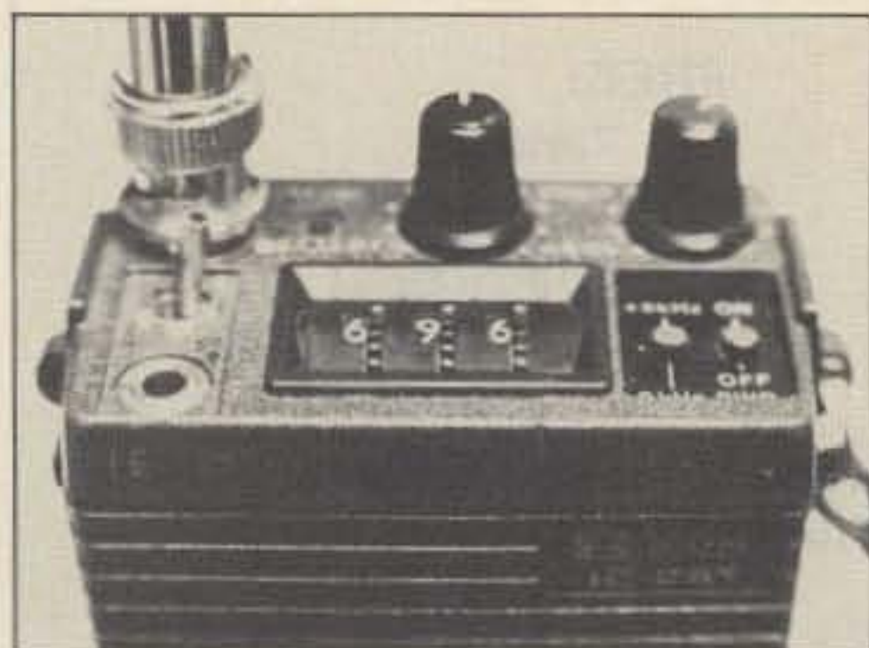
Photo A. Install the range switch in the microphone jack position.
