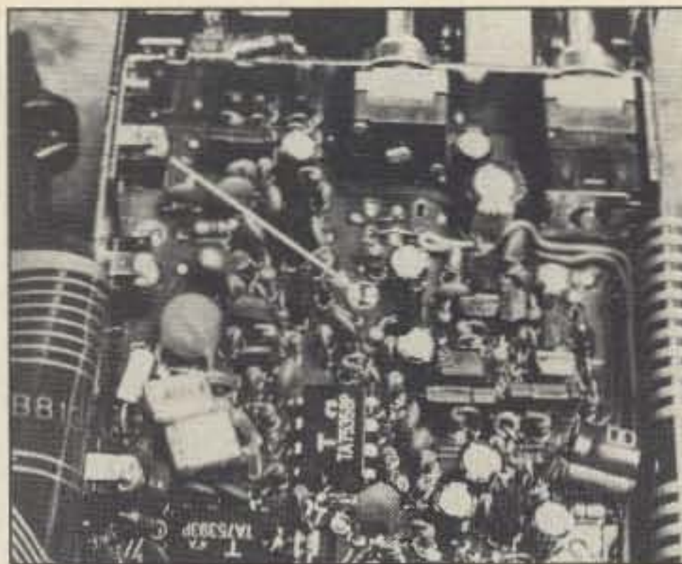
Photo D. Snipping C117 (see arrow) will boost the audio sent to the speaker.
