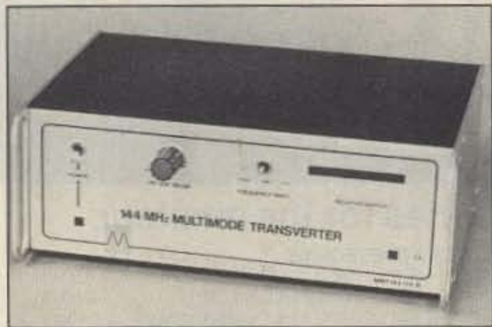
Photo D. Microwave Modules' MMT 144/28 R 2m multimode transverter.
