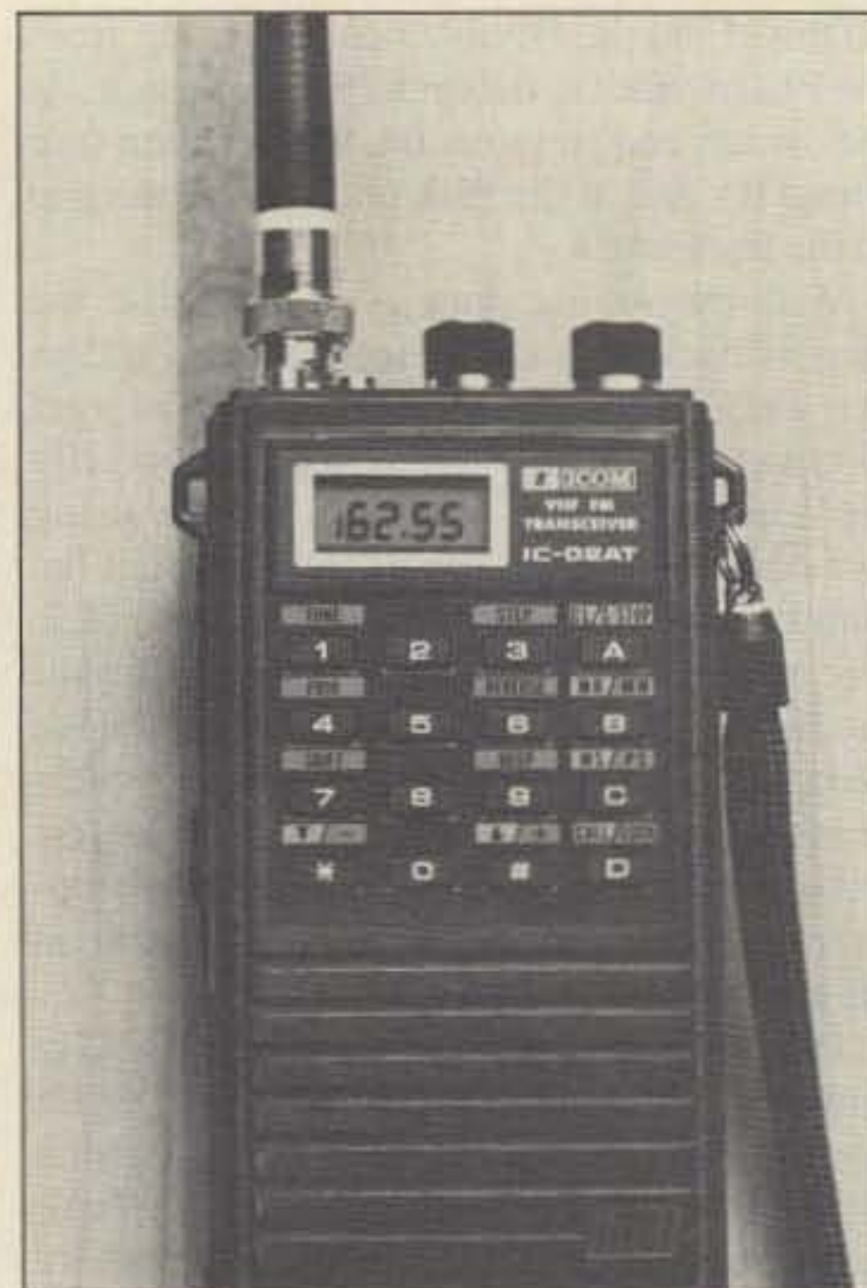
Photo E. The fruit of your labor—an 02AT receiving weather broadcasts on 162.55 MHz.
