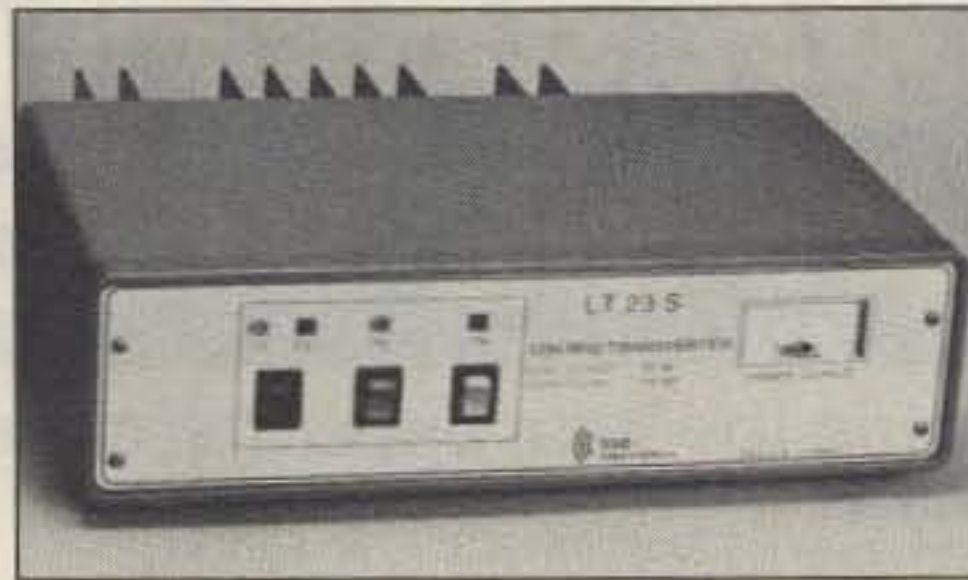
Photo E. The LT 23 S 1296-MHz transverter from SSB Electronics.
