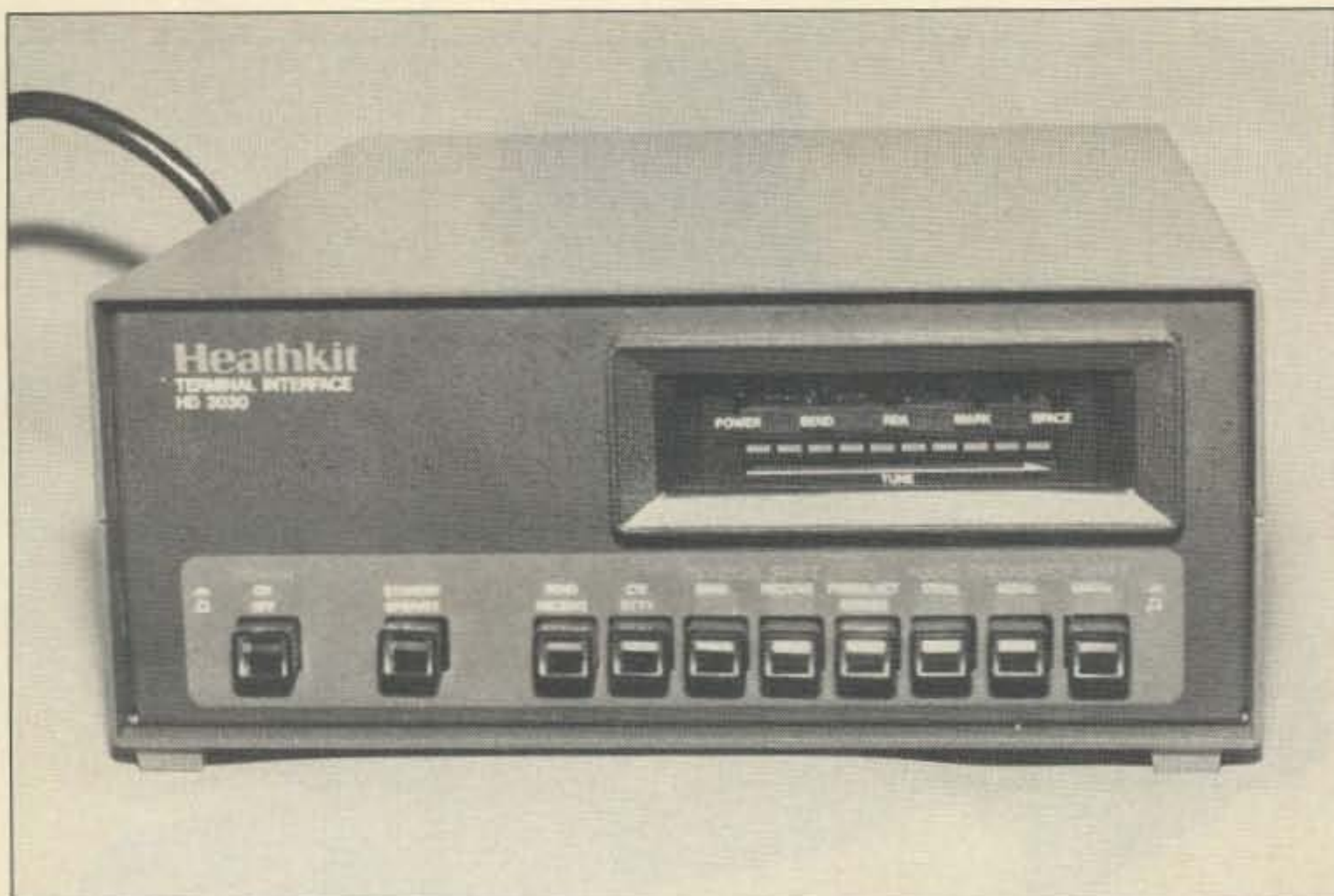
Photo A. The Heathkit HD-3030 RTTY/CW interface.
