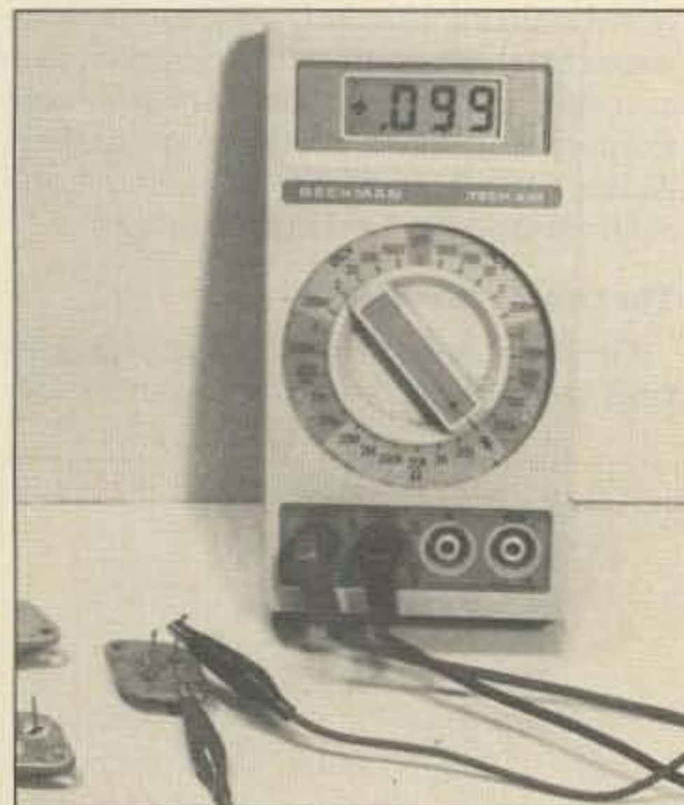
Photo F. A leaky transistor may show a low reading between any two elements in both directions. Here, a 99-Ohm leakage is found between the collector and emitter terminals of an audio-output transistor.
