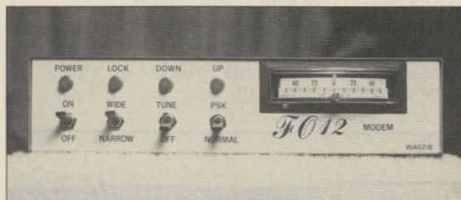
Photo C. Home-brew Fuji-OSCAR 12 modem using the G3RUH circuit board. The modem interfaces the radio to a standard packet TNC for mode "JD."
