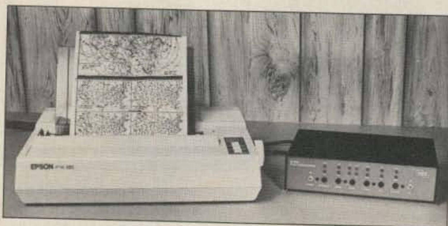
Photo C. The Info-Tech M-800 FAX converter and an Epson FX-85 printer. Photograph courtesy of Universal Shortwave Radio.
