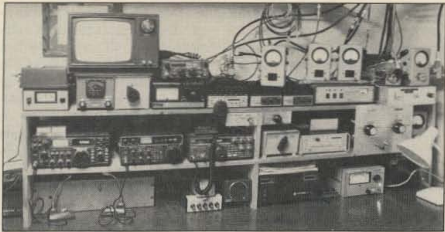
Photo A. Here's a front view of the operating position at KT2B. HF transceivers and VHF exciters are on the left side, while transverters and VHF/UHF amplifiers are on the right.
