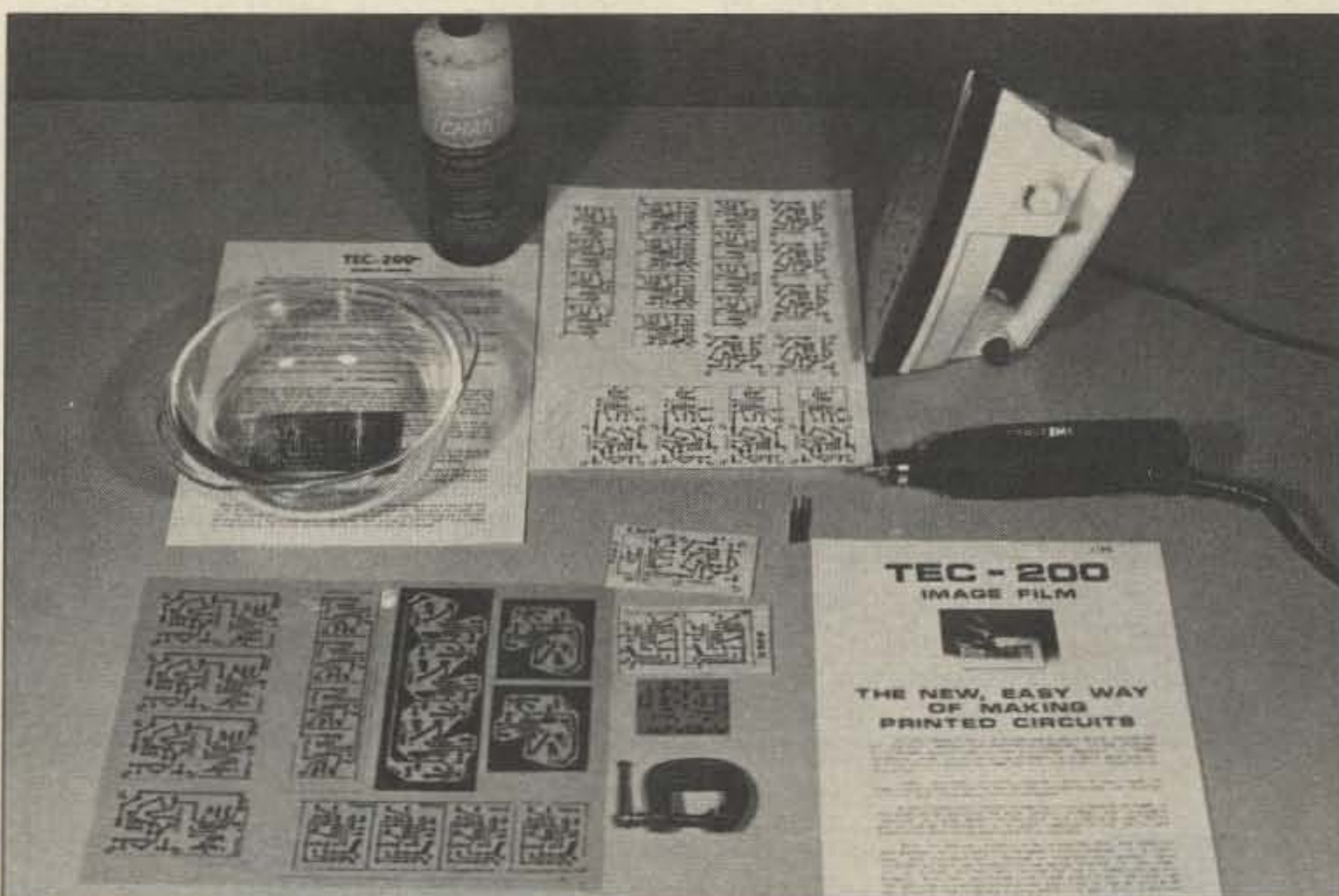
Photo A. A minimum of materials are needed to fabricate your own printed circuit boards. At the lower left is a completely filled sheet of TEC-200 film ready for transfer to copperclad board.
