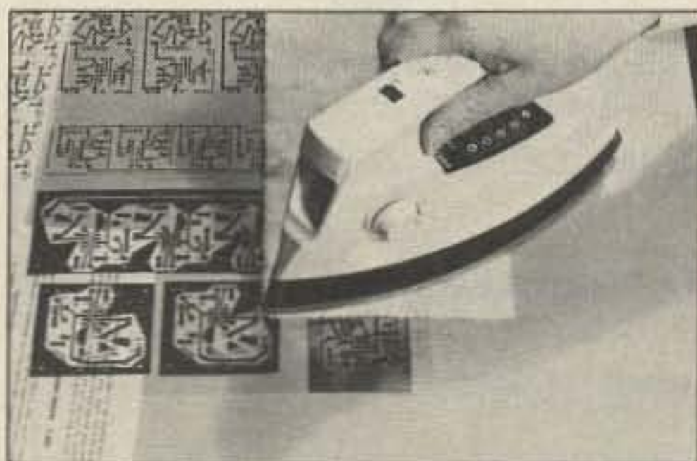
Photo B. An iron set for cotton (265°F to 295°F) is used to transfer the circuit design from the TEC-200 film to the copperclad board.
