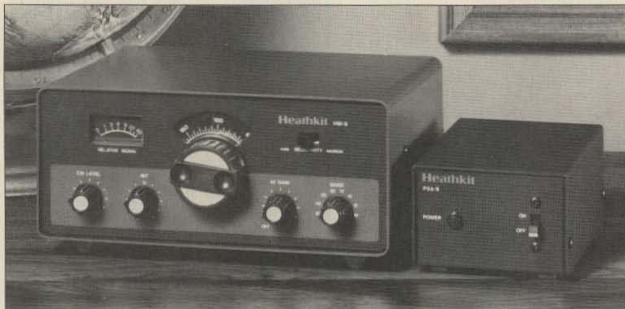
Photo A. The Heath HW-9 shown with the optional PSA-9 power supply.
