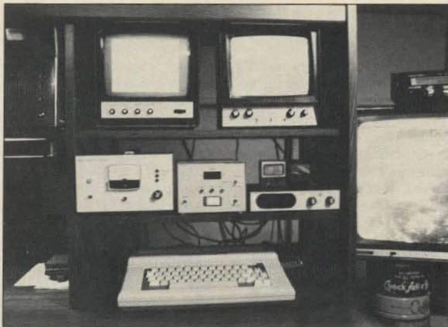
Photo B. Jack Hawkins' (WB6WJQ) scan converter-based satellite station. The 512K Radio Shack Color Computer 3 (lower center) handles the imaging chores in conjunction with Jack's version of the WSH scan converter in the cabinet on the left side of the middle shelf. The cabinet at the center of the middle shelf contains the station power supply and the station antenna control while the Hamtronics R75A custom-packaged kit receiver is on the right. The upper shelf has two monitors, one for the computer menu (left), and the other to view the output of the scan converter, like the large-screen monitor to the right of the shelf unit.
