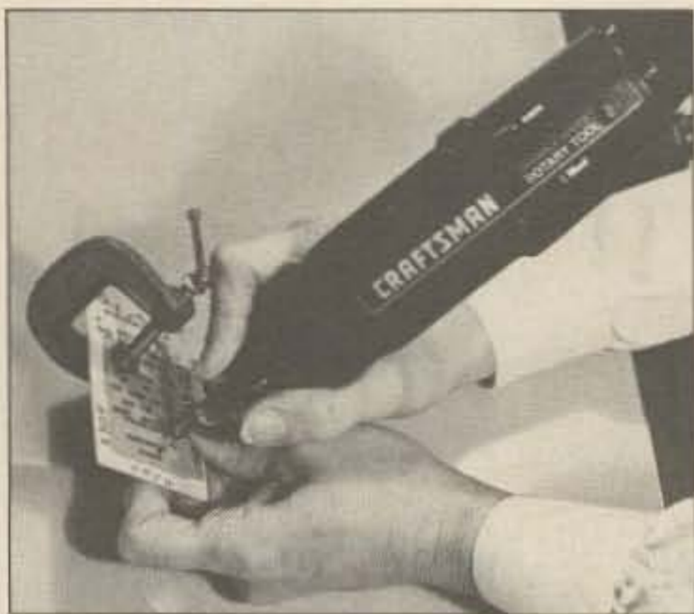
Photo D. Don't drill your finger! Place PC board with template on a suitable surface before drilling. The small drill bits are easy to break, so take your time.
