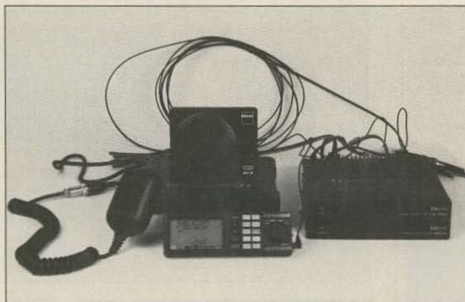
Photo A. The layout of the components of the IC-900 mobile rig. The band units (two black boxes at right) are stowed in an out-of-the-way place, such as the trunk. The interface (below speaker) goes inline between the control panel and the band units.
