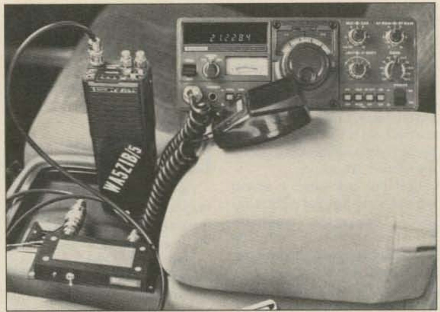
WA5ZIB's Mode-T mobile system. The Kenwood TS-130S provides between 50 and 100 Watts output on 15 meters. For reception, the Santec LS-202A HT is used with the Advanced Receiver Research GaAsFET preamp.
