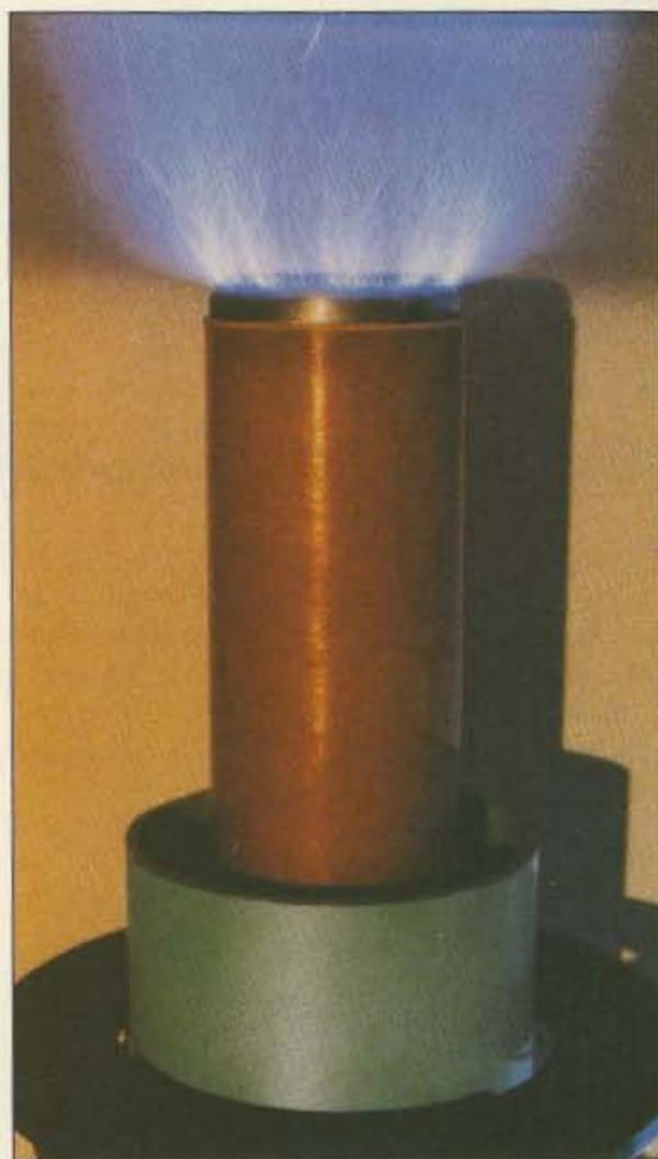
Photo A. Completed Tesla primary and secondary coils.
