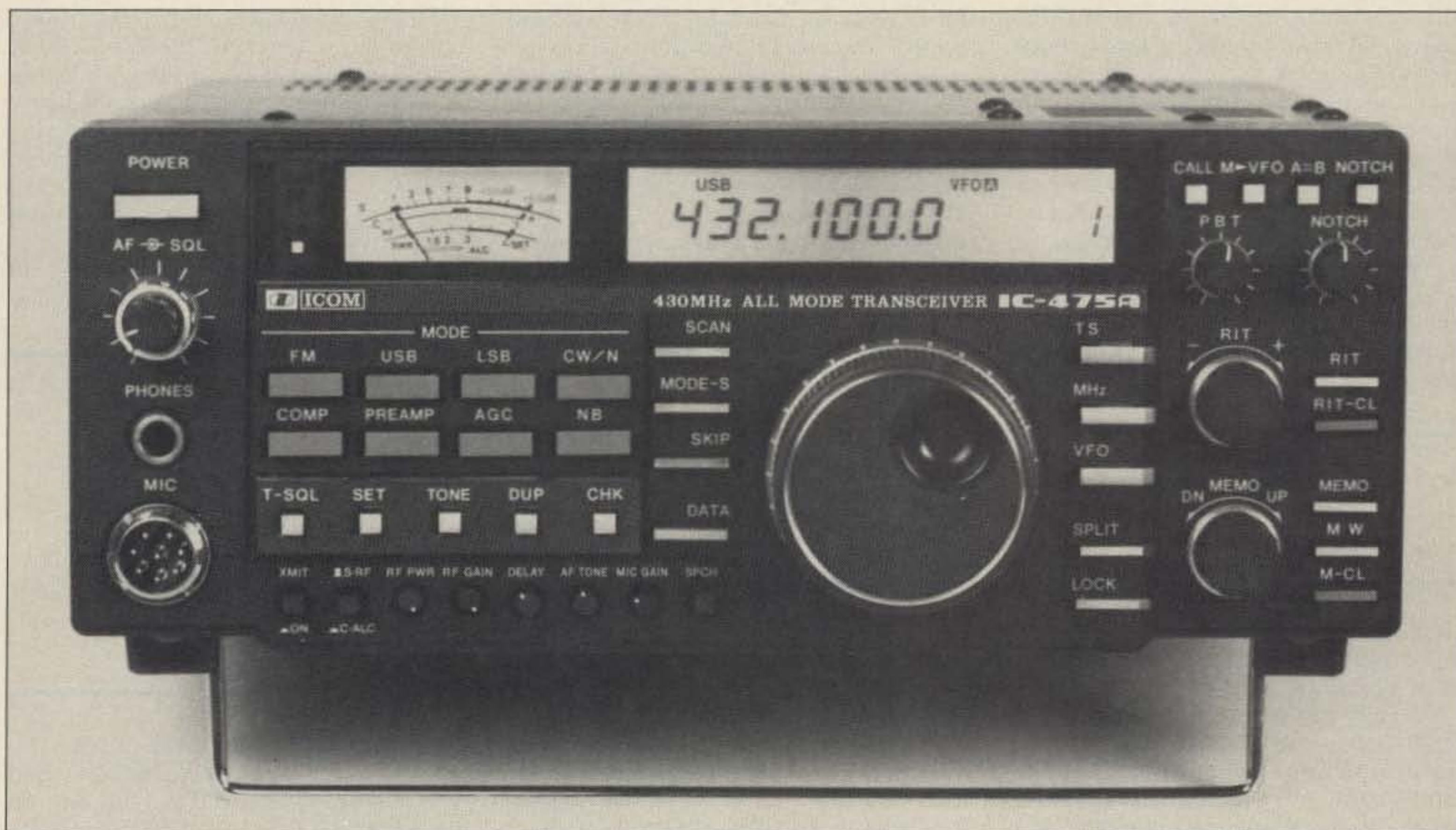
Photo A. Front view of the ICOM IC 475A, 70cm Multimode Transceiver.
