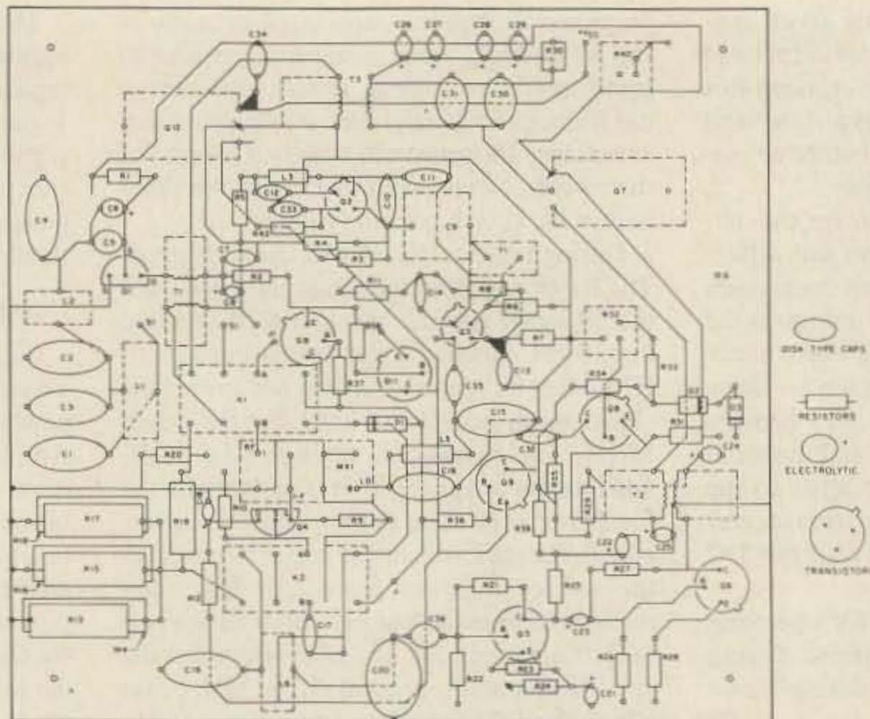
Figure 3. Parts placement for the transverter. A circuit board and parts kit are available. See text for details.
