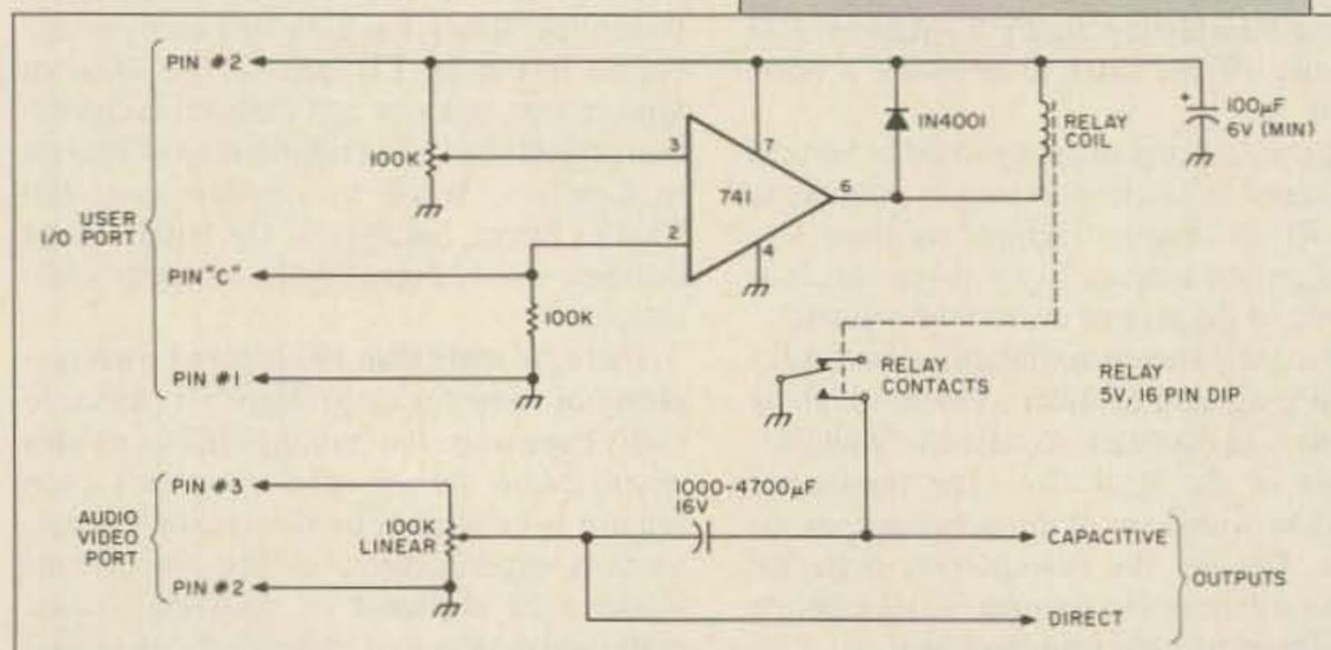
Fig. 2. Schematic for the audio/video port interface. Ludvigson does not supply this interface.
