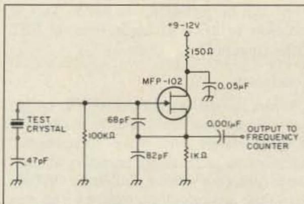
Fig. 2. Test oscillator for characterizing surplus crystals.
