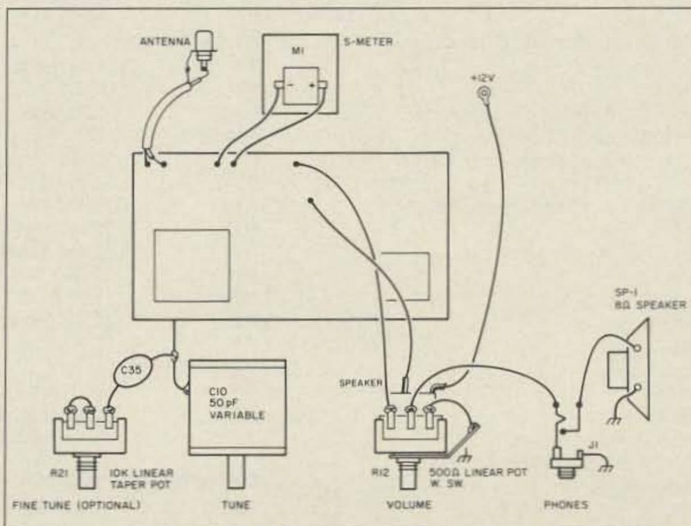
Fig. 4. Module connections.
