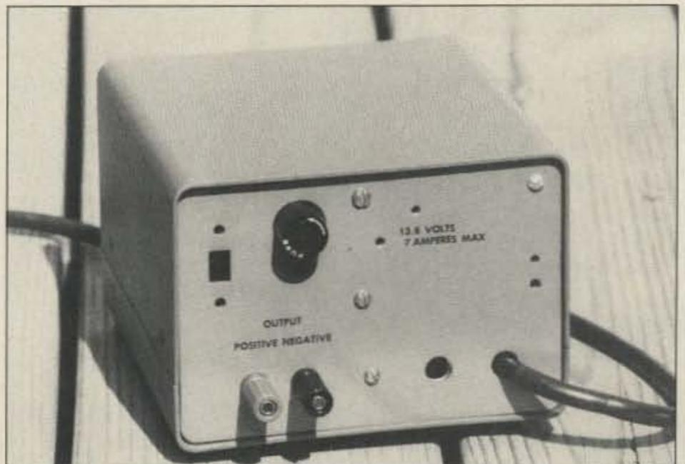
Photo D. Fuse in foreground is for the primary of the transformer.
