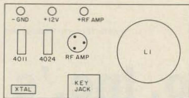
Figure 2. Layout of parts.
