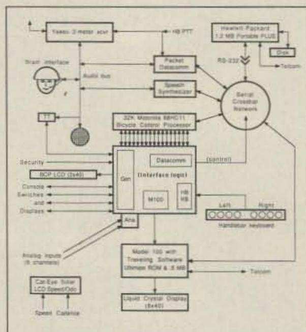
Fig. 1. The Winnebiko control system's internal architecture.
