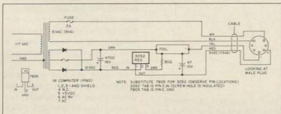
Figure 1. Power supply schematic for Commodore 64.
