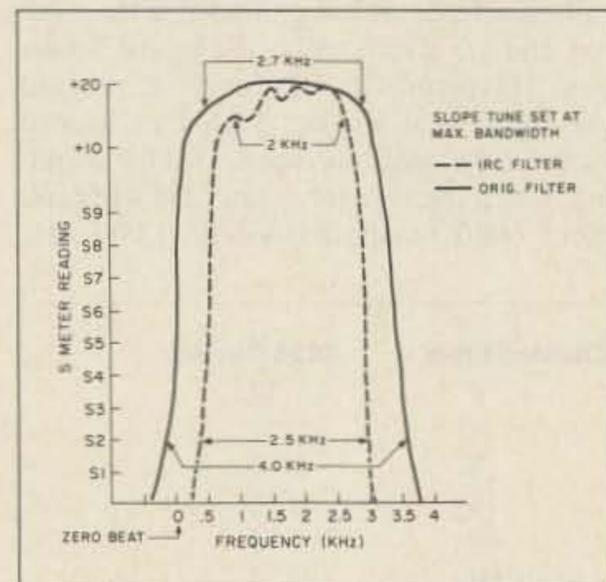
Figure 2. Slope tune, set at maximum bandwidth.
