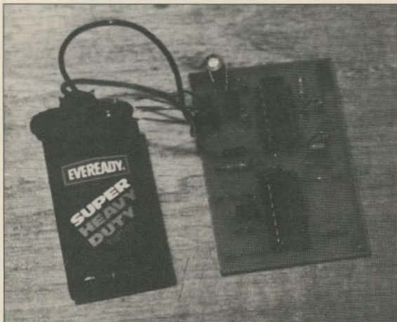
Photo A. Not much larger than the 9 volt battery that operates the circuit, the QRP CMOS keyer.
