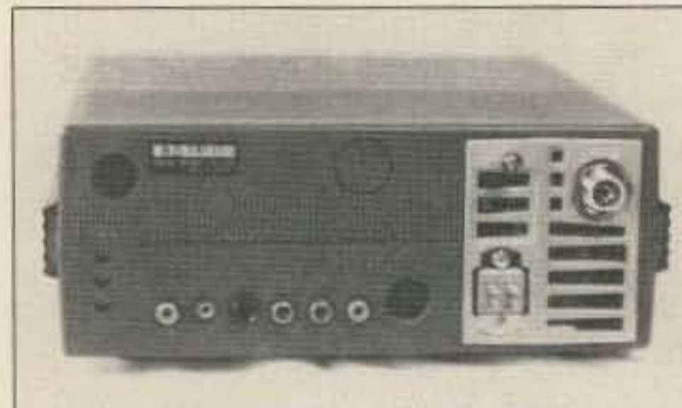
Photo B. The rear panel showing the part of the cast aluminum transmitter chassis.
