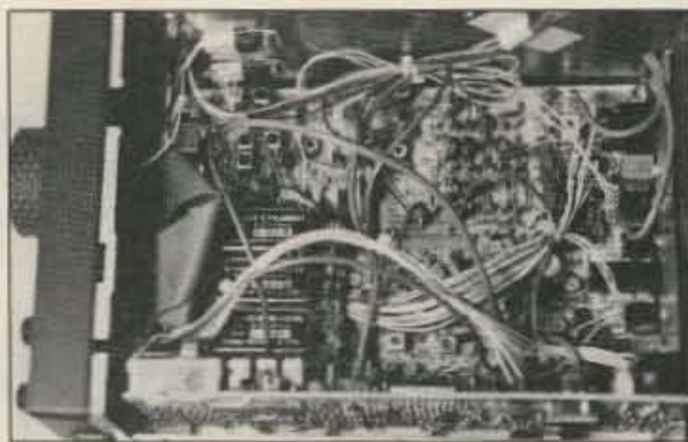
Photo C. Notice the factory installed (standard) crystal filters.
