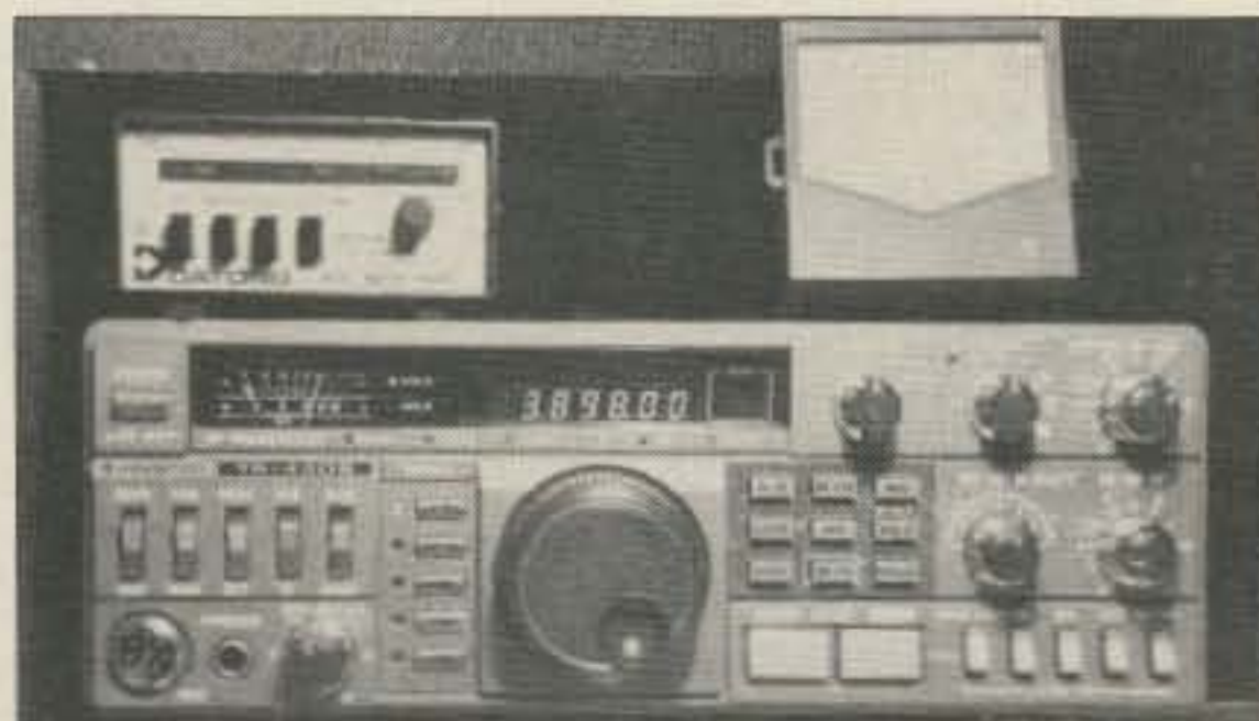
Photo B. Notice the 10 segment LED bar graph at the top of the ANF for displaying search and lock action.
