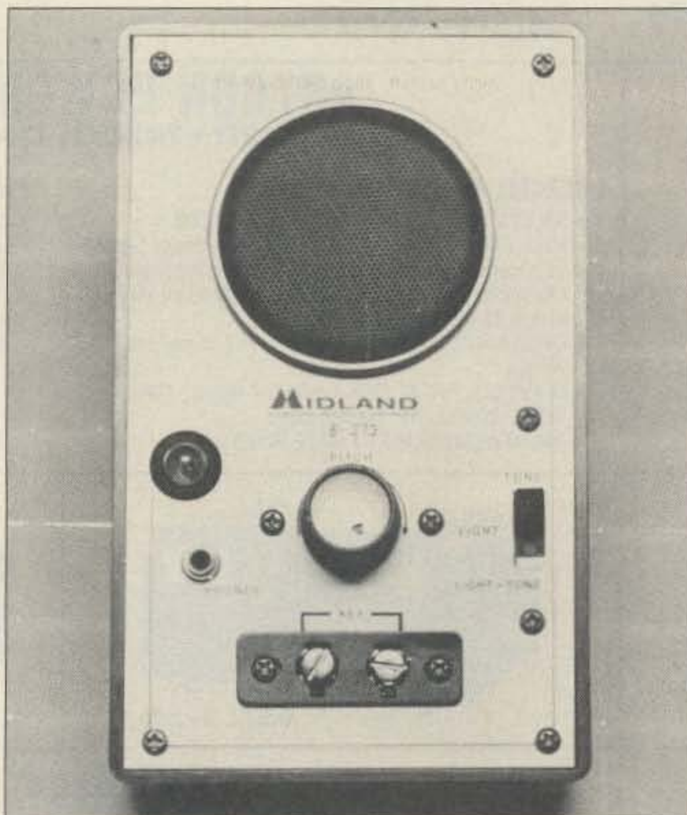
Photo C. Here's an oscillator with a built-in light. "Seeing" the code helps some students.
