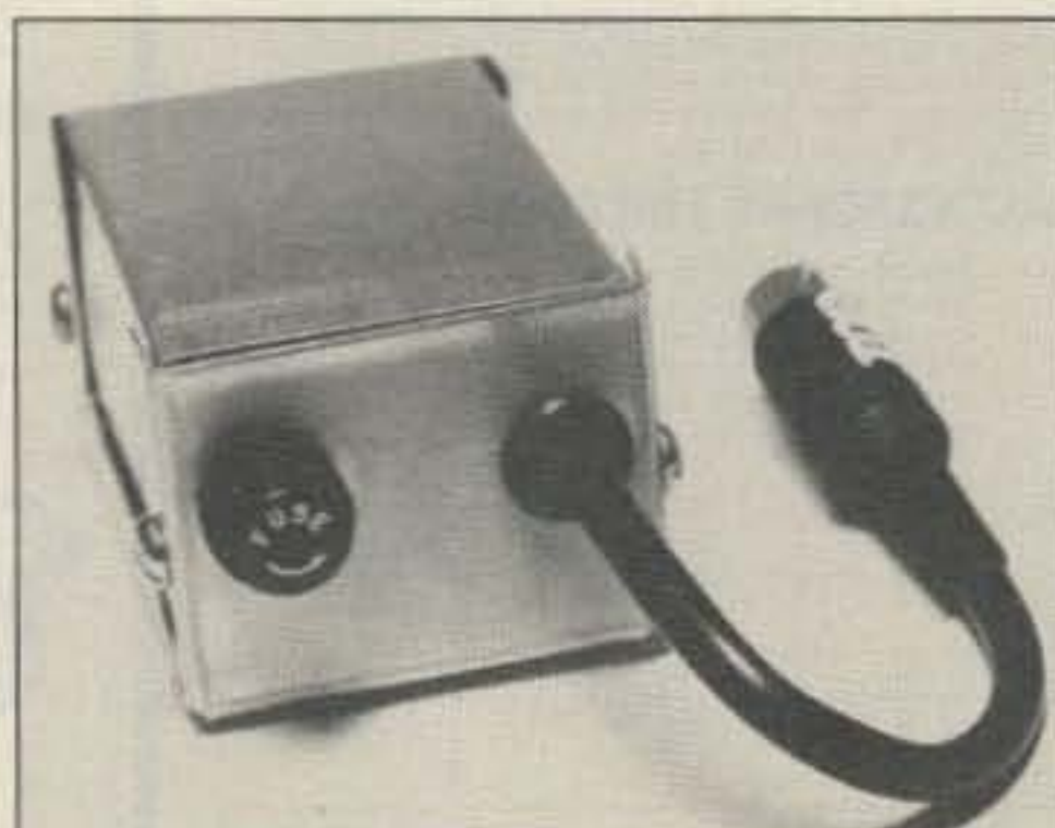
Photo A. The completed Commodore 64 Voltage Protector.
