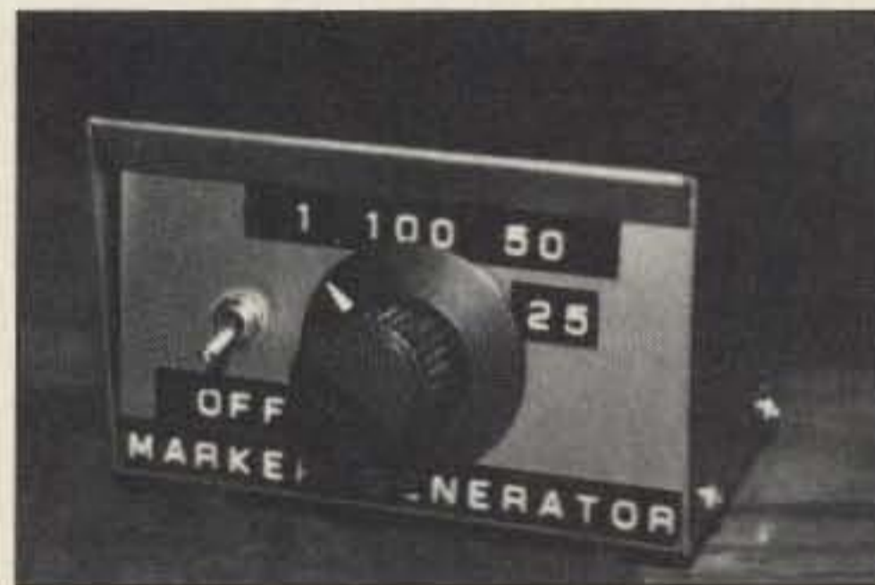
Photo A. The finished project. The entire unit is housed in a chassis box purchased at a local flea market.
