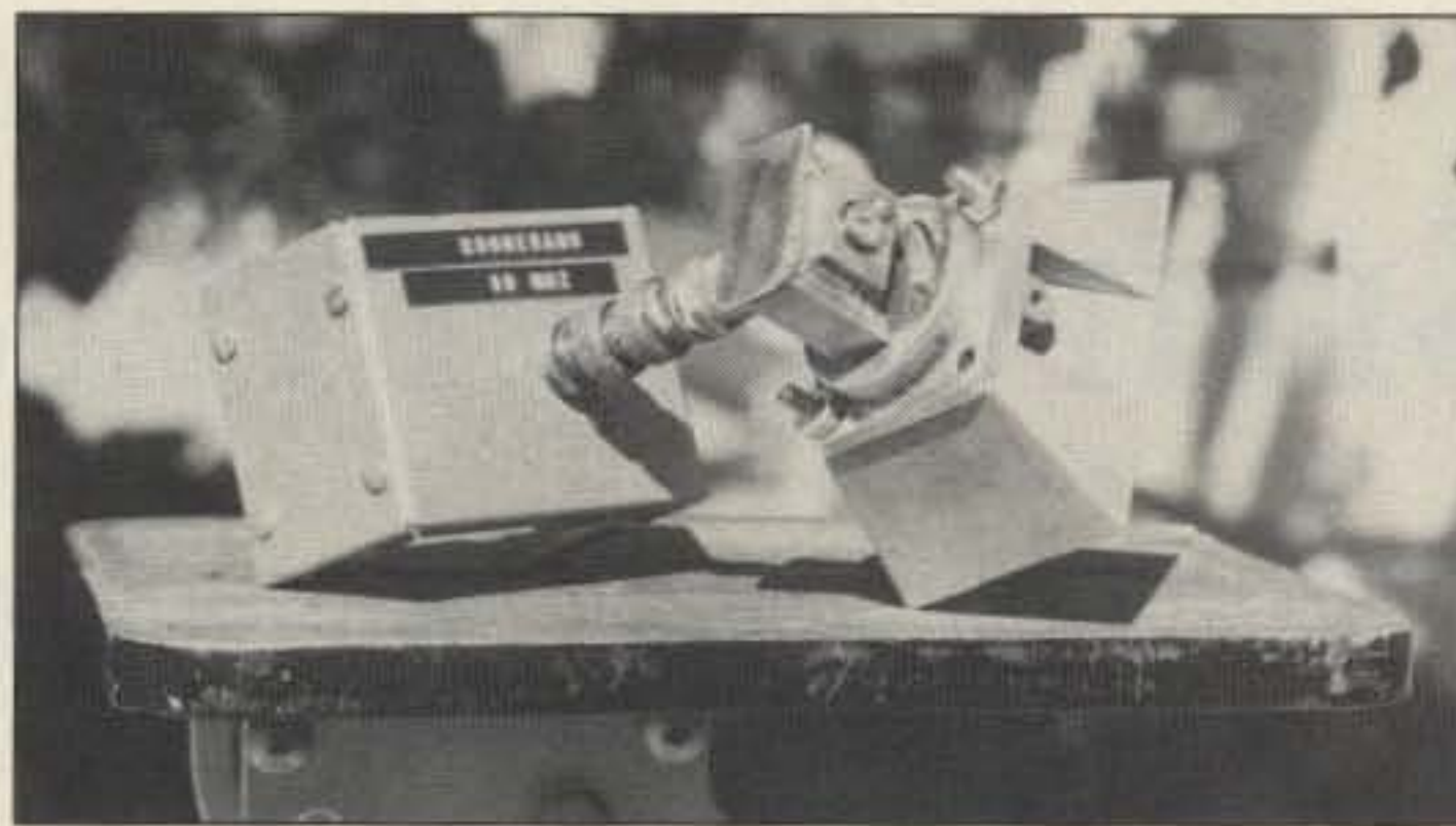
Photo D. Rear view of Boomerang showing back construction used on home-brew detector mount.
