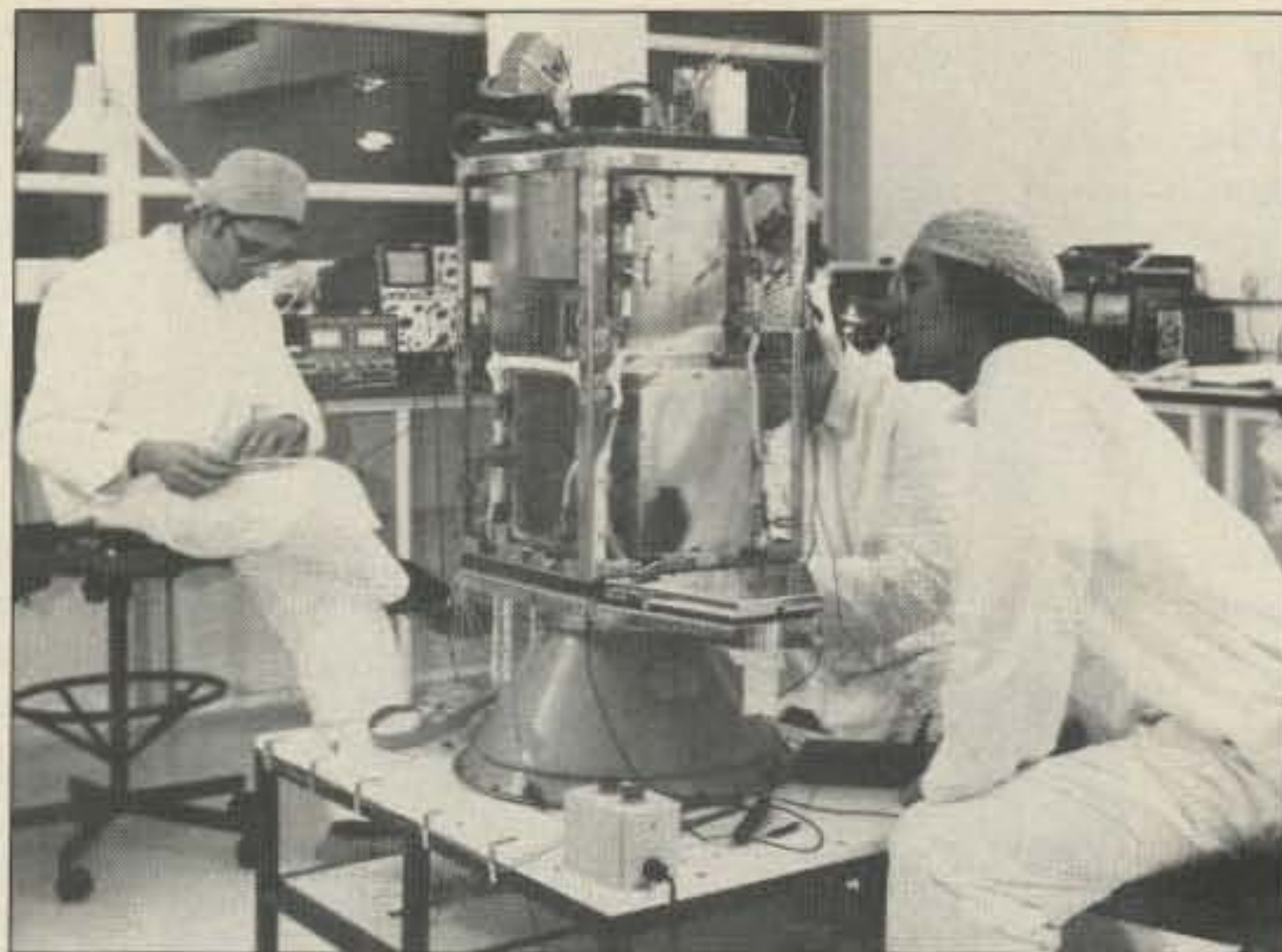
Photo B. Mike Blewett G4VRN (left) and Richard MacBeth G8VLY examine UoSAT-OSCAR-11 in the University of Surrey clean room. The solar panels are removed to permit access to modules and the wiring harness. Photo by Martin Sweeting G3YJO.
