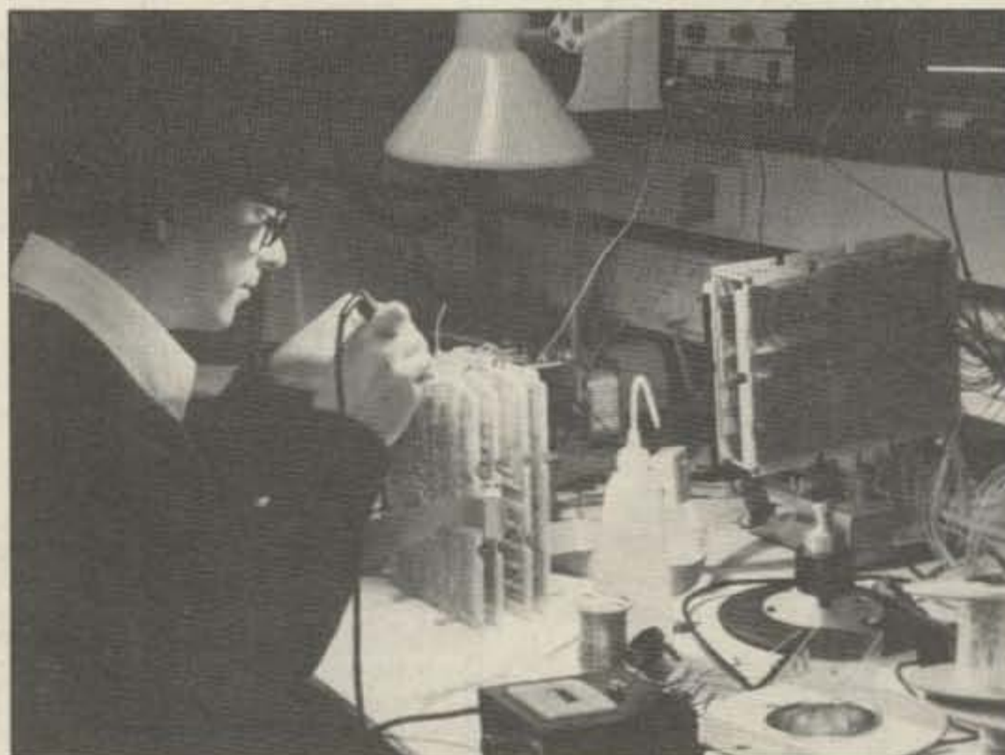
Photo A. Roger Peel G8NEF working on an engineering model of the UoSAT-OSCAR-11 on-board computer. Photo by Martin Sweeting G3YJO.
