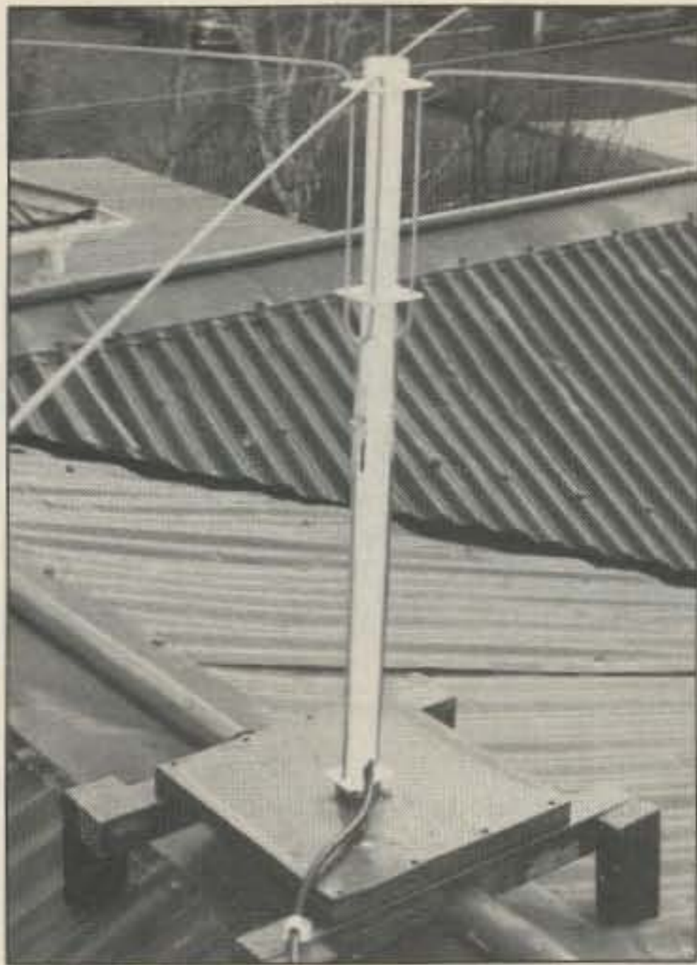
Photo B. The collinear sections are made from single lengths of 1/4-inch brass tubing. The coax-feedline comes up through the PVC mast. It is matched to the turnstile by a 1/2-wave section joining the two collinears. The roof is the reflector.
