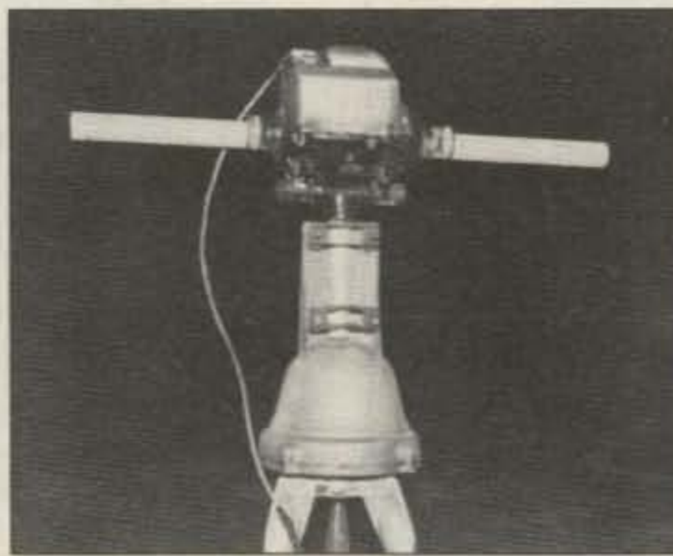
Photo D. Elements of an Az-El. In this system, the modified El rotor is united with a flea market CDR rotor with short sections of 1" od threaded water pipe components. The horizontal mast is typically about 38" long.
