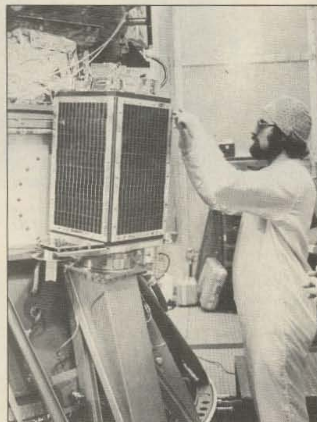
Photo E. Inside the launcher gantry at Vandenberg AFB, California, Ian Ferebee G6BTU places the solar panel on UoSAT-OSCAR-11. The satellite is in its final position, just below the main payload. Photo by Martin Sweeting G3YJO.
