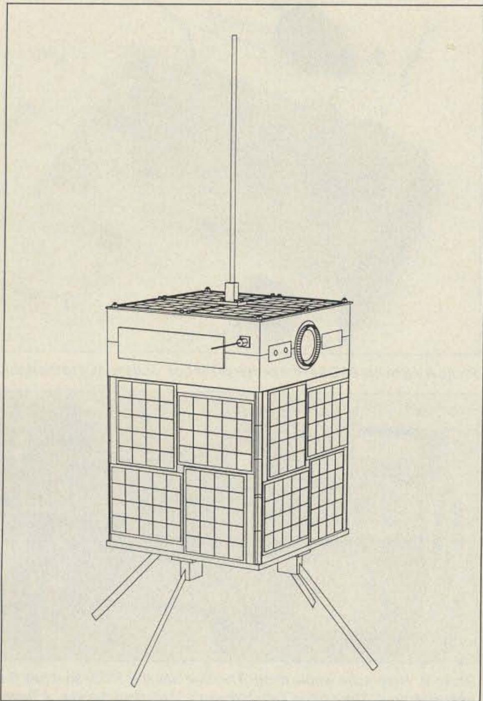
Photo C. Drawing of WEBERSAT by Dick Jansson WB4FAB, AMSAT-NA. Note camera lens on the side of the top module.
