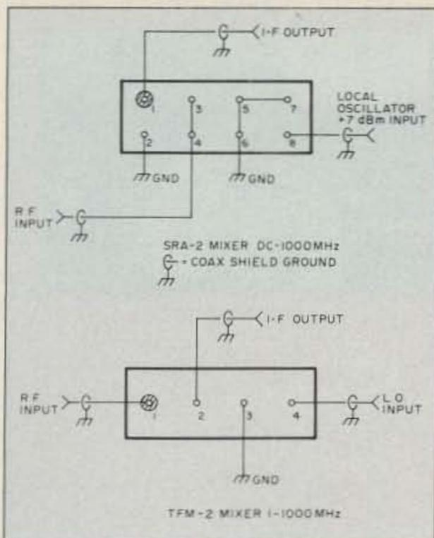
Figure 2. Typical mixer connections.
