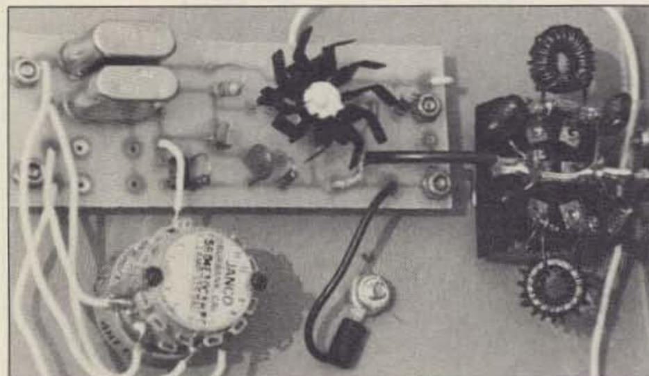
Photo B. Here's the whole thing. This one has the 3553, so it has the heat sink on it. The crystal switch doesn't come with the kits. A better band switch is now provided.
