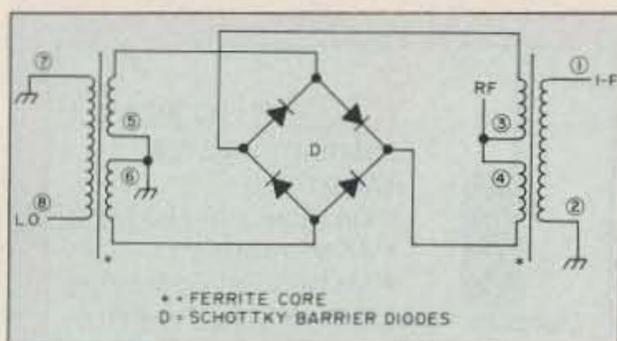
Figure 3. Schematic for basic mixer.
