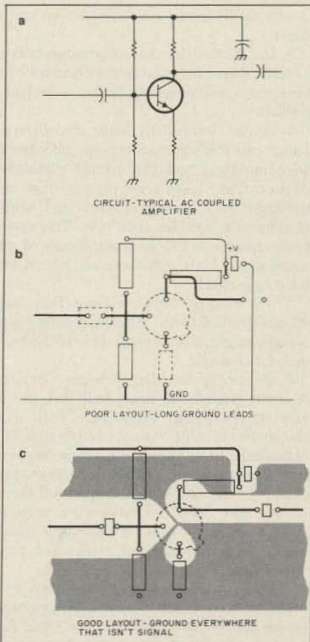
Figure 1. (a) Typical AC coupled amplifier circuit. (b) Poor layout. Notice the long ground leads. (c) Layout with lots of ground. Ground is everywhere except for signal leads.
