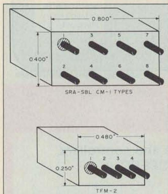
Figure 1. Dimensions and pinouts of common mixer modules.
