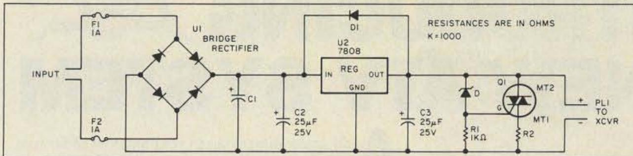
Schematic of the UNI-8 power converter.
