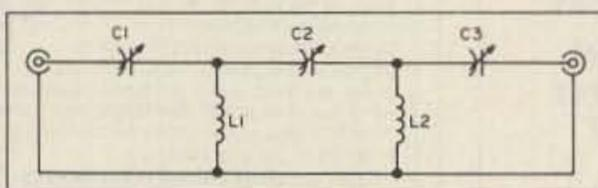
This filter goes between the transceiver and the antenna. Of course, if the CB guy is running three kW, sterner measures may be required.
