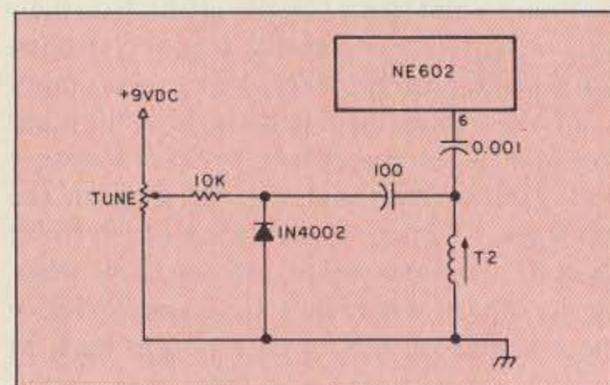
Figure 1. The original HR-4 tuning circuit.
