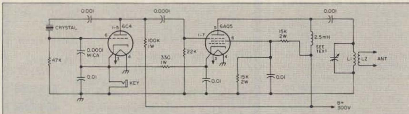
Figure. A 6C4 is used in a Pierce oscillator driving a 6AQ5 as an amplifier or doubler.
