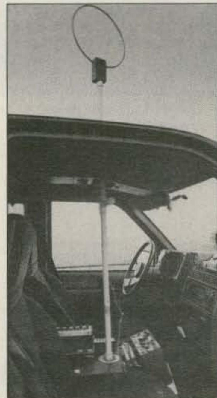
Photo A. The HF Homer system installed in the van, ready for hunting with a TS-130 transceiver and RF attenuator on the home-built center console. Coax and relay wires go inside the mast to the top of the tee-handle, then break out.
