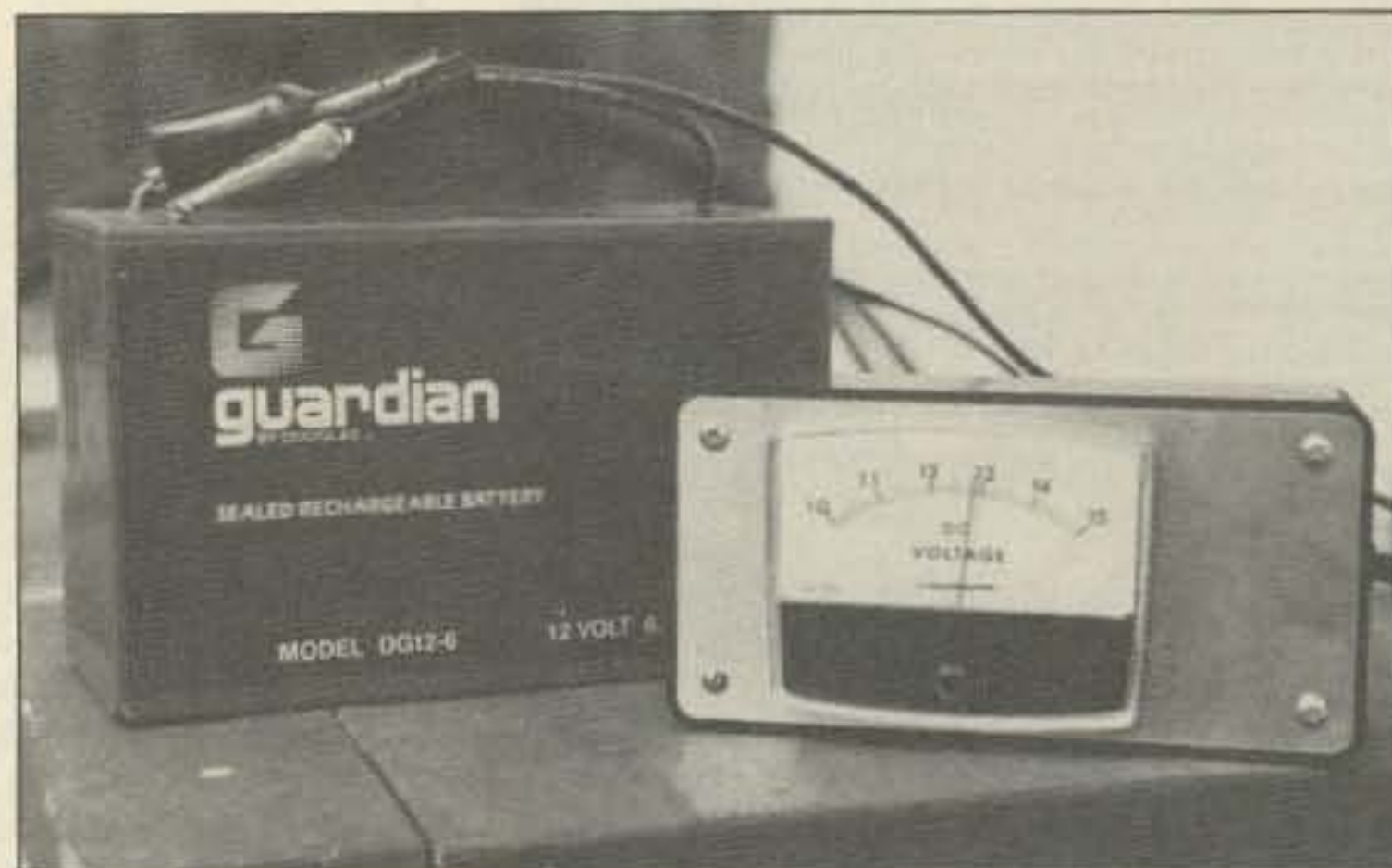
Photo A. The completed, expanded voltmeter keeps an eye on the battery.
