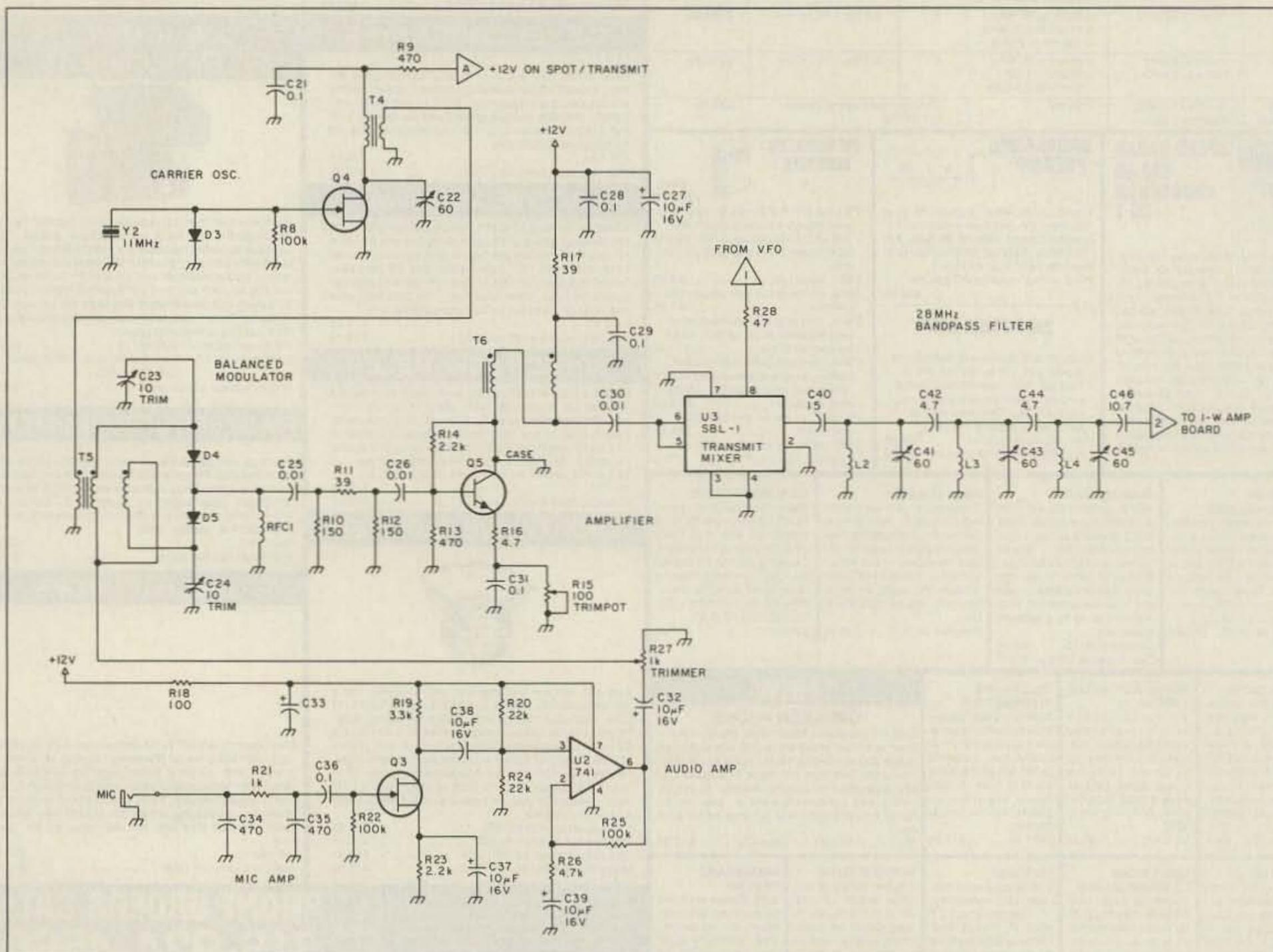
Figure 3. The balanced modulator/mixer board.
