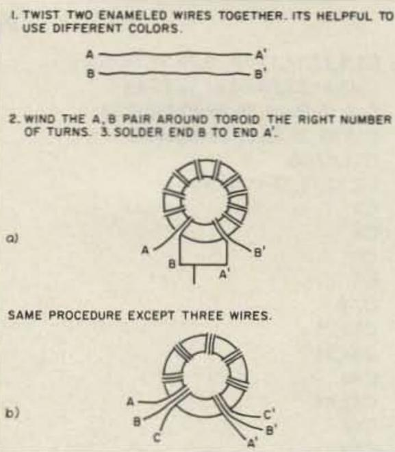
Figure 9. Winding the (a) bifilar transformer, and the (b) trifilar transformer.
