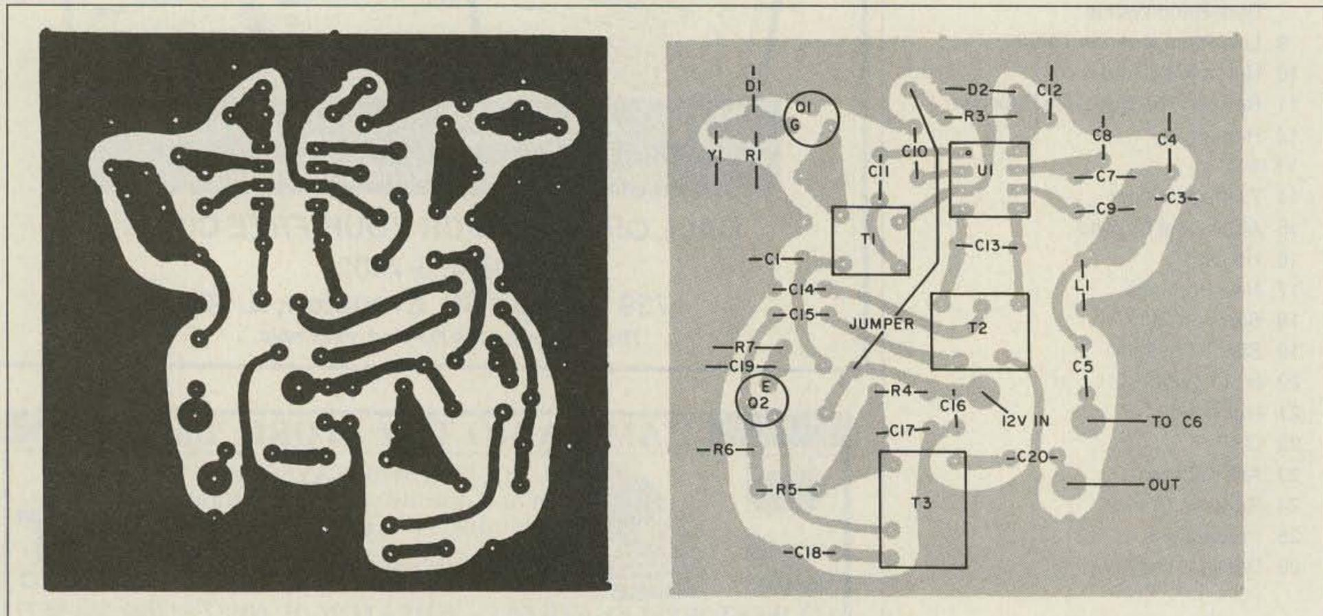
Figure 5 (a) The VFO foil pattern. (b) Parts placement.
