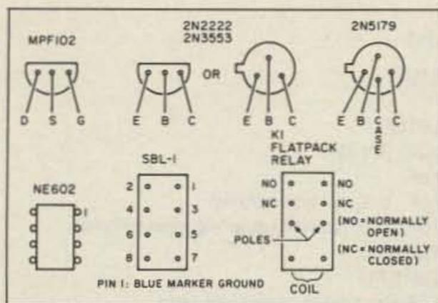
Figure 8. Base diagrams, all bottom view.
