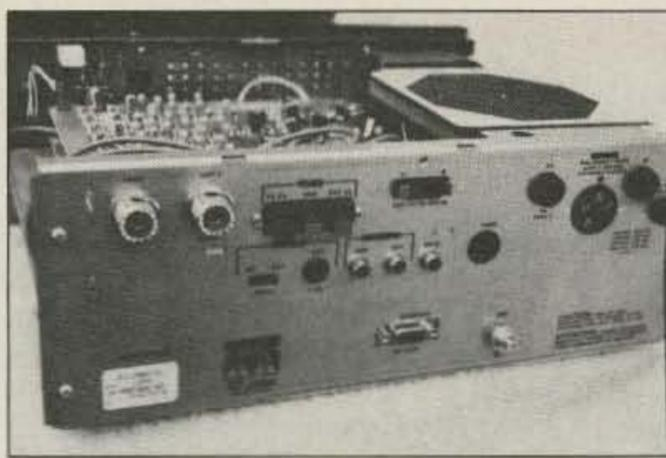
Photo B. The R8 can be connected to various antennas as well as to a computer through the RS-232 port.
