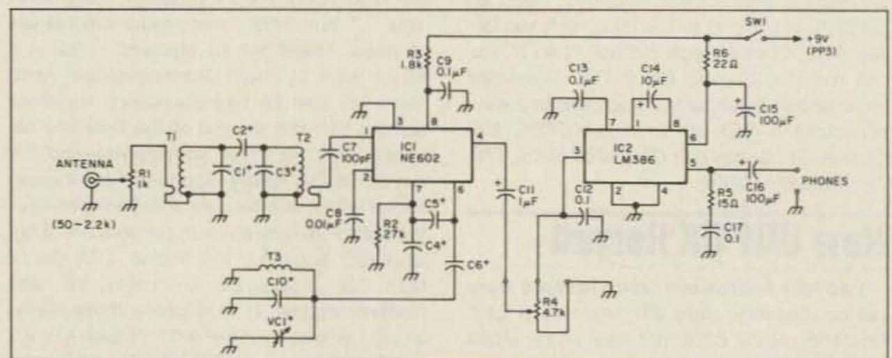
Figure 2. Schematic of the Sudden Receiver circuit.
