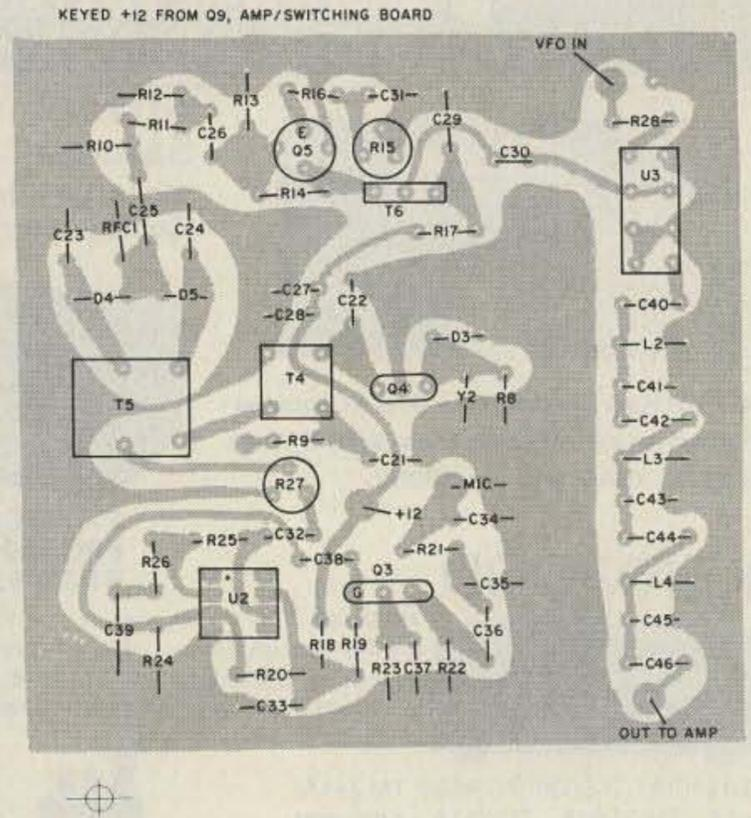
Figure 6 (a) The balanced modulator/mixer foil pattern.
