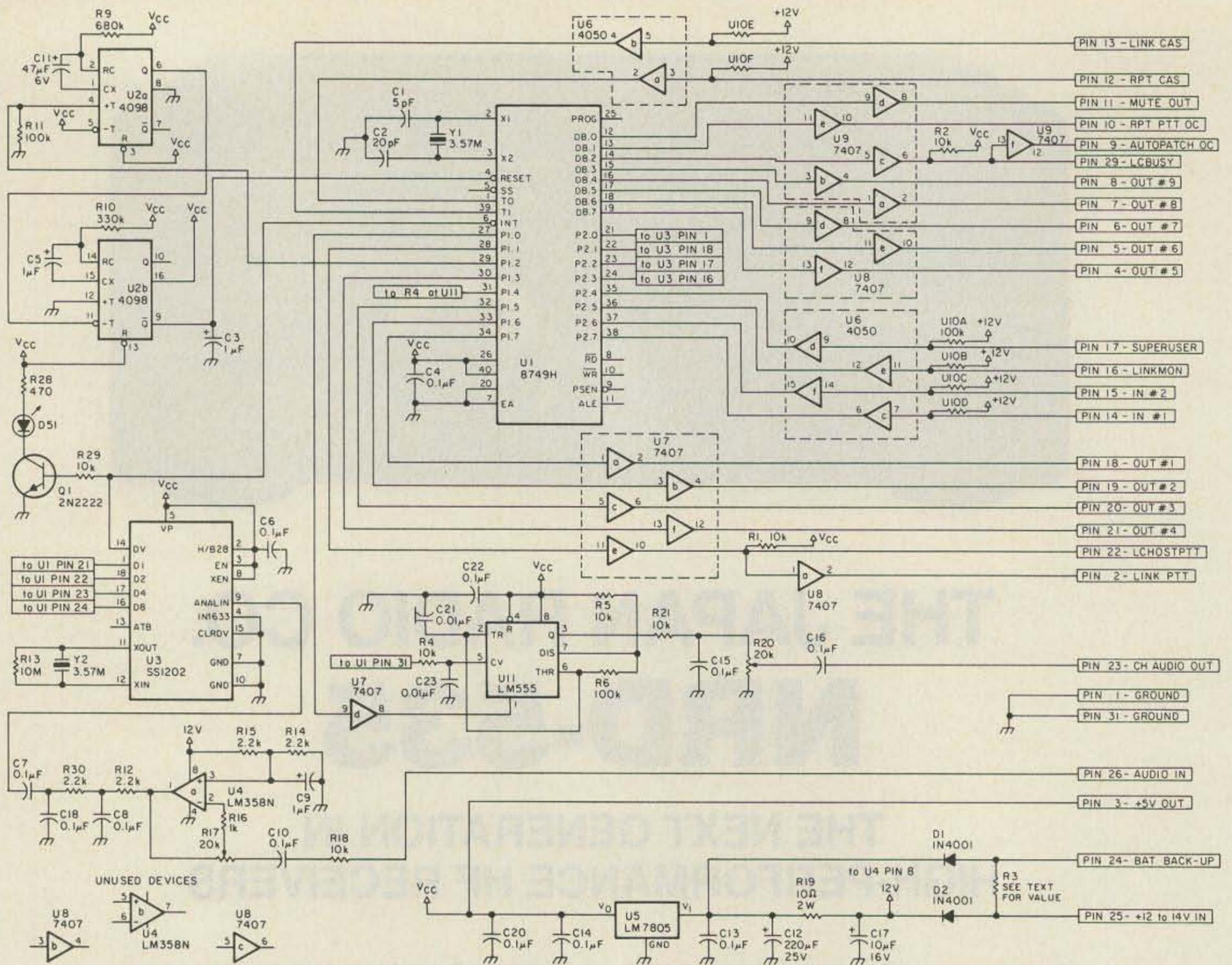
Figure 2. Schematic for the repeater controller computer board.
