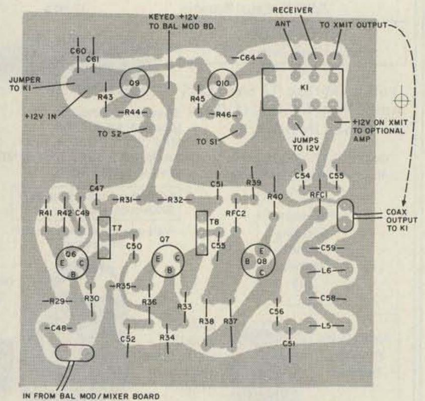
Figure 7 (a) The 1 watt amplifier/switching board.
