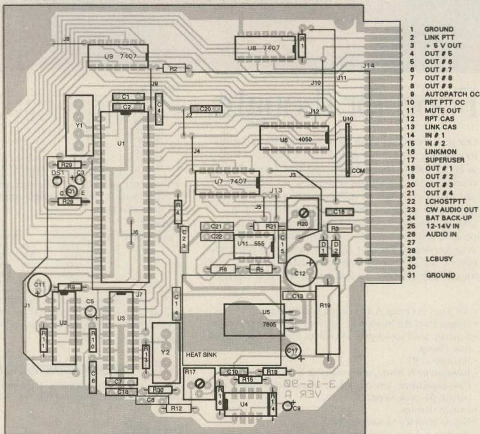
Figure 4. Computer board parts placement.
