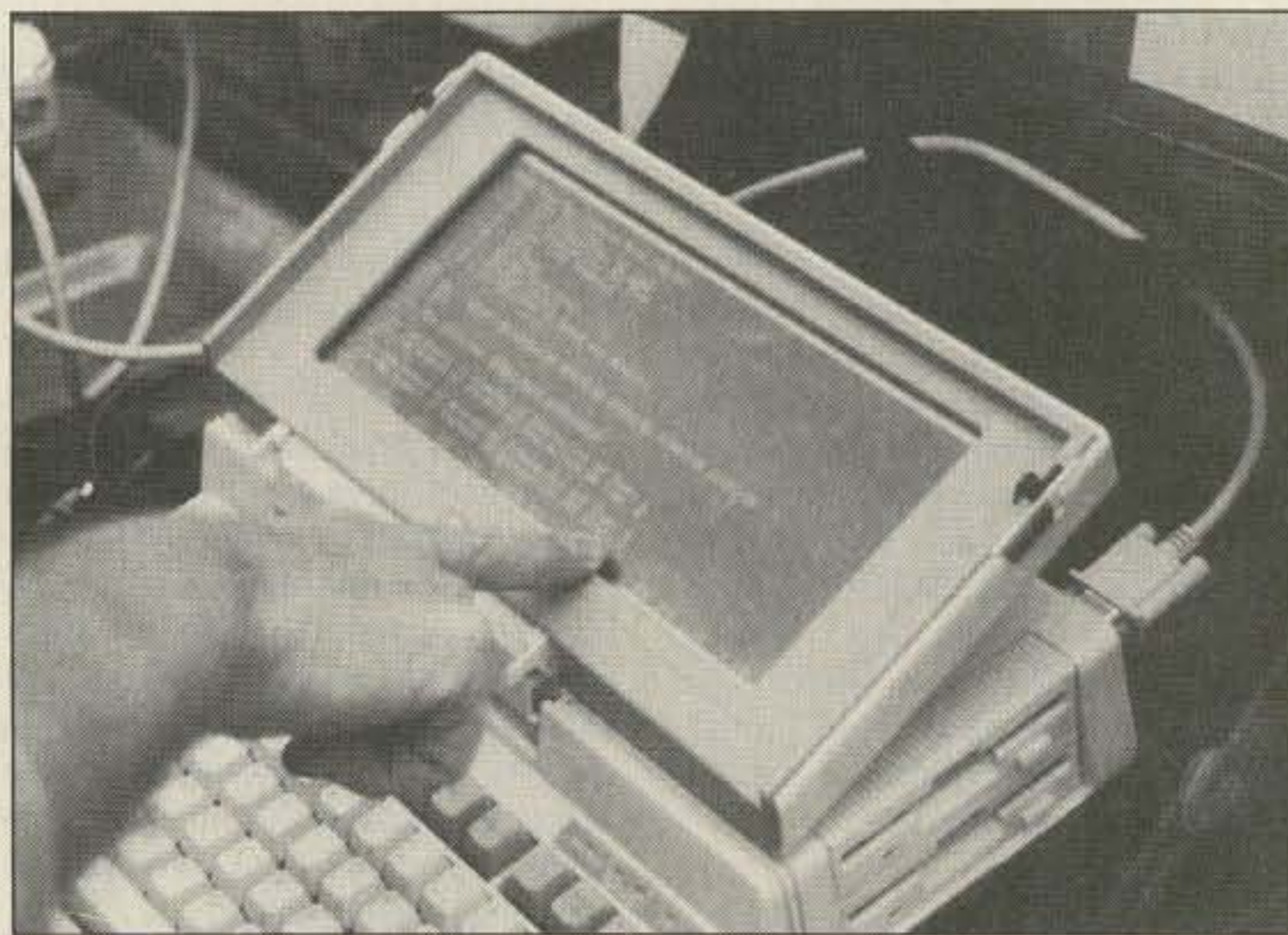
Photo A. TBOX parameters can be changed in the field with a laptop computer operating in the "dumb terminal" mode. The firmware is menu-driven.
