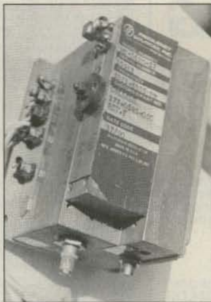
Photo A. The Frequency West 6 GHz PLL brick. It's mechanically similar to the 10 GHz brick. Remove the blue label on top to access the filter adjust screws.
