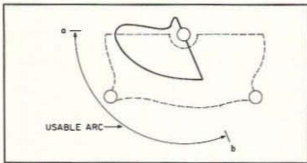
Figure 1. Capacitor rotor shape.
