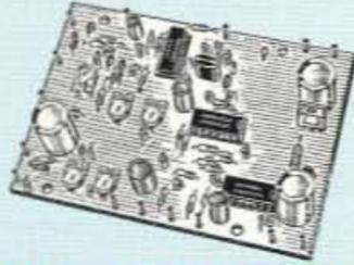
**COR-3 REPEATER CONTROLLER.** Features adjustable tail and time-out timers, solid-state relay, courtesy beep, and local speaker amplifier .....kit \$49
