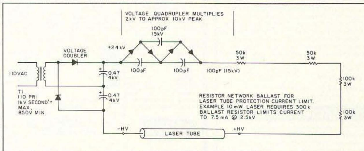
Figure 1. Laser power supply starting circuit.
