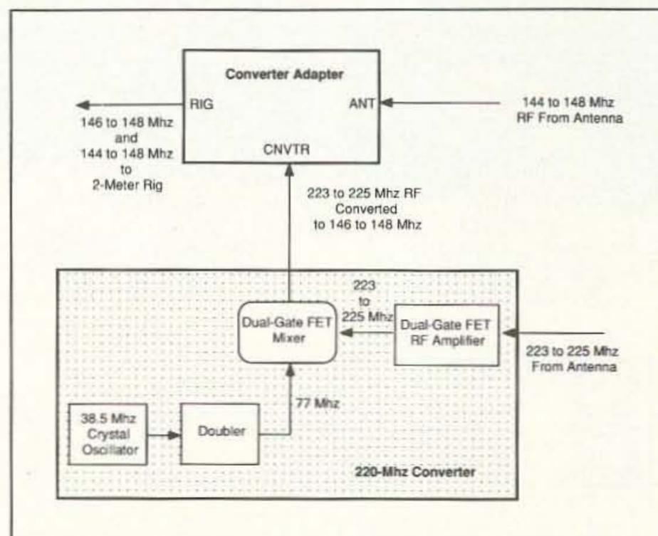
Figure 5. Converter circuit for 220 MHz operation.
