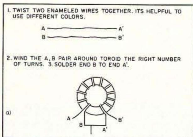
Figure 4. Bifilar winding details for toroid T2.
