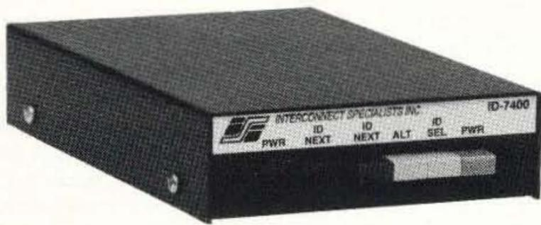
The ID-7400 is an automatic voice identifier for use on any transceiver or repeater. The ID-7400 records your voice ID, then automatically transmits it at the proper time, on the release of your PTT switch. Two switch selectable IDs can be recorded and stored in non volatile electronic memory. Records from the station microphone. Installs between the microphone and the transceiver. No soldering required. Uses 8 pin mic connectors.
