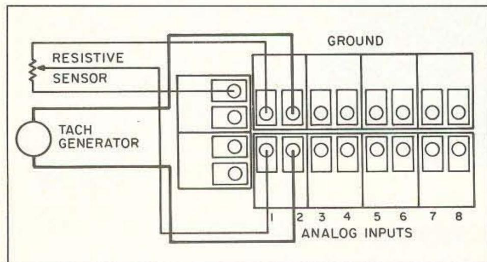
Figure 2. Typical connections for a variety of transducers.
