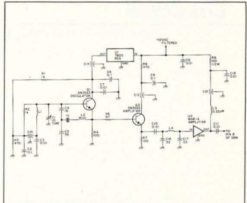
Figure 7. Schematic diagram of the local oscillator.
