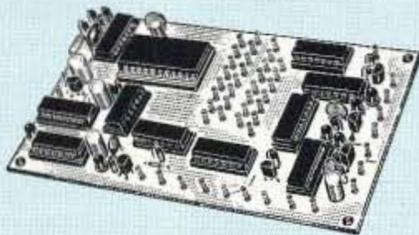
**TD-2 TOUCH-TONE DECODER/CONTROLLER kit.** Full 16 digits, with toll-call restrictor, programmable. Can turn 5 functions on/off. Great for selective calling, too! .....kit \$89, wired/tested \$149
