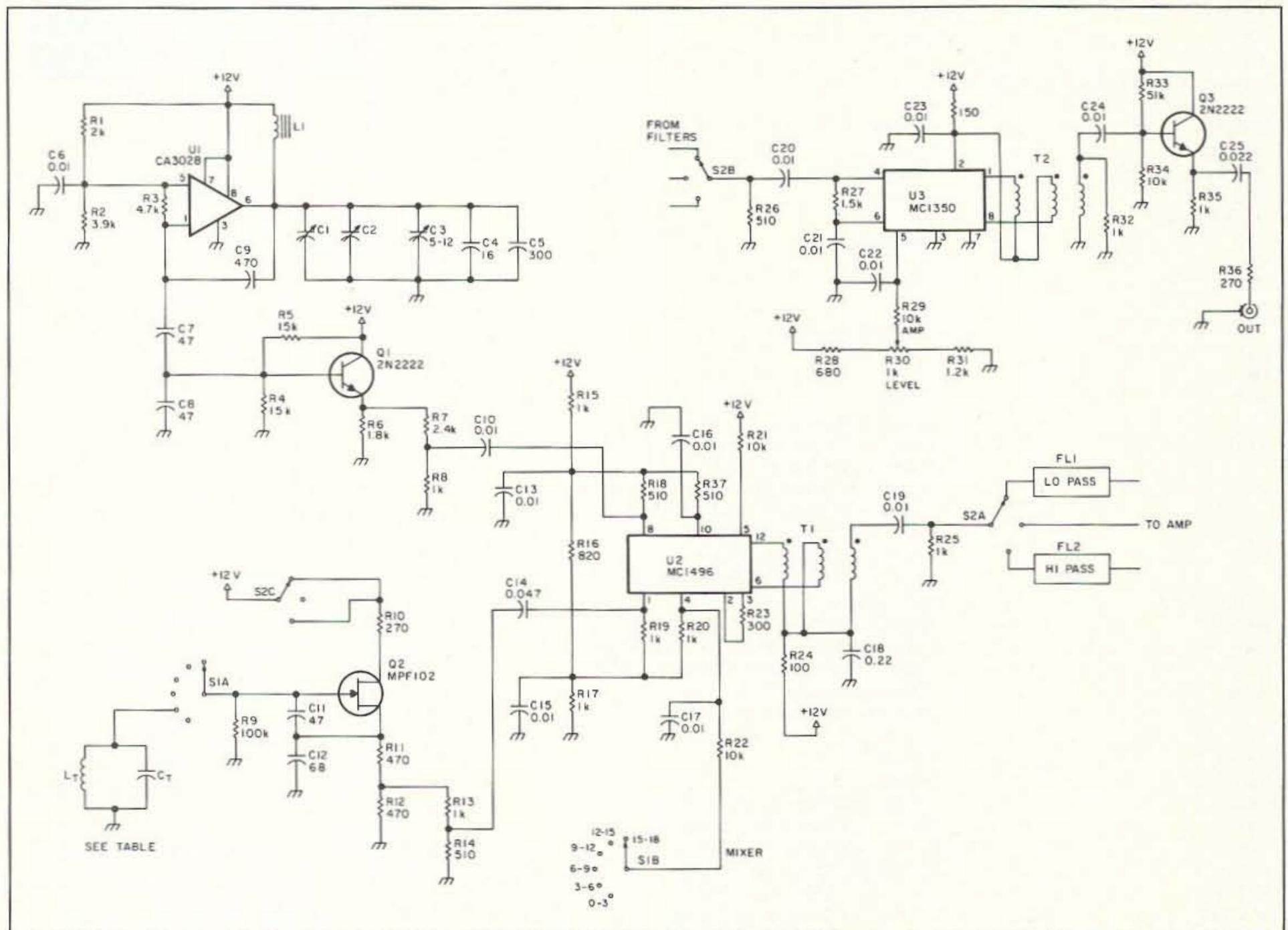
Figure 7. Overall schematic of signal generator.
