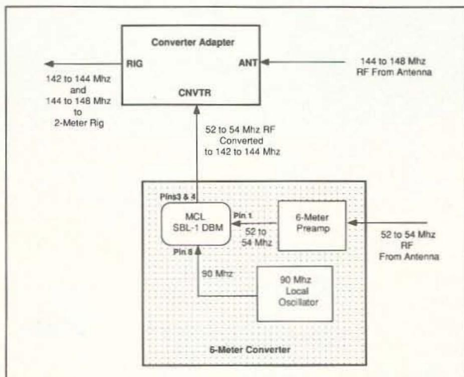
Figure 4. Six meter converter for the Converter Adapter.
