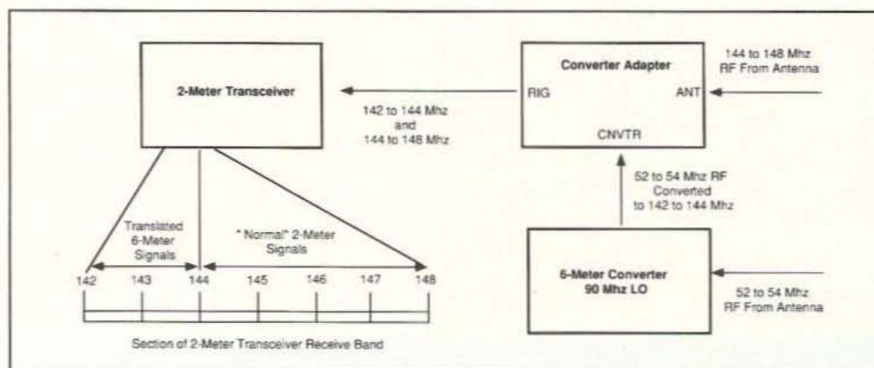
Figure 1. Block diagram of the Receive Converter Adapter.
