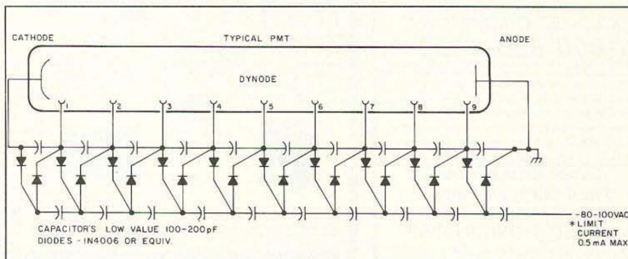
Figure 2. New PMT power supply drive circuit.
