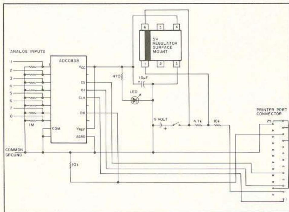
Figure 1. Schematic diagram of the A-to-D converter.
