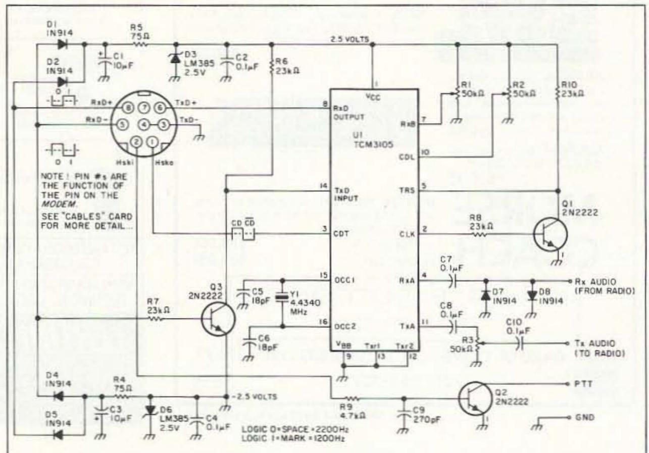
Figure 1. Schematic diagram of the PacketMac Modem.
