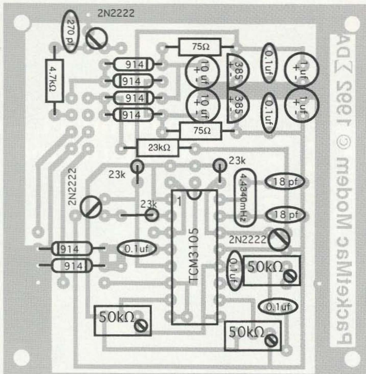
Figure 3. Parts placement.
