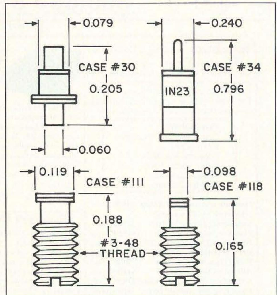
Figure 4. Various case styles for microwave diodes, detectors, and Gunn devices. All dimensions are in fractional inches.
