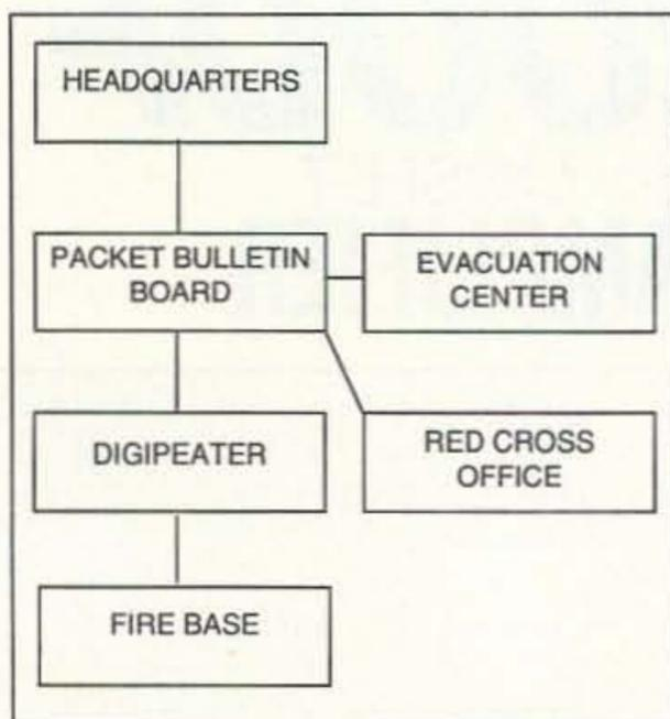
Figure 1. Typical packet radio network block diagram.
