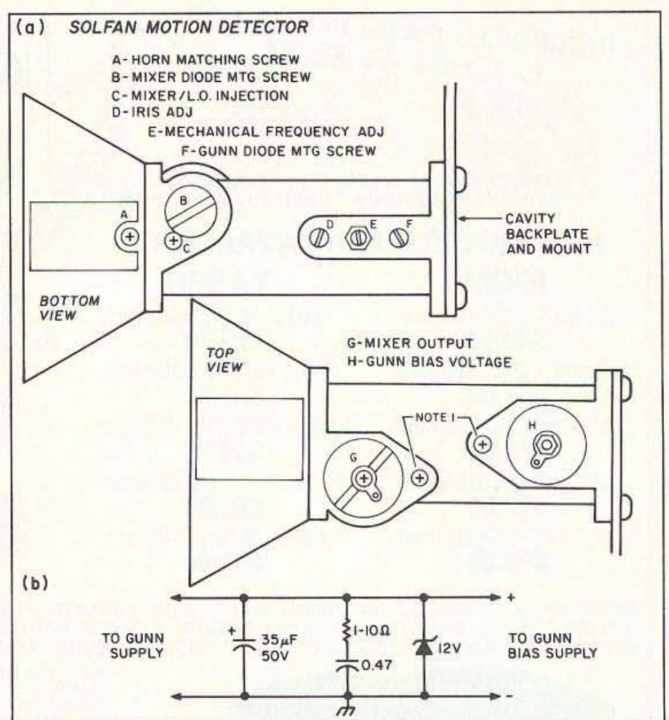
Figure 3. Typical Solfan cavity design adjustment/DC feed locations. a) Note 1: There is a cluster of parts attached to these two screws, one of which is a ground lug and the other insulated. See text. Note 2: All adjustment and mounting screws use a liquid lockwasher compound. Use moderate heat and/or suitable solvents to clean these. Use caution when removing so as not to break off these screws. b) Recommended Gunn protect network (see text).
