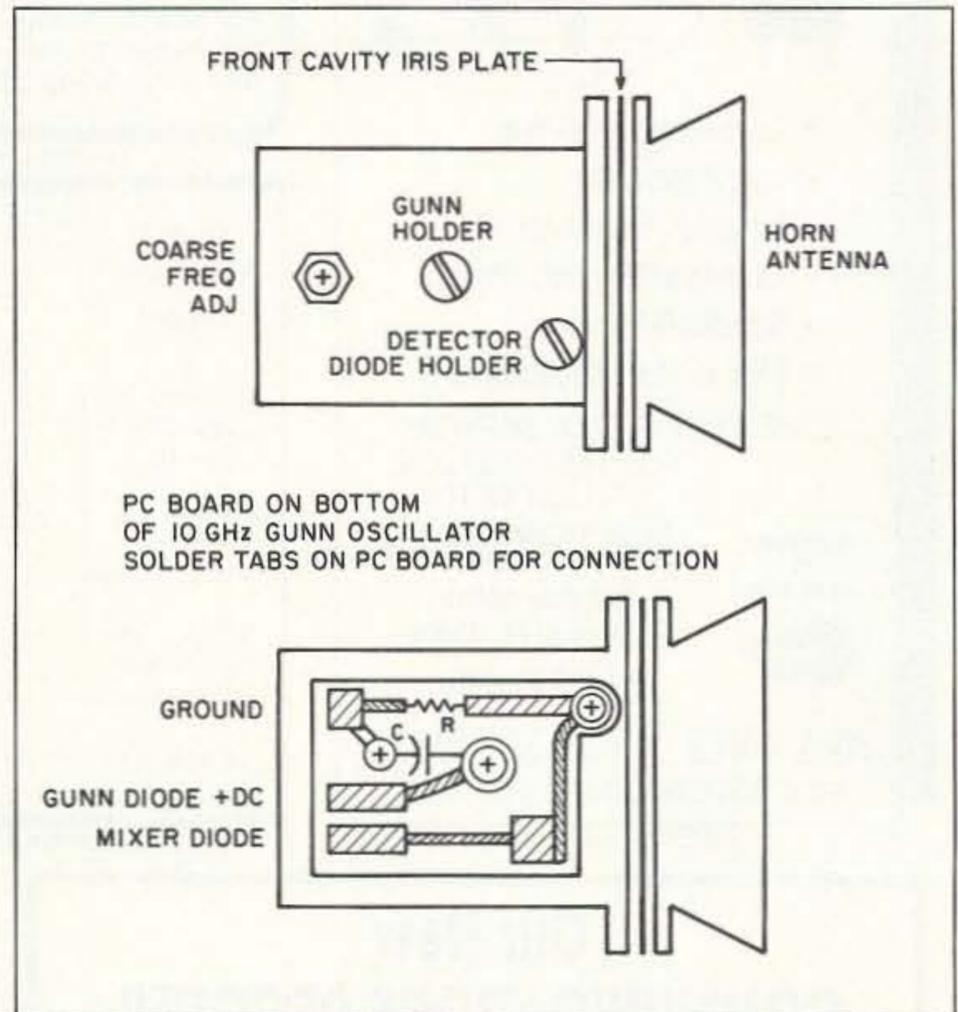
Figure 2. Drawing of the EMCOR Industries cavity (see text).
