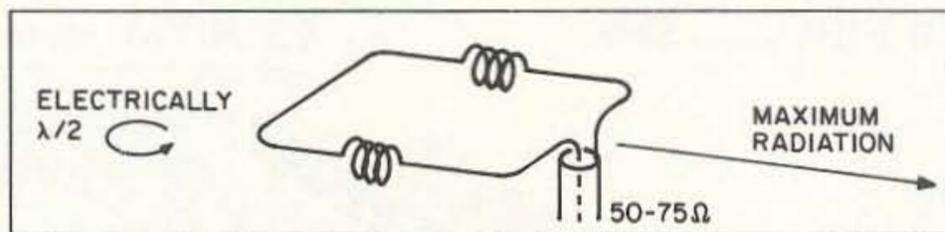
Figure 1. Diagram of the baby loop antenna.
