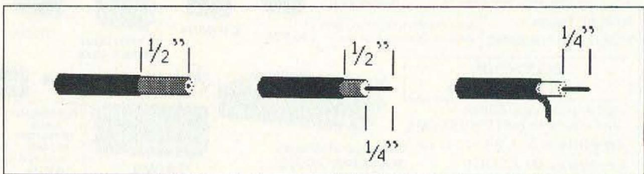
Figure 3. Preparation of the coaxial cables.
