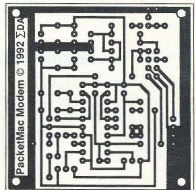
Figure 2. PC board foil pattern for the PacketMac Modem.
