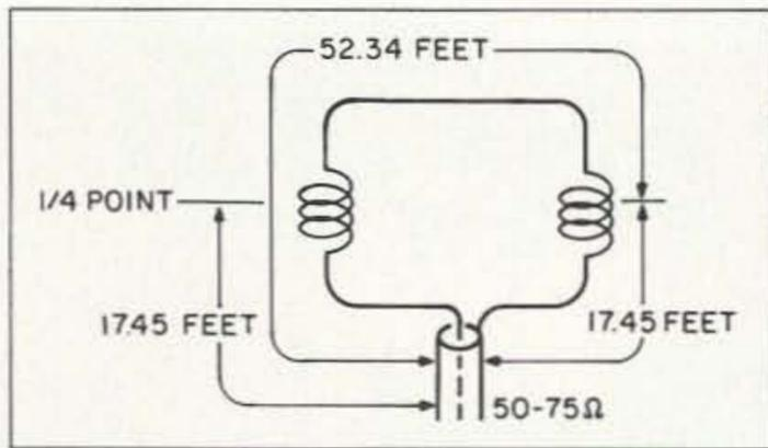
Figure 2. Dimensions of the 40m version.
