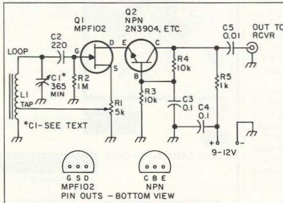
Figure 1. Preamplifier circuit.
