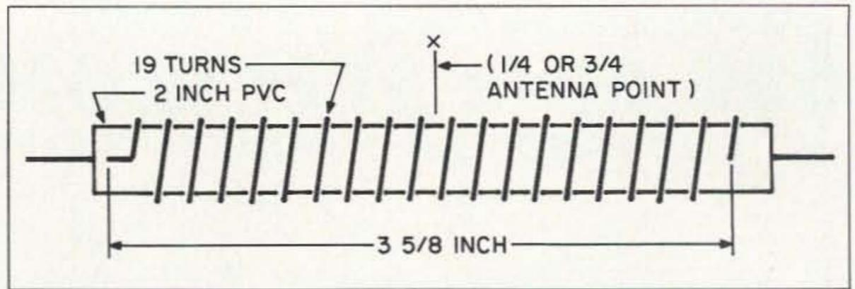
Figure 3. Coil winding details.
