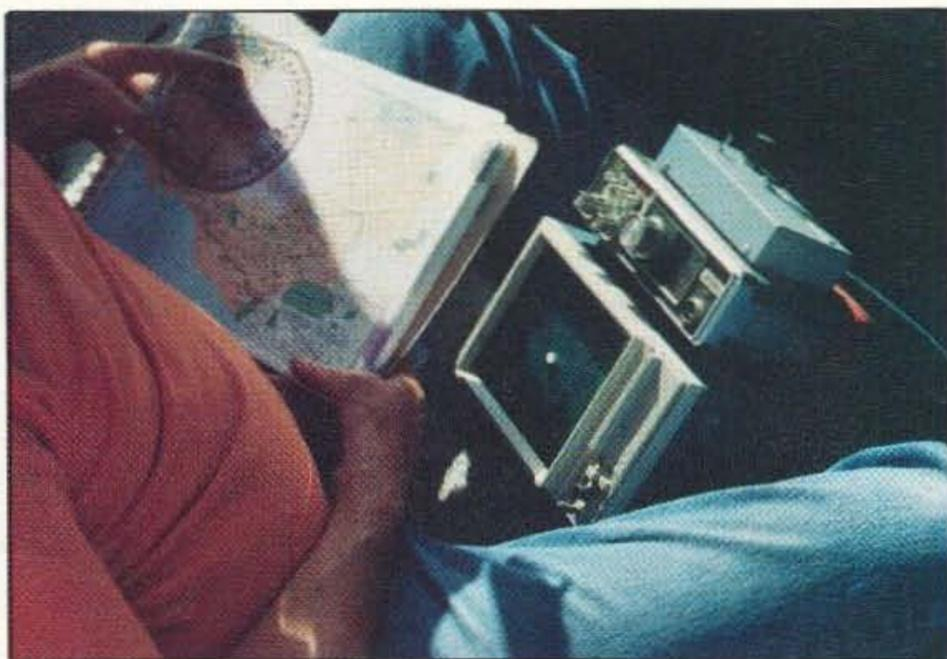
Photo A. KK6CU shows how his mobile CRT display is used. The storage scope is in a very deep cabinet, so it goes on the floor in front of the passenger/navigator.
