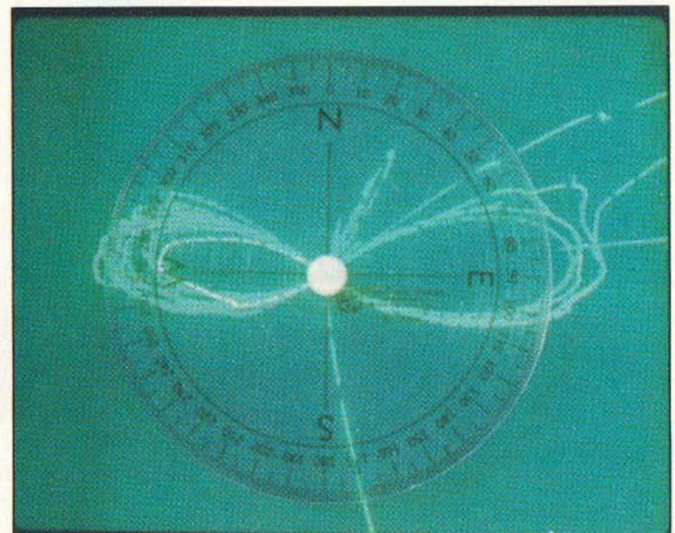
Photo E. A Doppler can't separate two simultaneous signals of equal amplitude, but KK6CU's CRT display and a good beam make it look easy.
