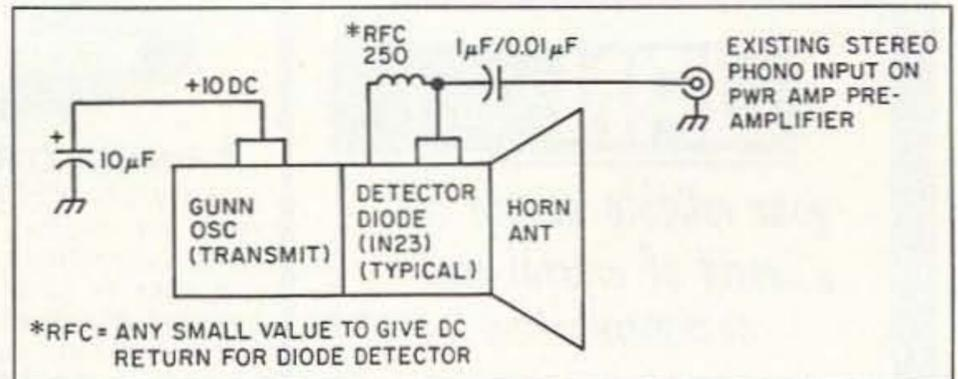
Figure 1. Simple Gunn Doppler "radar" motion detector. Audio tone equals approximately 130 Hz per MPH.
