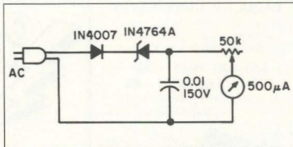
Figure 1. AC line voltage monitor.
