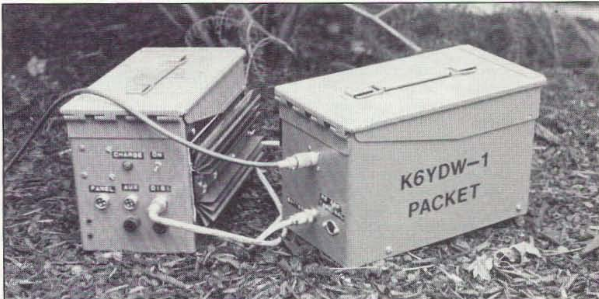
Photo A. The HT/TNC and battery box connected.
