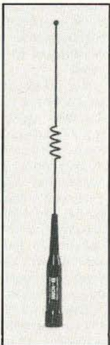
B-10/B-10NMO Dual-Band 146/446 MHz Gain & Wave: 146MHz -dB 1/4 wave 446MHz 2.15dB 1/2 wave VSWR: Less than 1.5:1 144-148MHz, 440-450MHz Max Power: 50 watts Length: 12" Connector: PL-259 or NMO style Construction: Black, cellular lock-a-like w/Fold-Over
