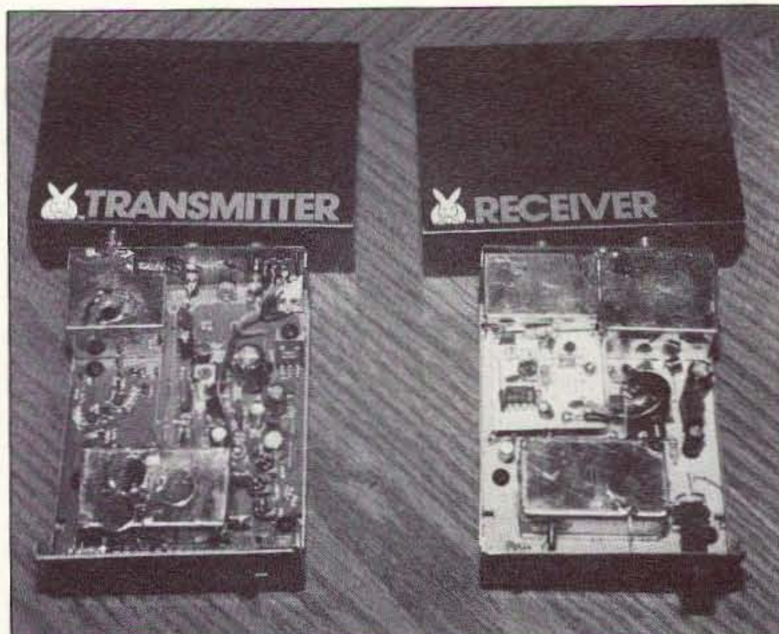
Photo A. The Gemini Rabbit wireless video system consists of a tunable TV transmitter and receiver that operates on the 900 MHz band. (Photo by Jim Pliett K9OMA.)
