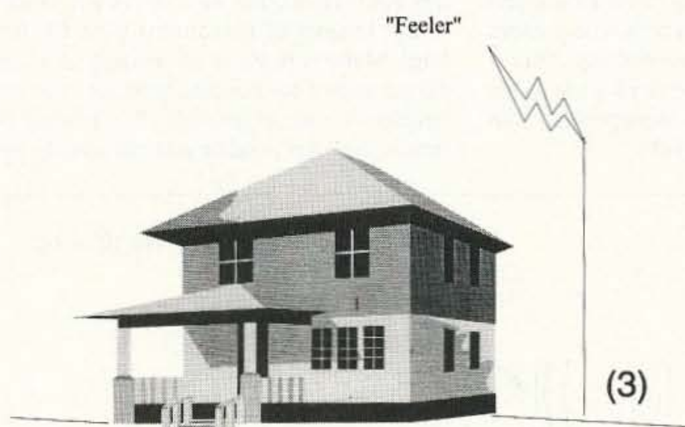
Fig. A3. As the charge increases, a "feeler" begins to form.
