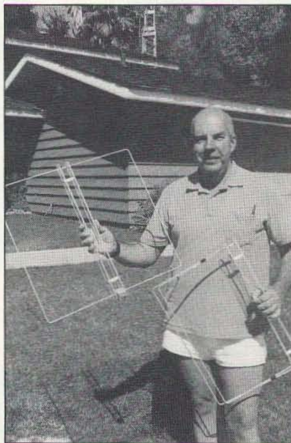
Photo A. The inventor of the Quagi, Wayne Overbeck N6NB, holding the assembled driven element and partly-assembled reflector element from the new Sentech Q144-8 Quagi. Wayne is beaming like a proud papa.
