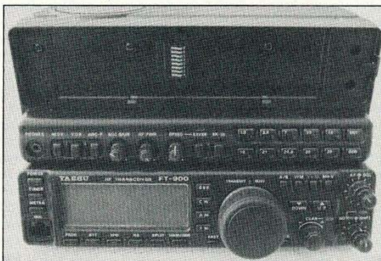
The Yaesu FT-900 with front subpanel detached and resting below the main radio body. See the review on page 10.
