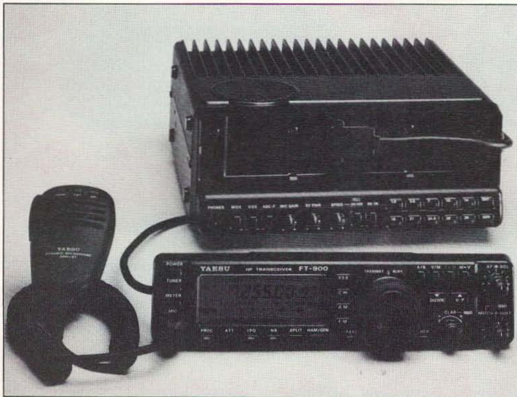
Photo A. The Yaesu FT-900 with front subpanel detached. The subpanel "clicks" off with a finger latch.
