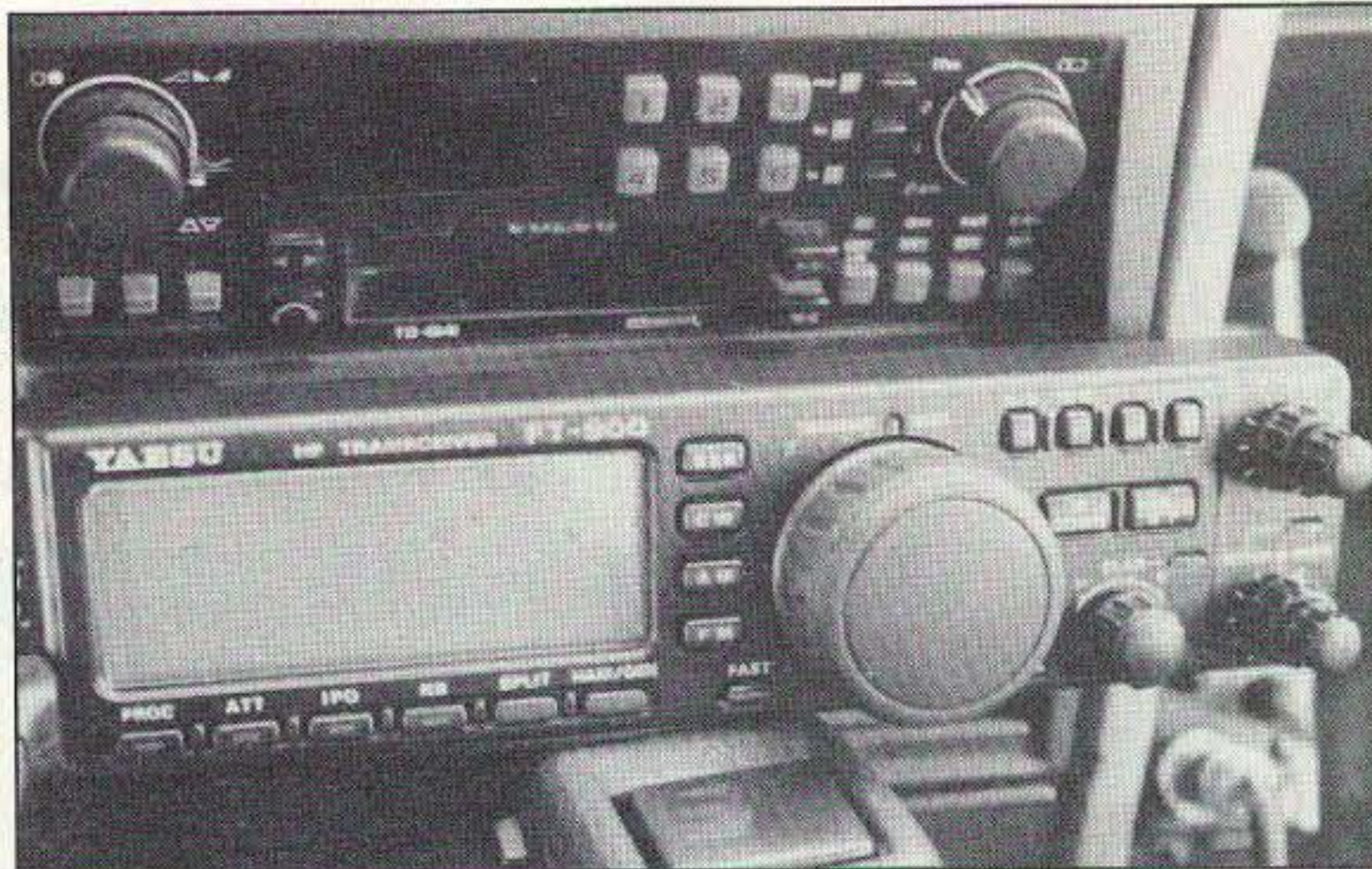
Photo B. The FT-900 subpanel installed in the author's car using Velcro strips. For permanent installations you could use a gooseneck accessory fixture instead.
