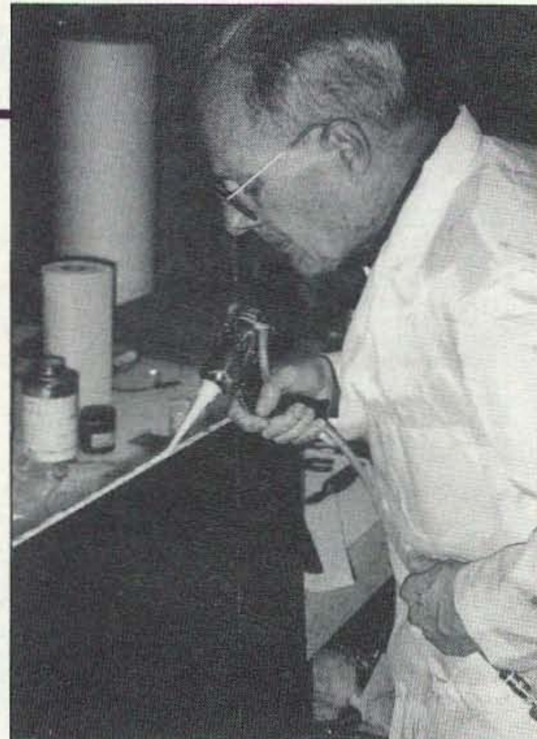
Photo B. Later, Jansson applied epoxy resin to the edge of one of the panels, which are constructed of 1/2" thick aluminum honeycomb material covered by a thin carbon composite facesheet. Each panel weighs only a few kilograms. (Photo by Keith Baker KB1SF.)
