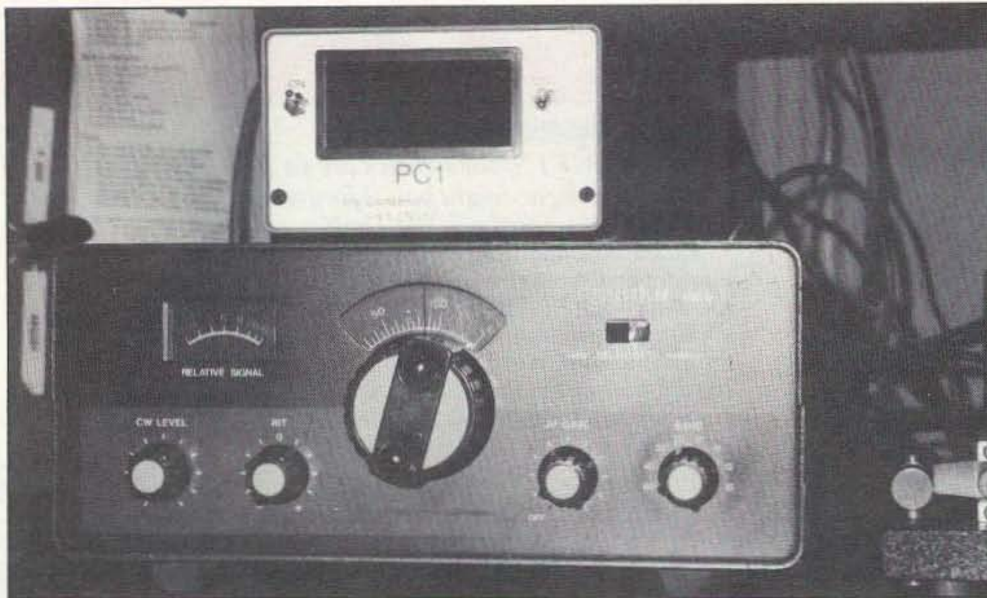
Photo B. The completed PC-1 used as a digital display for the author's HW-9. (Photo by AC4HF.)
