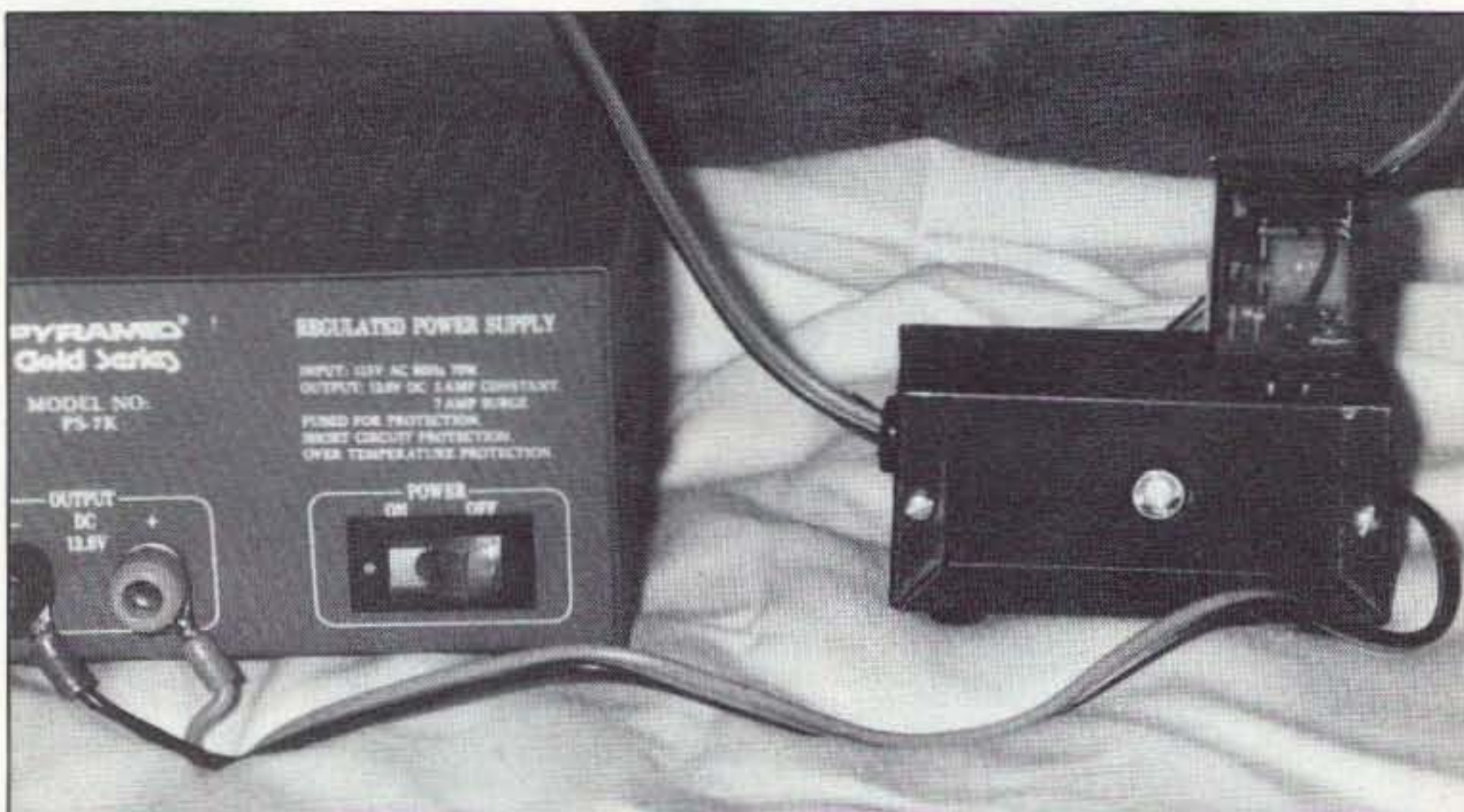
Photo B. The "Foolproof Power Controller" connected to the 13.8-volt DC power supply.
