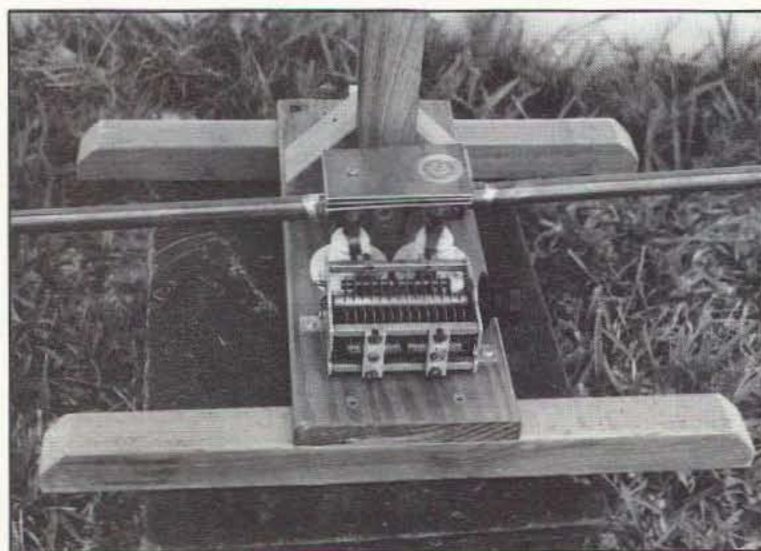
Photo C. Details of the loop antenna base.
