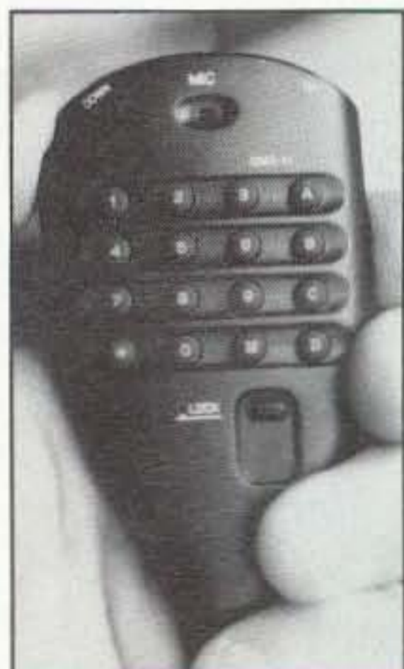
Photo C. The full-featured Alinco 6m mobile microphone.
