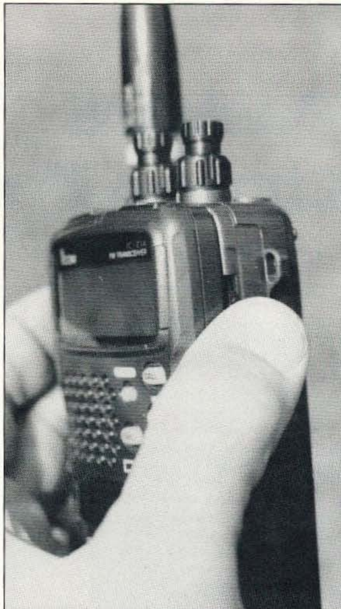
Photo D. The head detaches by moving the release buttons up.
