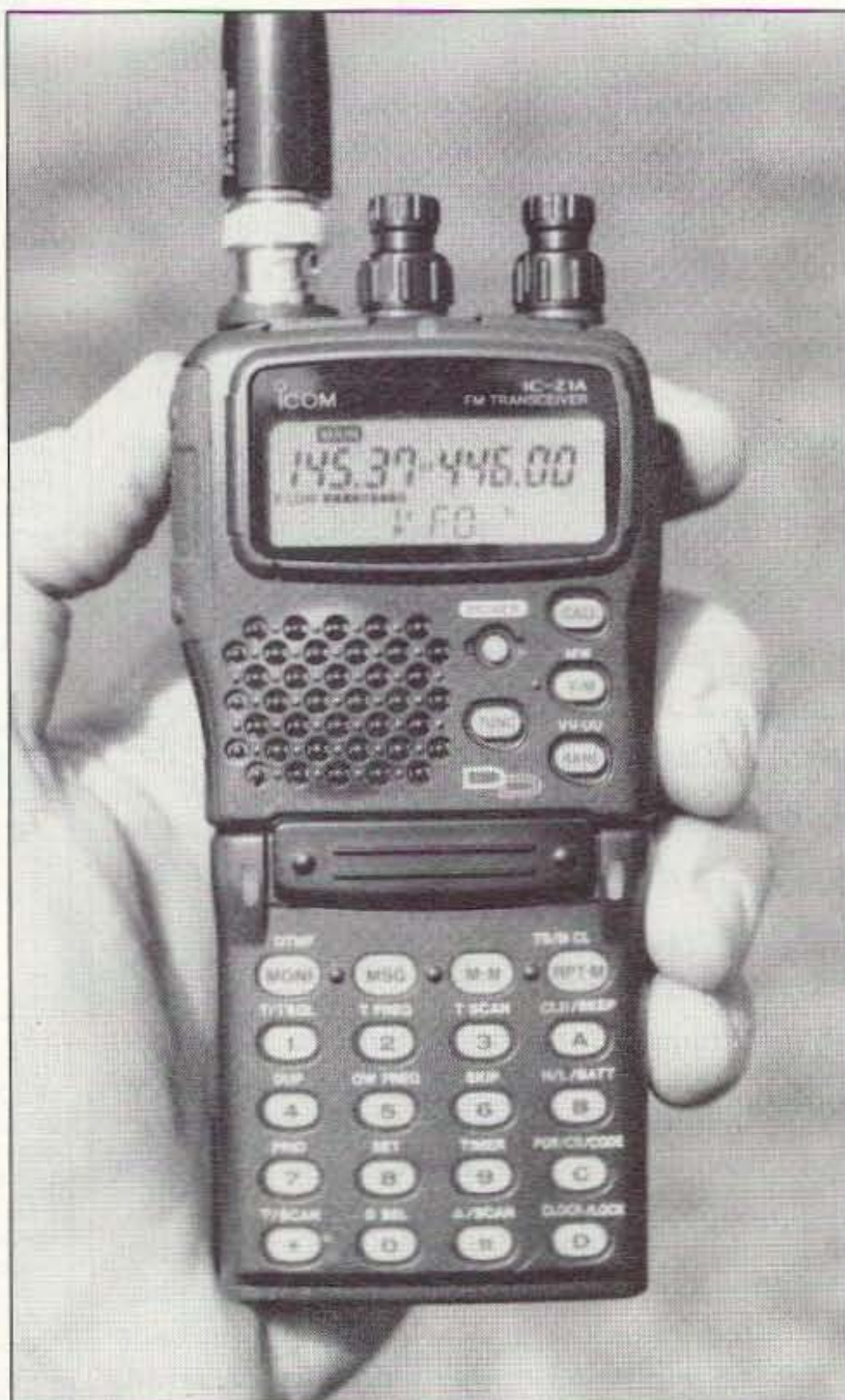
Photo A. The Icom Z1A ran all day on the supplied dry-cell battery pack holder.
