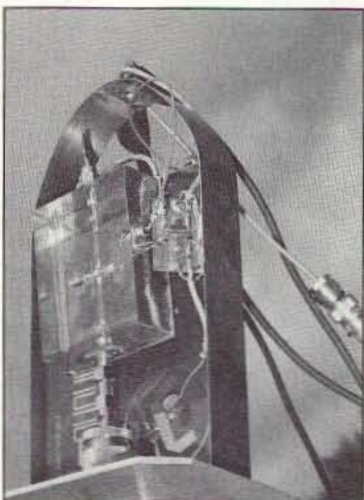
Photo B. The preamp/converter side of a Mode "S" unit using parts from Down East Microwave.
