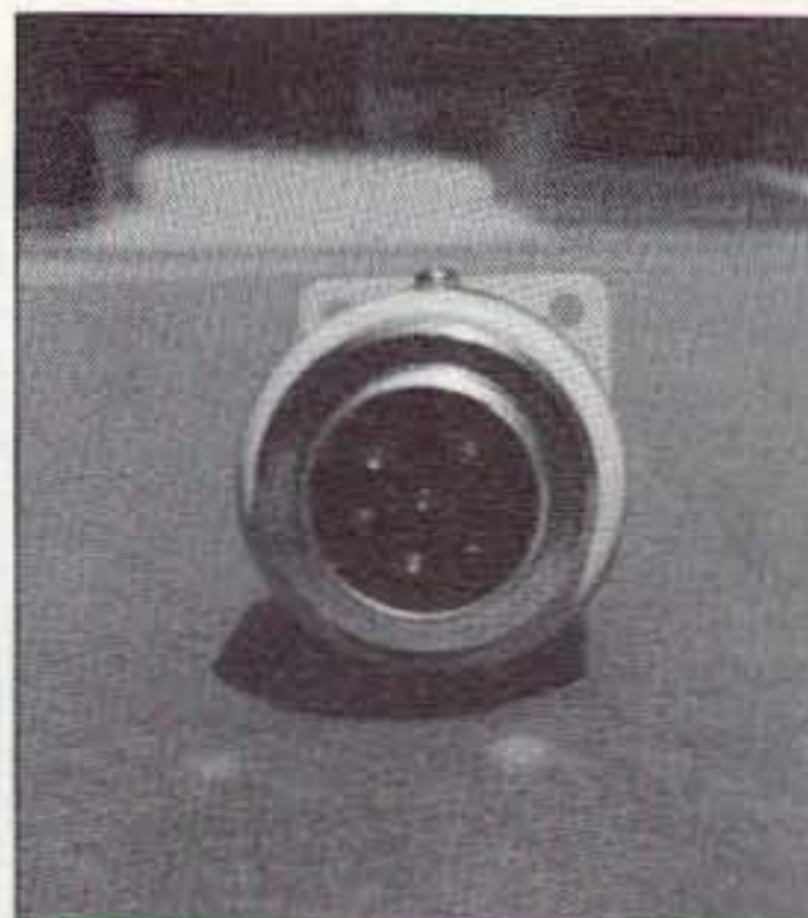
Photo D. Rear cable end connector. Note similarity on pin-out arrangement to Motorola microphone connector.
