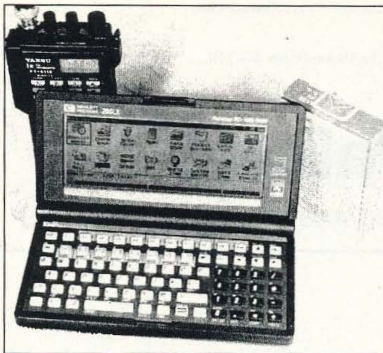
Photo B. The 200LX can control your HF rig via a DOS-based program available for all of the popular rigs that sport a computer connection.
