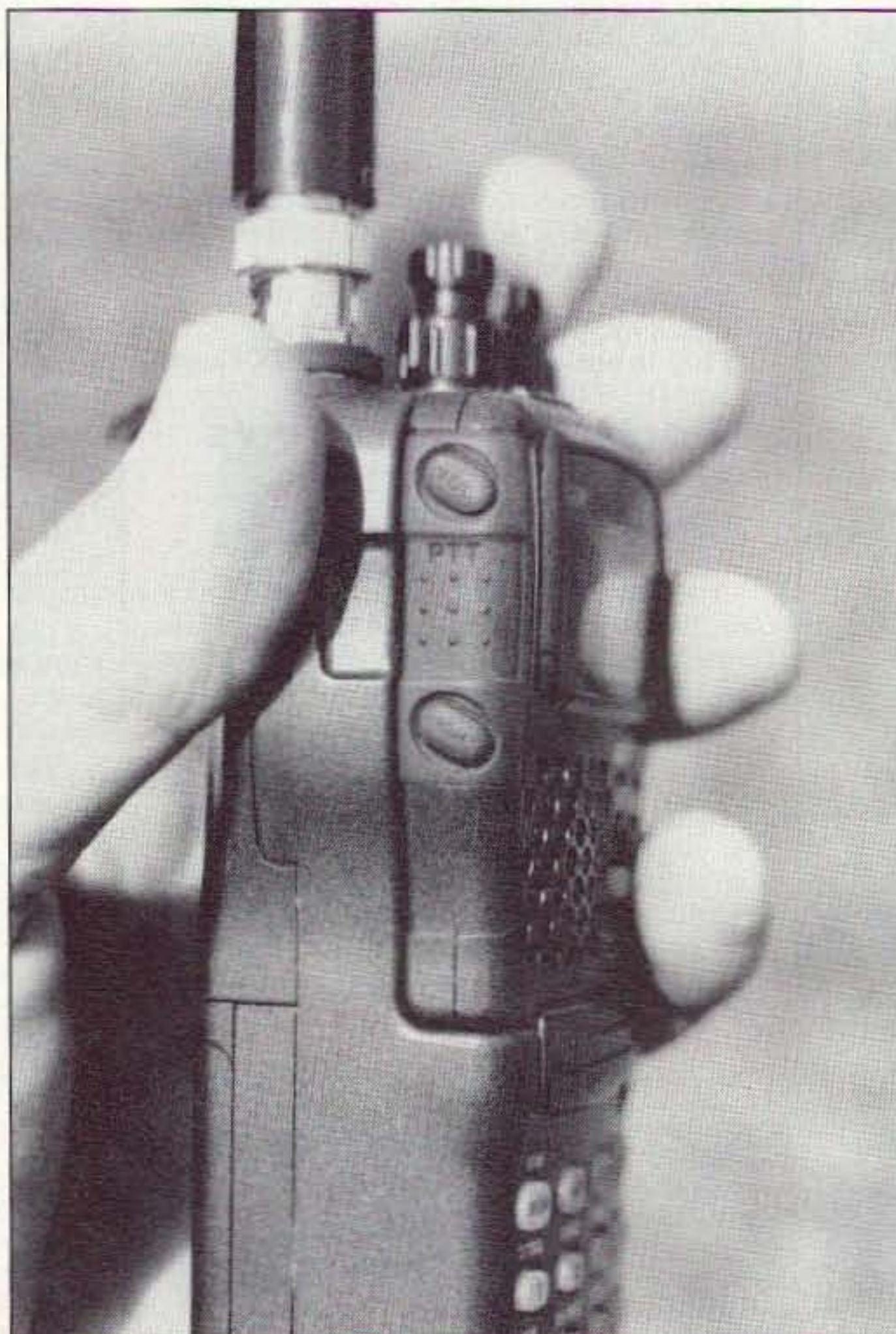
Photo C. You can see where the head detaches from the Z1A body.
