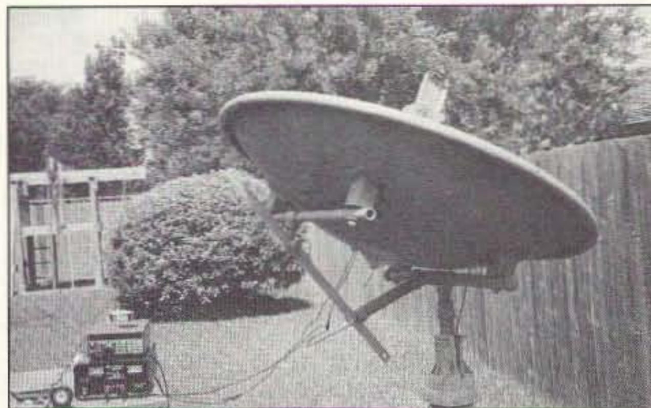
Photo A. Early Mode "S" experiments at WA5ZIB used a 4-ft dish.
