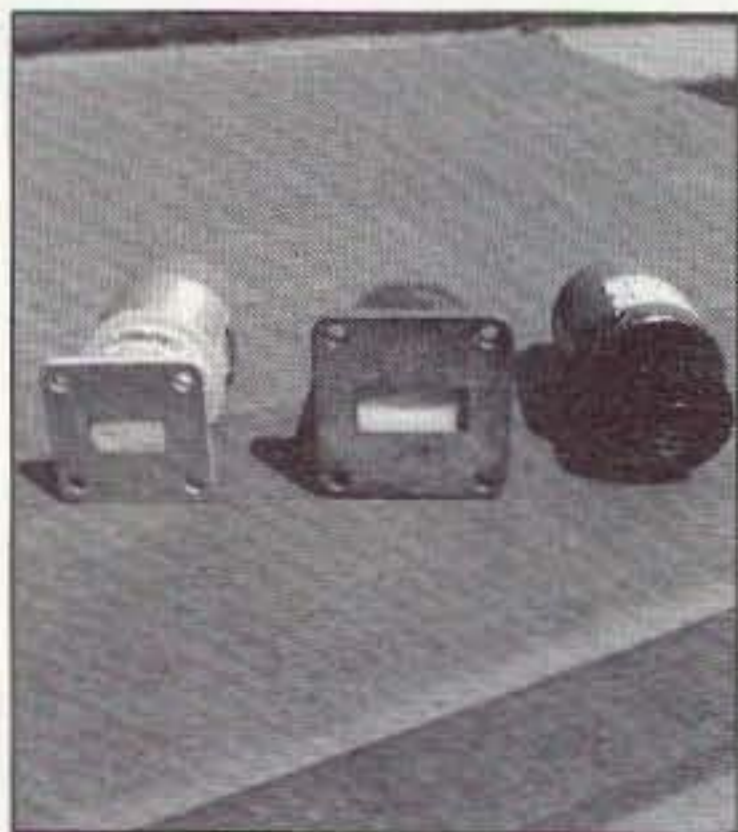
Photo B. Front-end view of three different power heads. Left and center: 12-18 GHz and 8-12 GHz waveguide types. Far right: 478A coaxial 10 MHz to 12 GHz.
