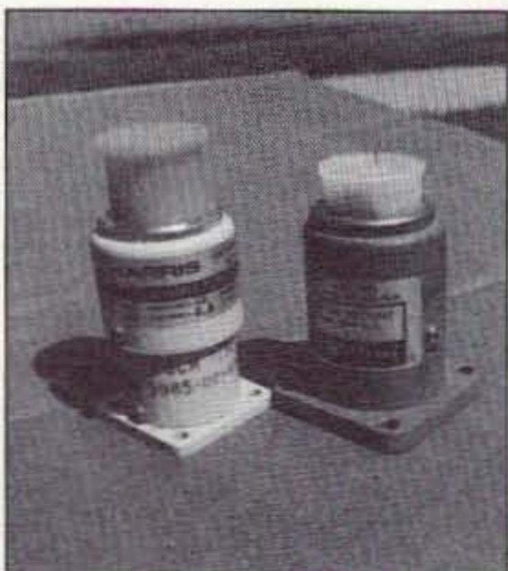
Photo C. Side view of the 18-GHz (left) and the 10-GHz (right) RF power meter heads.
