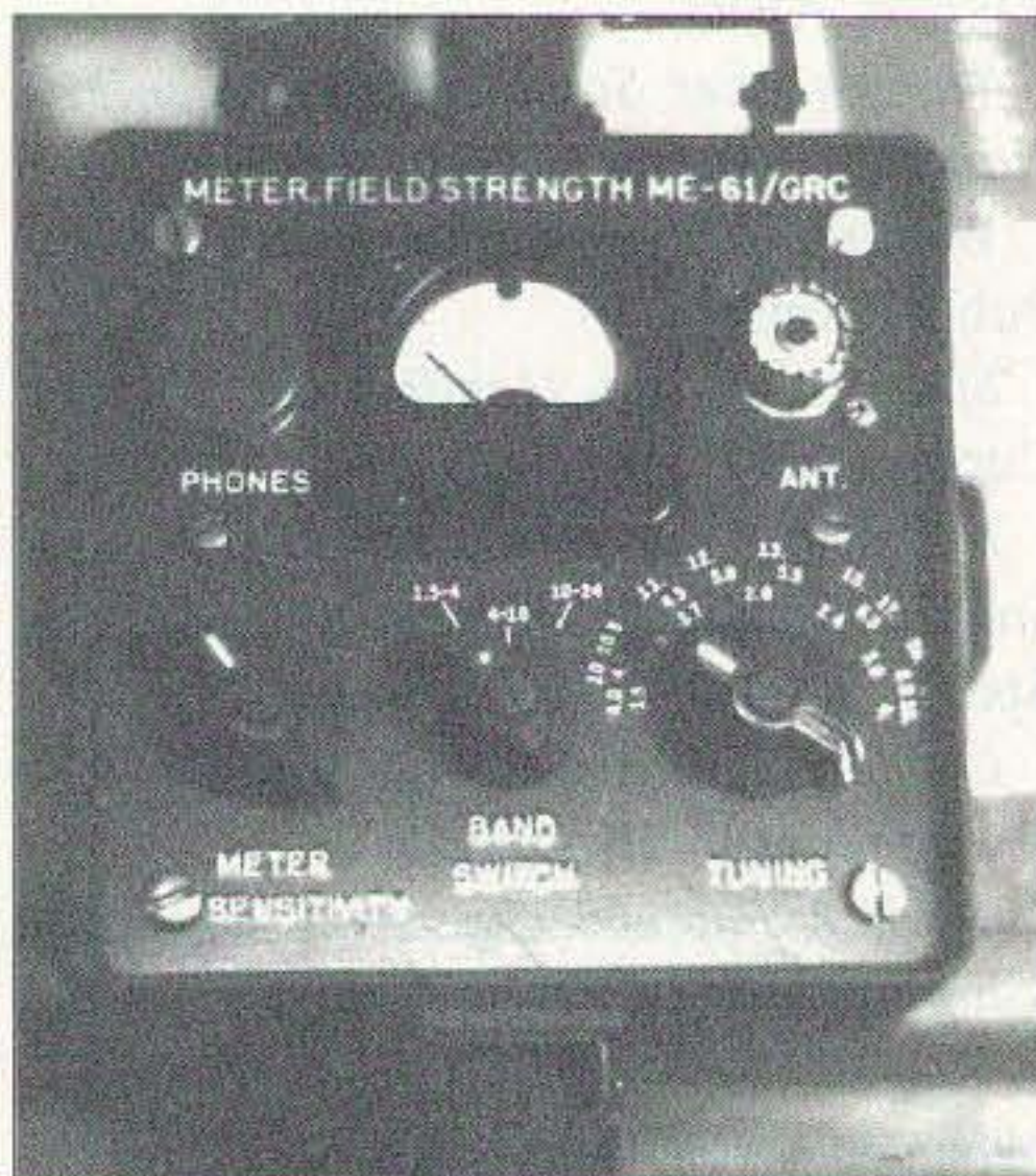
Photo A. The ME-61/GRC field strength meter with the SO-239 connector.
