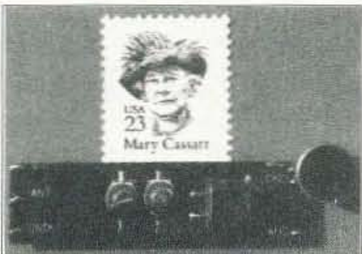
Photo A. The Agrelo Engineering HPVFC micro-transmitter is factory-tuned into a 50-ohm load with the trimmer capacitors on this side of the board. On the other side are 46 SMT components.
