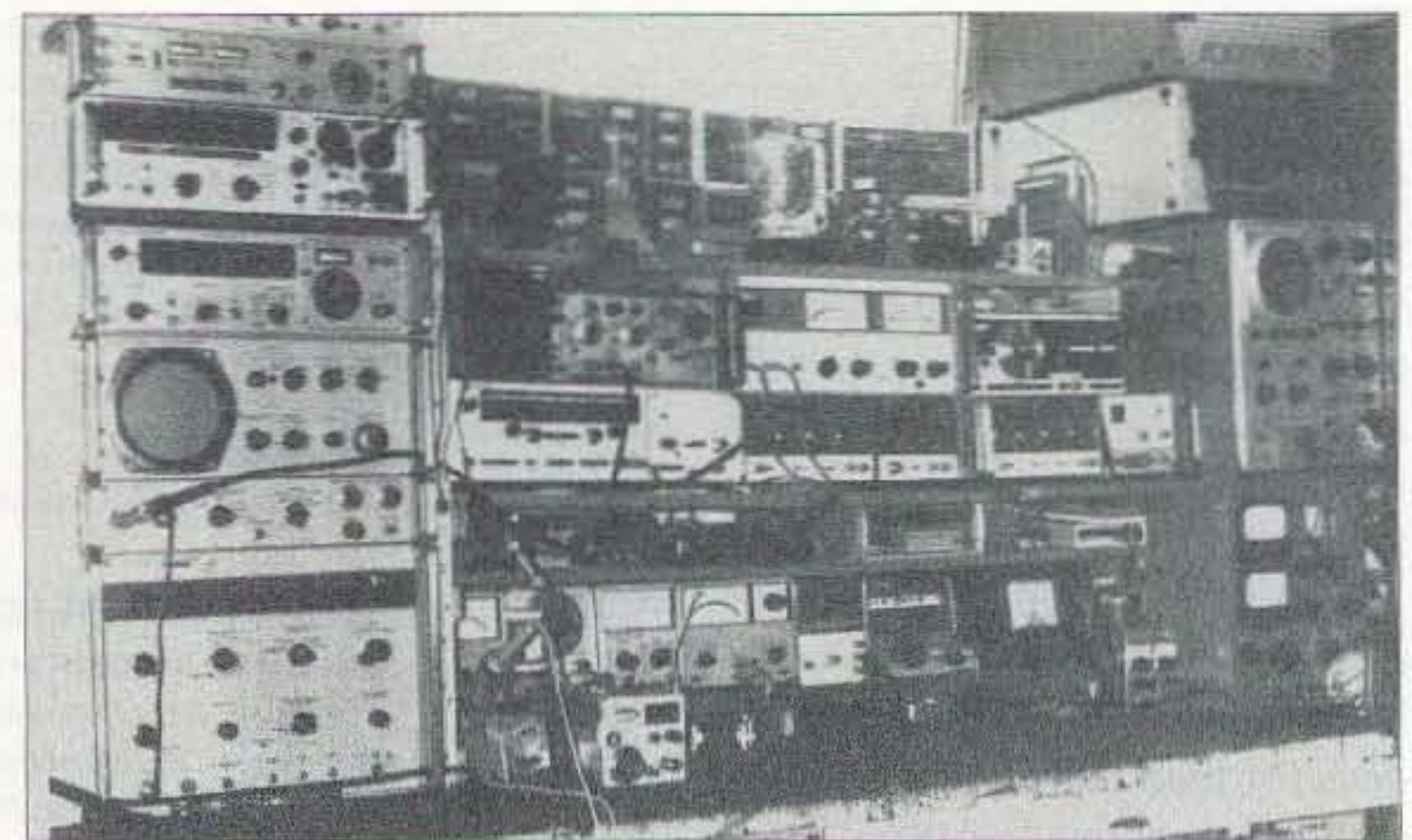
Photo B. The test workbench at WB6IGP. It's equipped with spectrum analyzers, sweepers, signal generators, vector voltmeters, scope and plain old VOM and solderings—a lot of junk that the power company would be proud of if I turned it all on at one time! This is where most projects get the final test.
