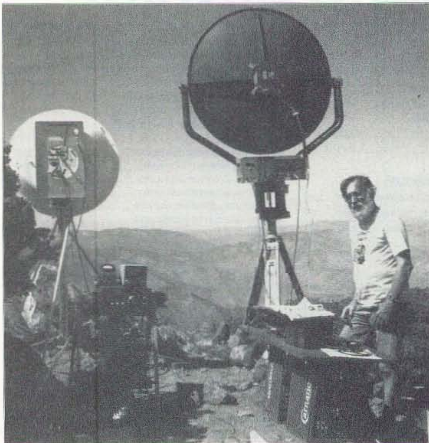
Photo A. Microwave operation in the San Diego mountains at an elevation of 6,000 feet above sea level. Making contact over the distant mountains required antenna alignment to be accurate within 1 or 2 degrees on the compass. Just beyond this vantage point, the mountain drops off 5,000 feet to the desert floor.
