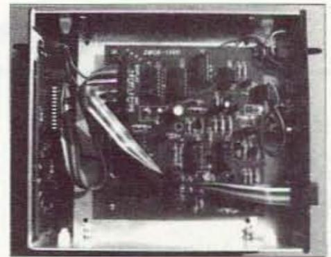
**Photo C.** Processing and display electronics are on separate boards in the Directional Systems Doppler unit.
