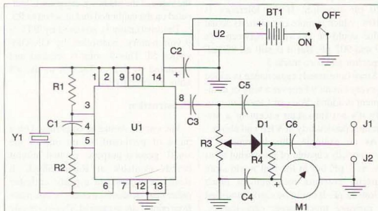
Fig. 1. Schematic diagram for the simple capacity meter.
