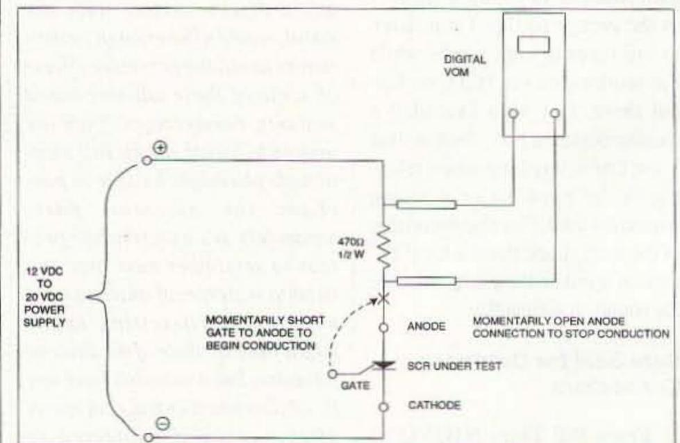
Fig. 1. AD4UA's simple SCR test circuit.
