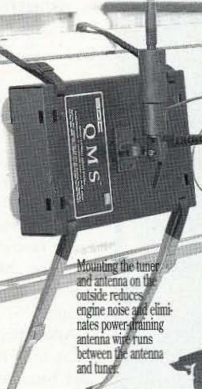
Mounting the tuner and antenna on the outside reduces engine noise and eliminates power-draining antenna wire runs between the antenna and tuner.
