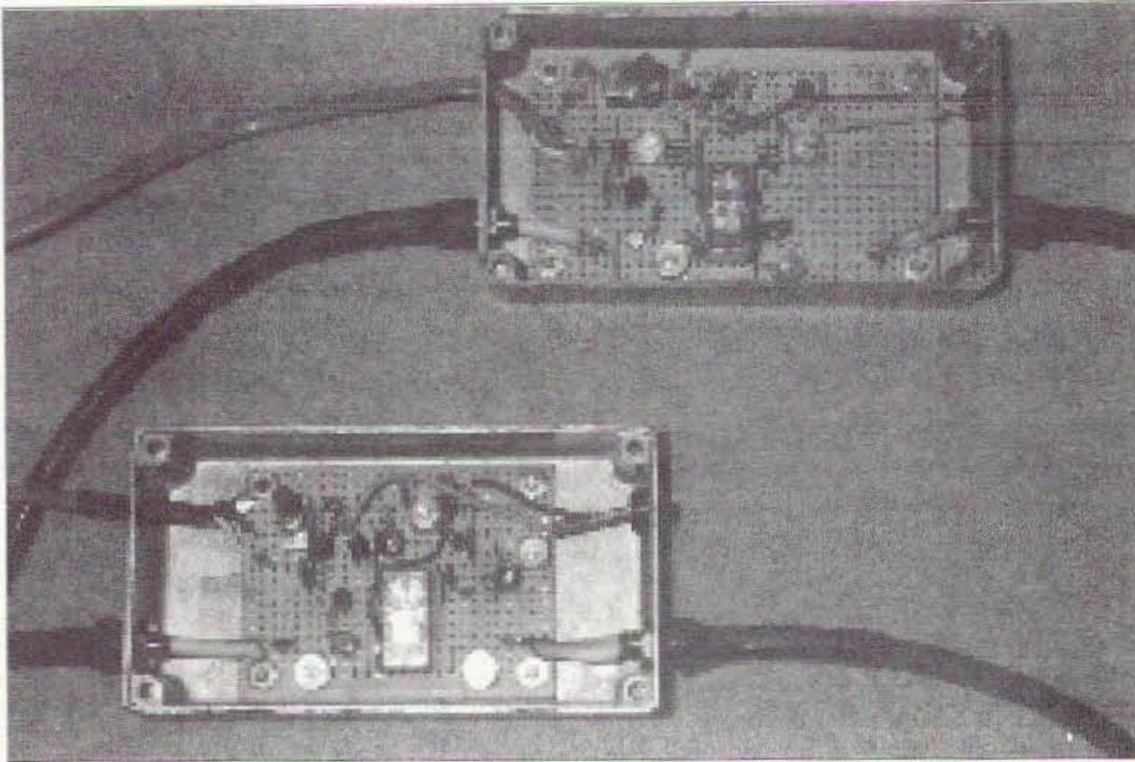
**Photo A.** A bipolar transistor preamplifier at the top (MRF901), and an FET preamp at the bottom (BF981). Both have the same RX-TX switching using a single relay and the die-cast box as the ground reference for the preamp. The box also is in the direct return path from the antenna.
