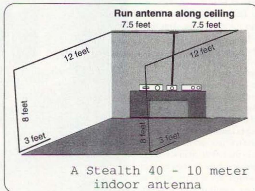
Fig. 1. Antenna installation diagram.
