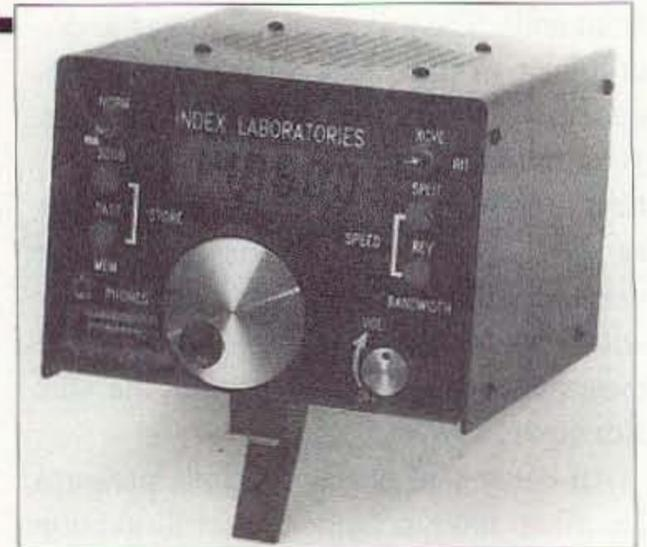
minute by pressing both the Bandwidth and the Rev buttons at the same time. The main tuning knob adjusts the speed in 5 wpm increments. When the Bandwidth button is pressed the bandwidth is displayed, along with the SSB/CW display. To change modes you push the Fast button while holding in the Bandwidth button. The memory of frequencies is stored by pressing the Fast and Mem buttons simultaneously.
