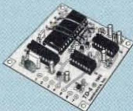
**TD-3 CTCSS DECODER/ENCODER.** Prevents access to repeater or receiver unless proper tone is present. Tone output for transmitters, too. ....kit \$29, w/t \$59
