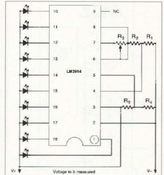
Fig. 1. Shows the schematic of the Tic Tac Tester. It's easy to build, accurate and can be carried in your shirt pocket.
