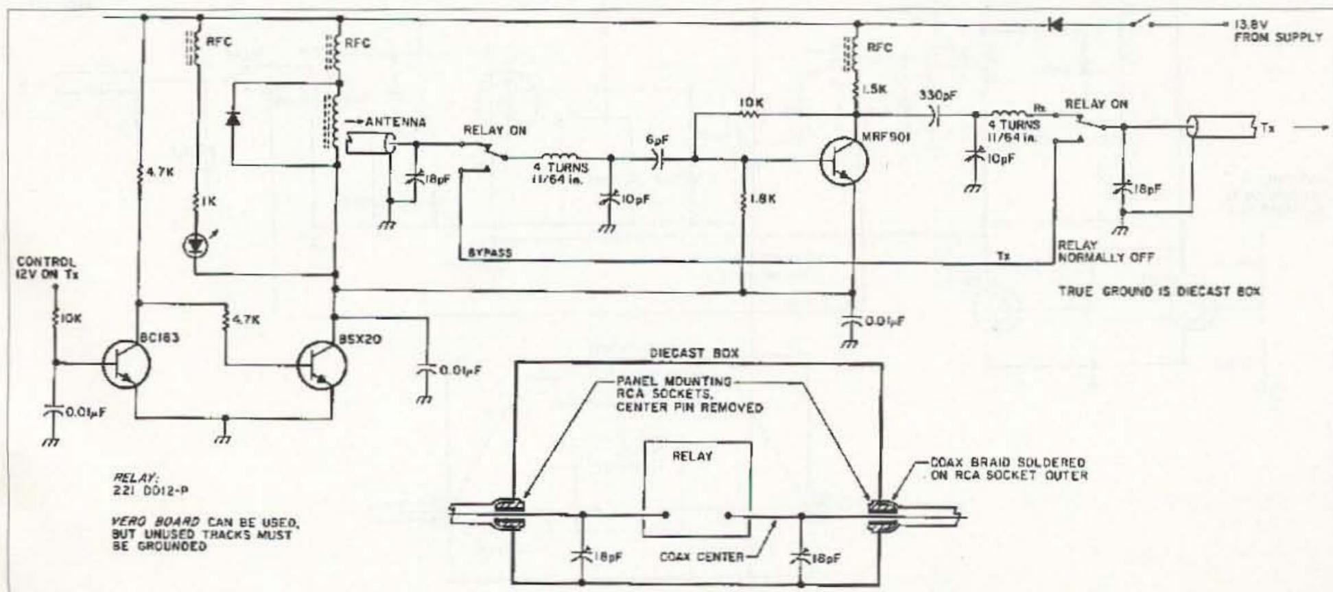
Fig. 1. A simple preamp that actually works.
