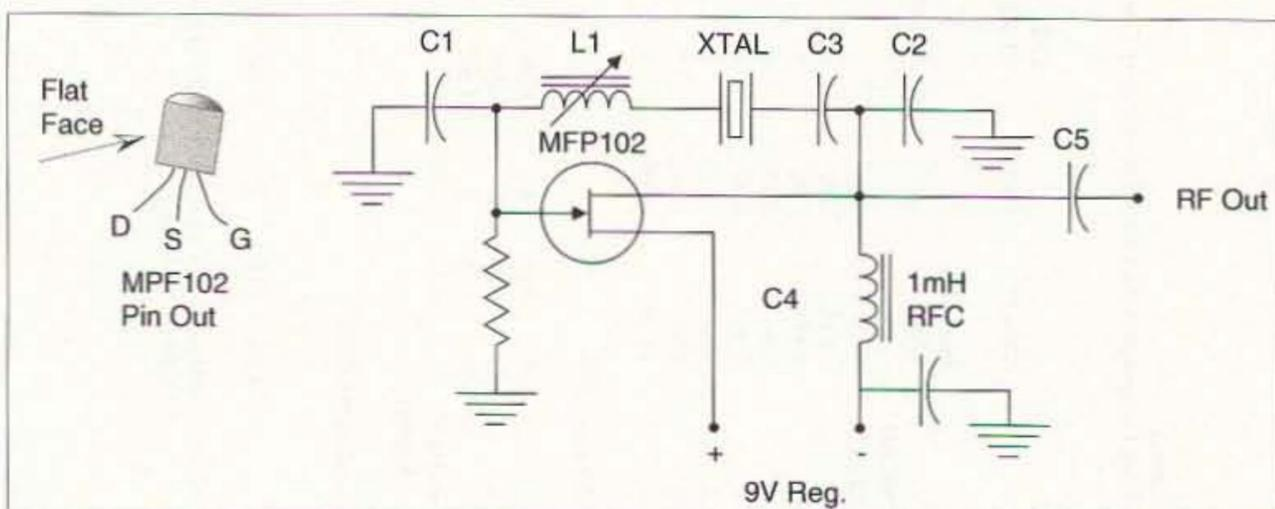
Fig. 1. Oscillator circuit.
