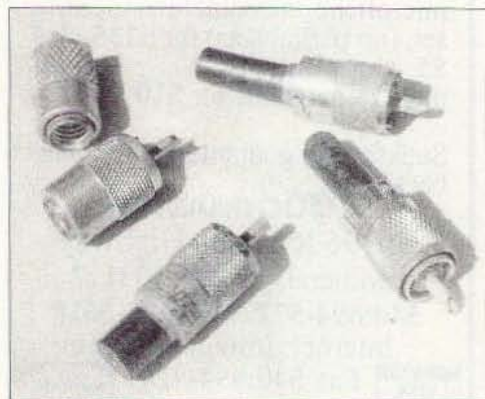
Photo A. PL259s with short cut-off lengths of 8u cable attached, 25¢ each.
