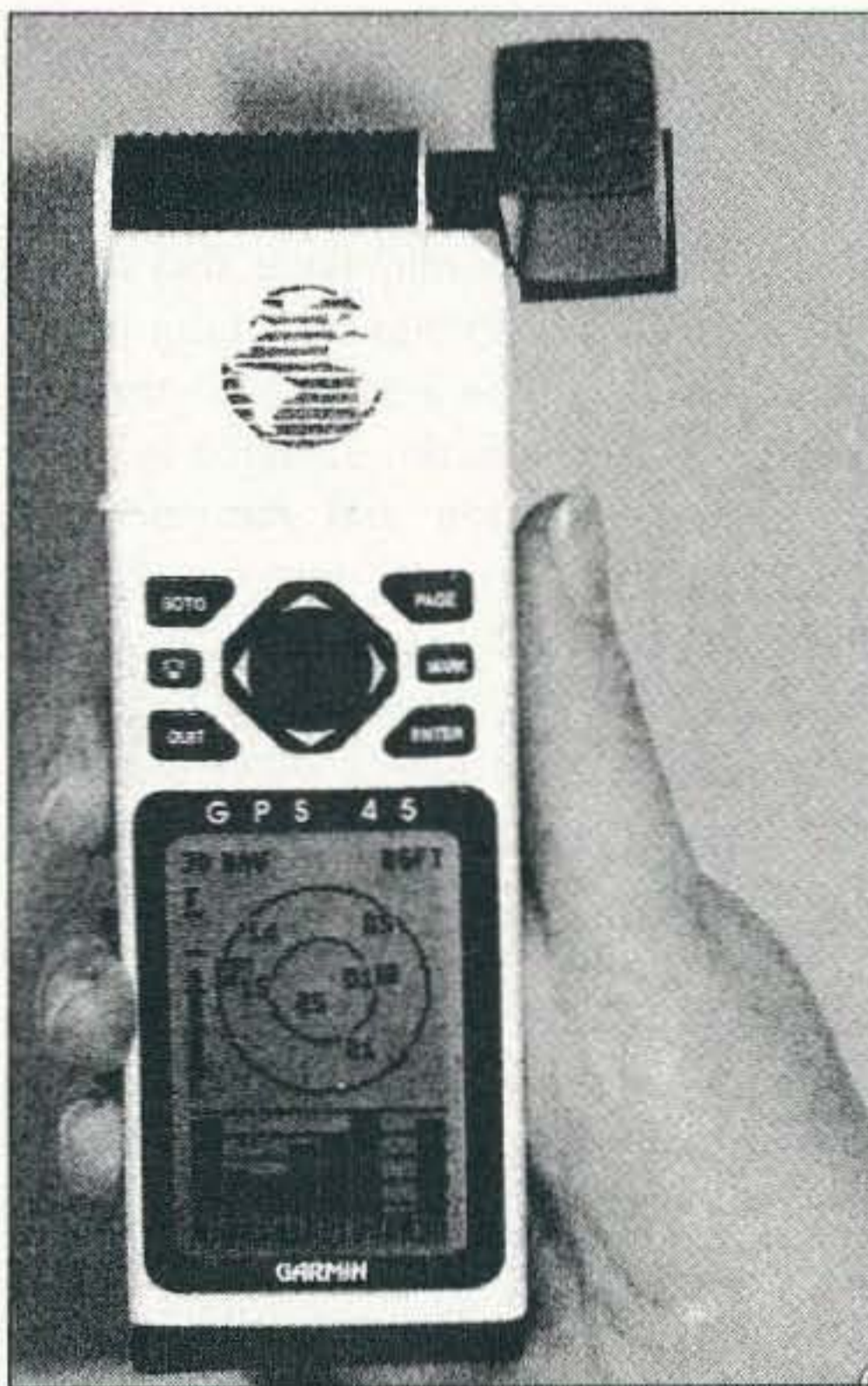
Photo A. Satellites are graphically depicted as being either on the horizon, at 45 degrees up from the horizon or overhead. The display also indicates the satellite's ID number, along with a relative signal strength bar for each of the satellites being tracked.
