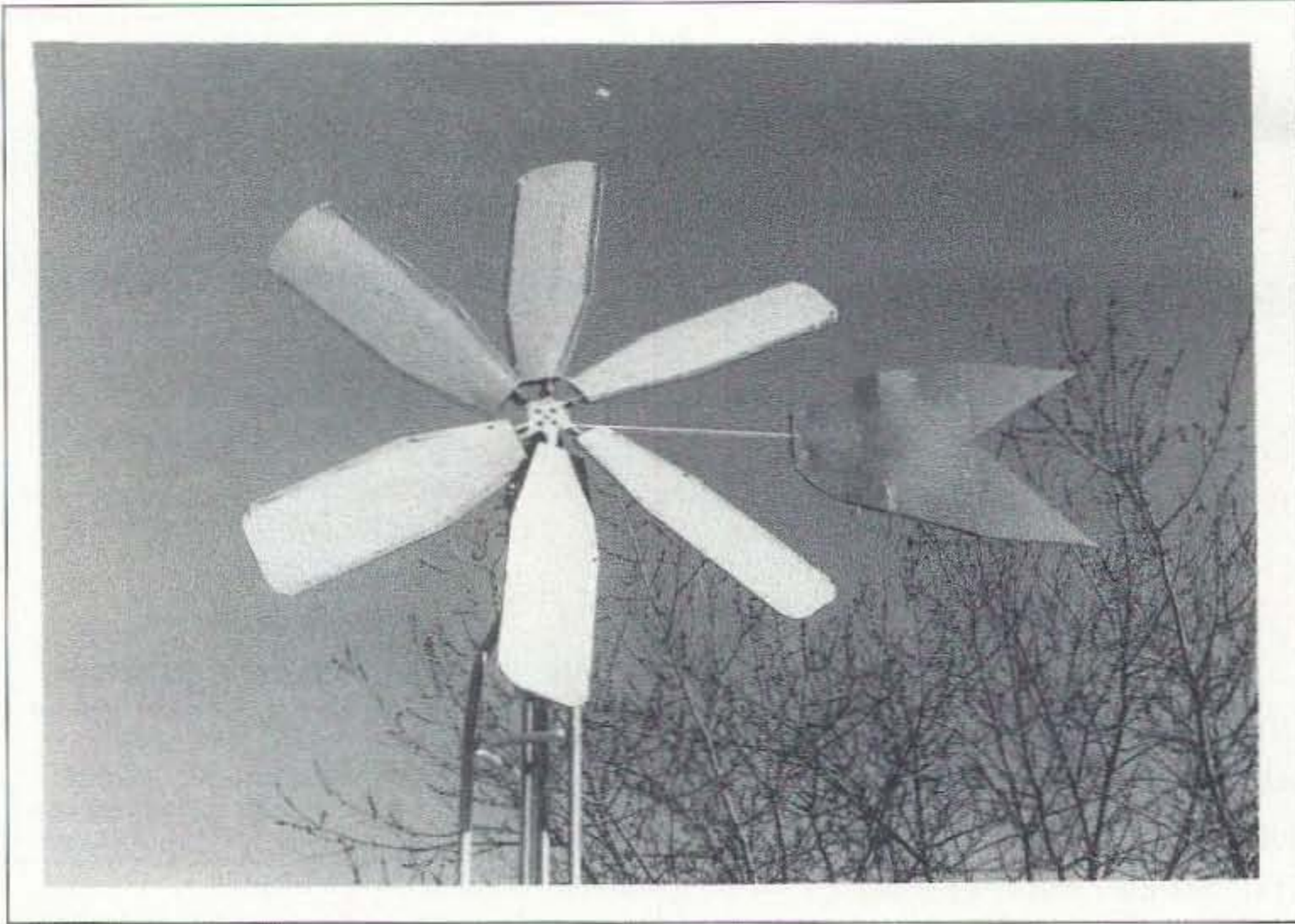
Photo D. The wind generator helps keep the batteries charged when the Sun is nowhere to be found. The tail is folded to prevent damage to the rotor in high winds.
