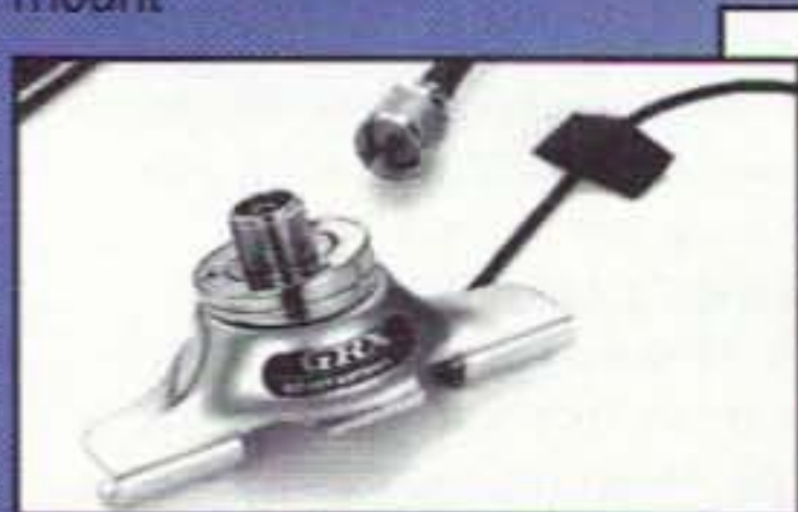
GR-5M Deluxe trunk lip mount. Rubber coated base protects the vehicles paint. All stainless steel, includes the CK-3M5 deluxe cable assembly to avoid water leads/cable damage when shutting the trunk. Four large set screws hold it securely in place. Two offset washers adjust the antenna to vertical. Gold-plated SO-239/PL-259 connectors.
