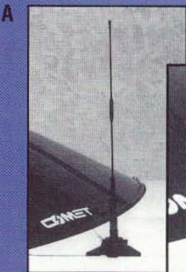
GR-5M Deluxe trunk lip mount. Rubber coated base protects the vehicles paint. All stainless steel, includes the CK-3M5 deluxe cable assembly to avoid water leads/cable damage when shutting the trunk. Four large set screws hold it securely in place. Two offset washers adjust the antenna to vertical. Gold-plated SO-239/PL-259 connectors.
