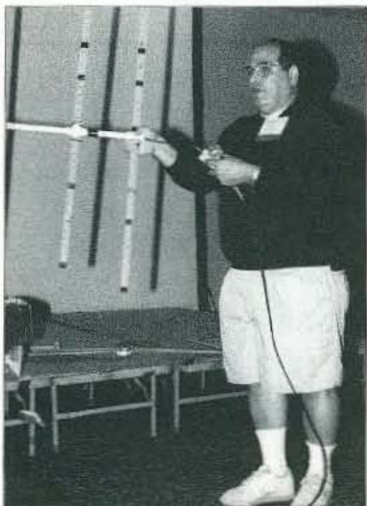
Photo C. Tape-measure beams are very popular for on-foot fox-hunting. Joe Leggio WB2HOL shows his three-element version at the Dayton Foxhunt Forum.
