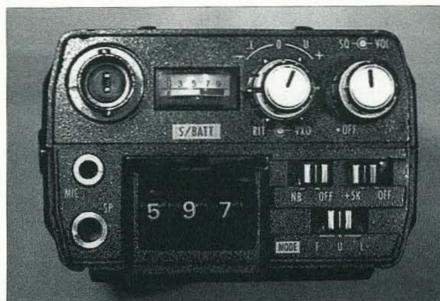
Photo F. The older 2-meter multimode Santec LS-202A HT had pots and switches on the top to control operation.
