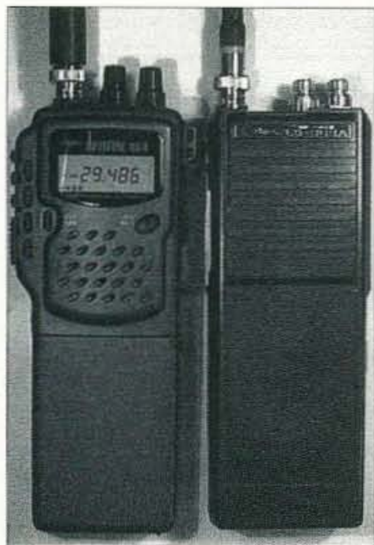
Photo D. The new Eagle Spitfire 454 10-meter HT is nearly identical in size with the much older Santec LS-202A 2-meter HT. Both are multimode radios with full band coverage.
