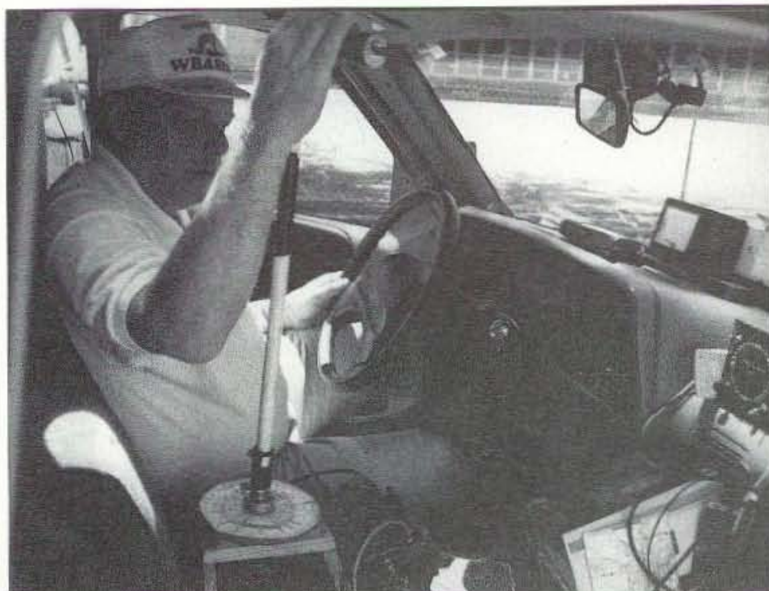
Photo A. Dick Arnett WB4SUV has a well-equipped mobile T-hunt setup including a doppler and a storage-scope display.
