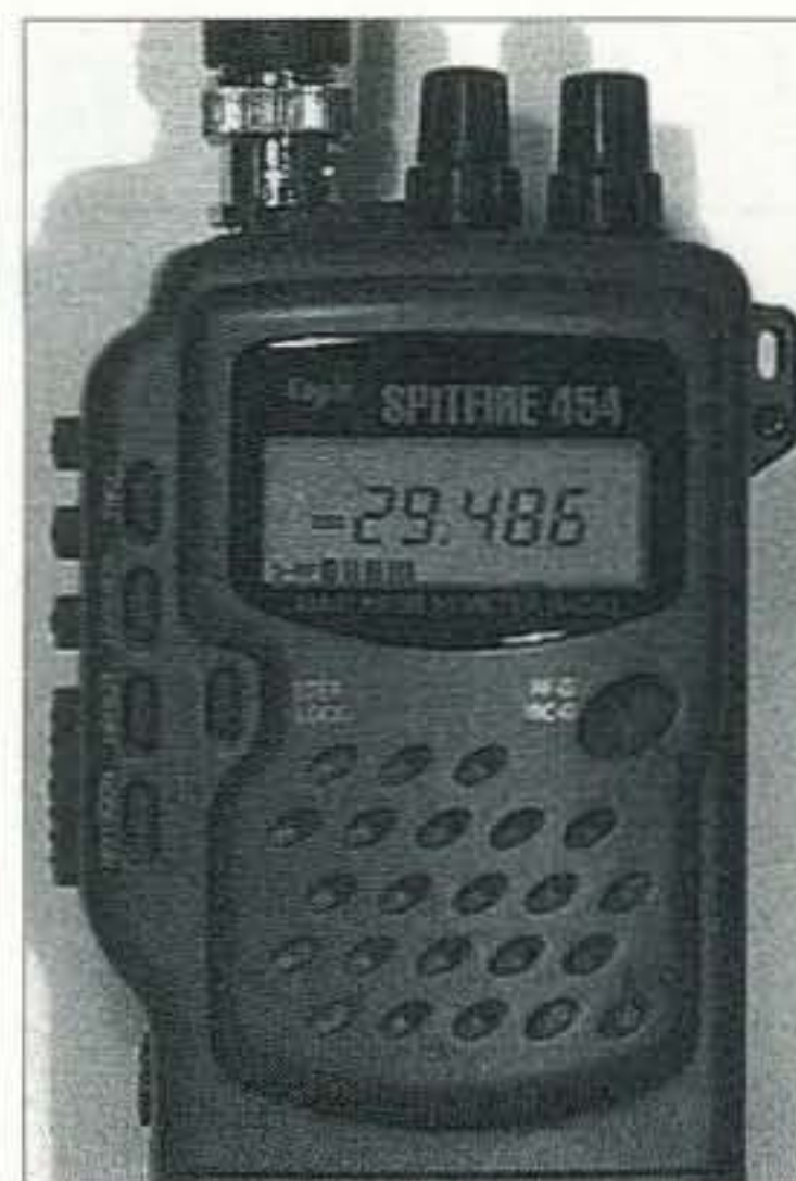
Photo E. A close-up of the Eagle Spitfire 454 10-meter HT. Most controls are buttons on the front or side of the radio.
