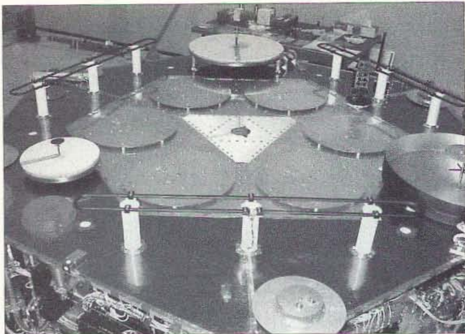
Photo C. The "Earth" side of Phase 3D has sprouted many antennas in this pre-vibration-test photo. (W3IWI photo)
