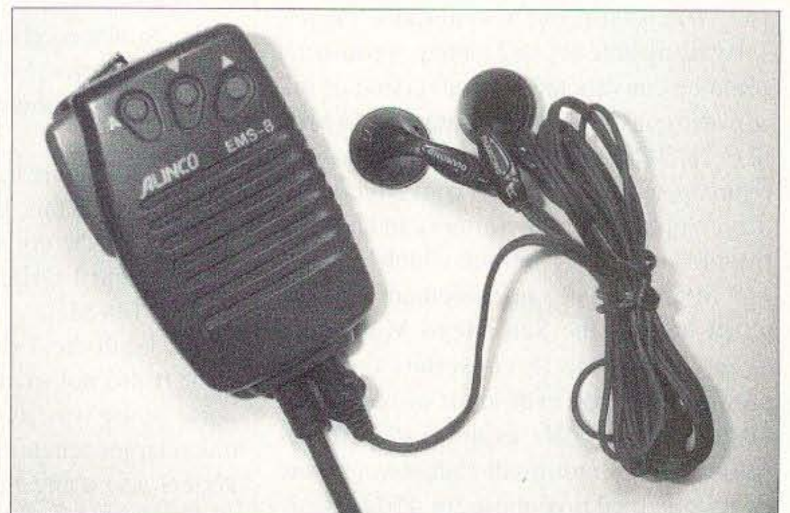
Photo B. The Alinco EMS-8 speaker/mike and earbud headphones ready for AO-27.
