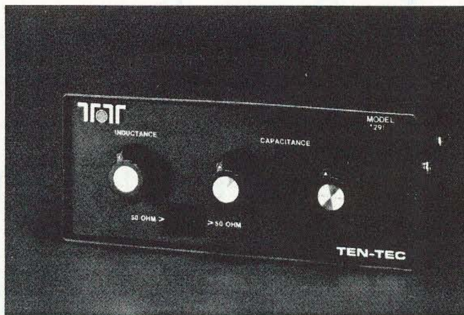
Photo D. Ten-Tec makes this small tuner that's perfect for mobile use or QRPing in the field.
