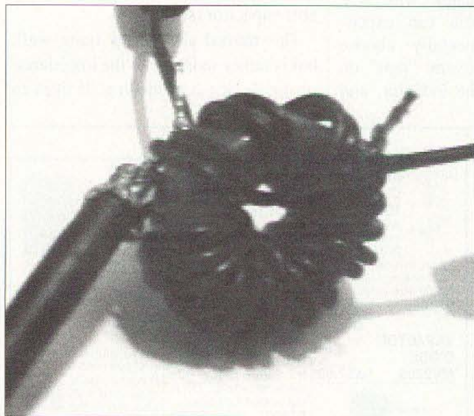
Photo L. Winding and construction of the 4:1 balun.
