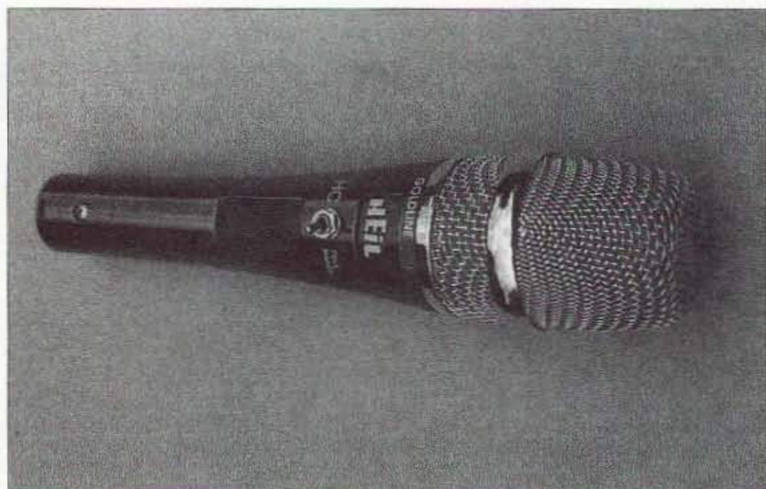
Photo A. Heil Sound's new "GoldLine" microphone is the ideal way to have a terrific studio grade sound plus a pileup-busting signal for DXing with one economically priced mike. What's the secret? It has two elements you select as desired by a small toggle switch mounted above the PTT slide switch. Details in text.
