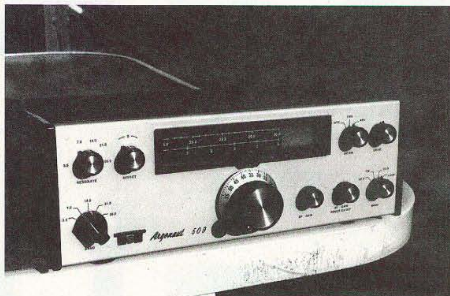
Photo B. The Ten-Tec Argonaut 509 has a built-in SWR meter. As a matter of fact, all the Argonaut series have SWR meters. Don't use an external SWR meter if your rig already has one inside. It's a waste of watts.
