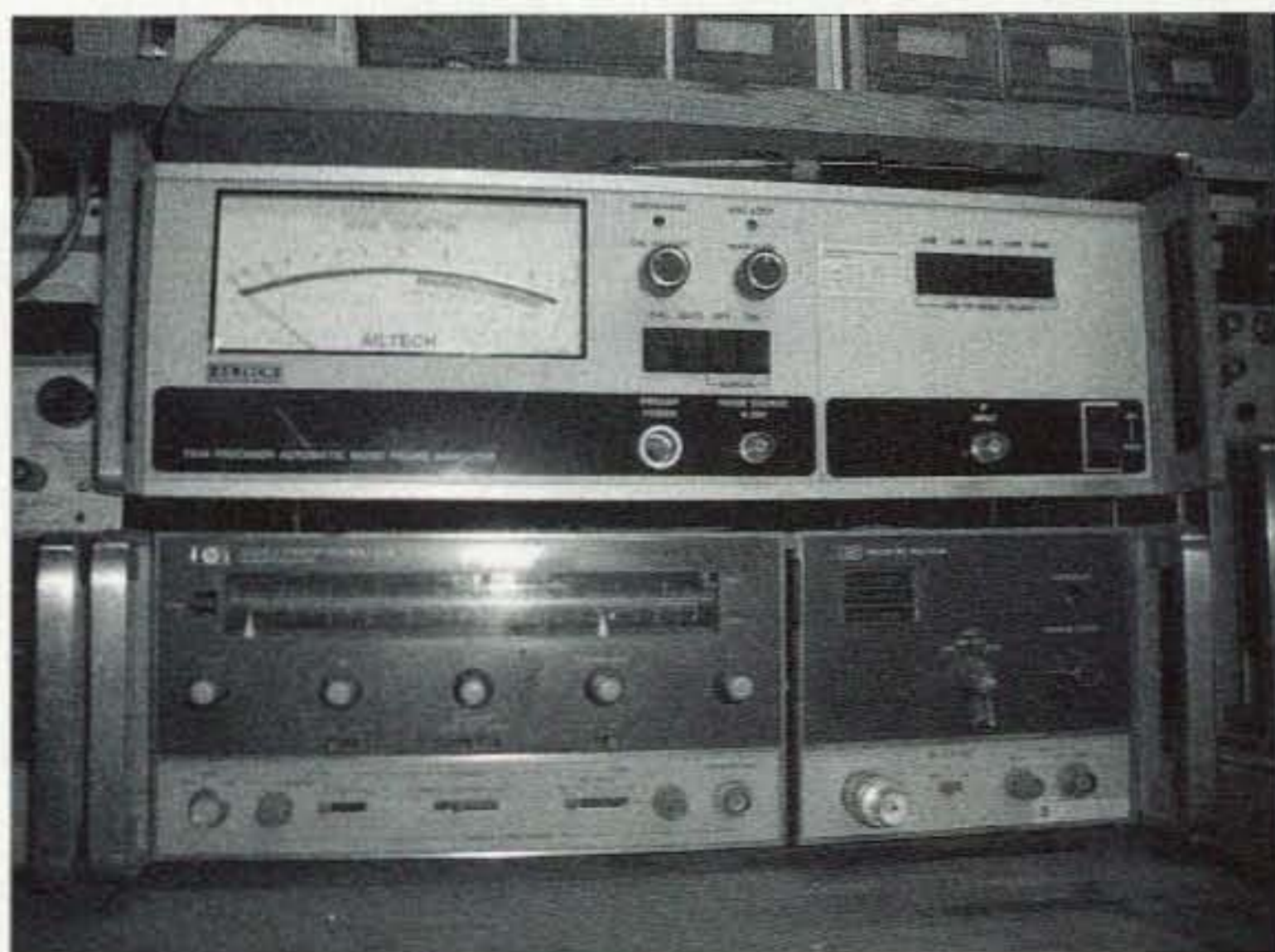
Photo A. The Ailtech 7514 noise figure meter and HP-8620C sweep oscillator are used with mixer as local oscillator for making noise figure measurements at microwave frequencies from 5-10 GHz.
