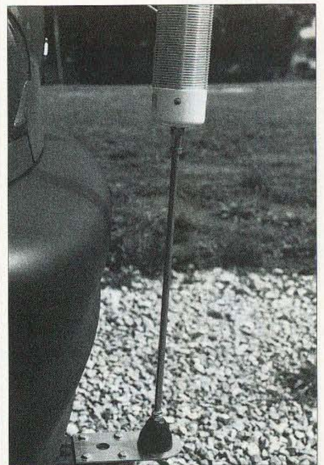
Photo B. This short shaft was eventually replaced to increase the height of the loading coil. Notice the metal mounting bracket from under the car's body.
