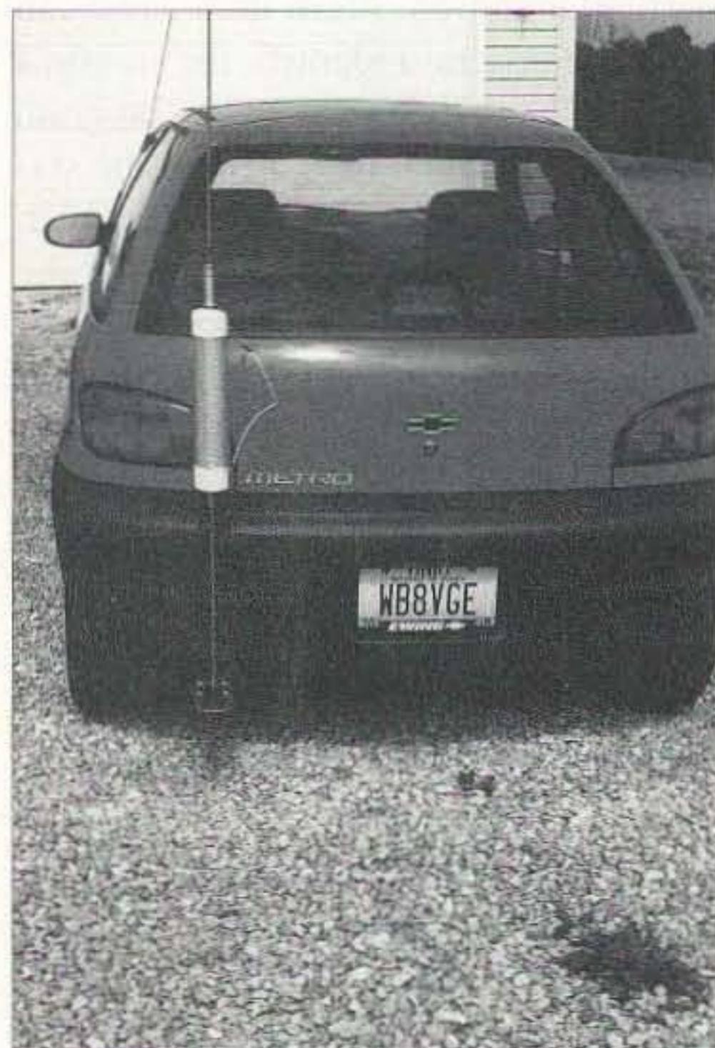
Photo A. This is the first version of the mobile antenna installation. Notice how short the loading coil is compared to the car's body.
