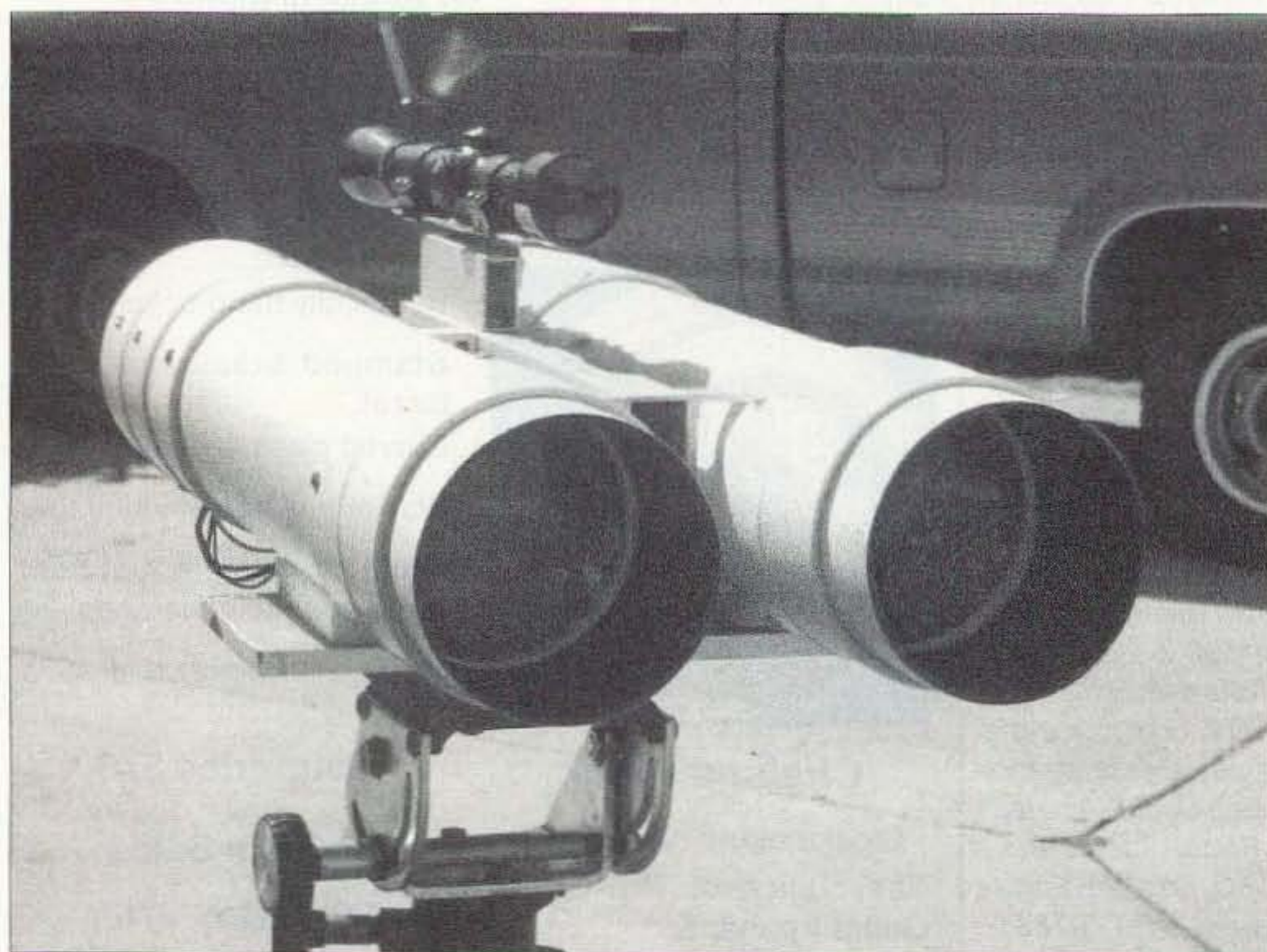
Photo A. Front view of entire system showing spotting scope on top, centered between the receiver and transmitter 4-inch assemblies. Visible just inside the front of each tube is the Fresnel lens in the splice union coupling.
