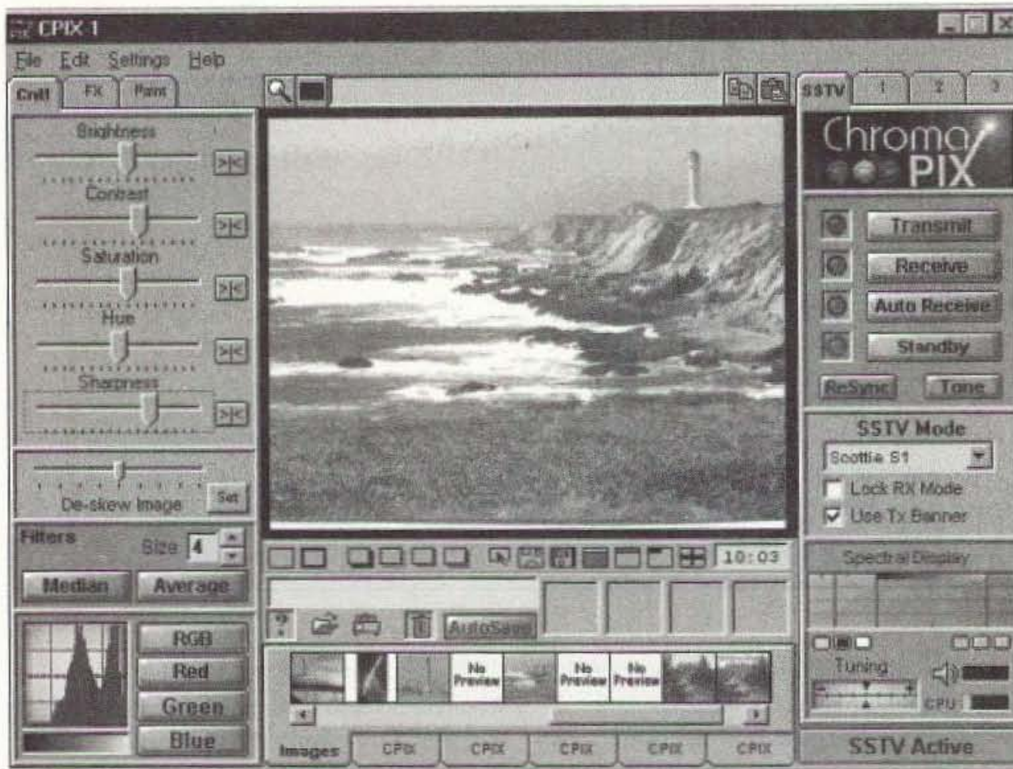
Fig. 1. ChromaPIX screenshot — This is what you see on your monitor. This was an off-the-air shot. The image is one I scanned in using the CSCAN module that comes with the package. I scanned using the option "clipboard." Then pasted to my graphics program and separated the several pics from the album page, then to the image file to be brought up as you see here. On the left are some slider adjusters which I tweaked a little to get the best resolution before this screenshot. The lighthouse in the upper right is still a bit hazy, but that may have been so in real life. The tabs above the sliders open other editing options. At the bottom left is a histogram for the image-keepers who are "pure-in-heart." Directly below the image are options for arranging borders and shading and inserting insets in the image. Below these controls is a well thought out file management system. The right panel is for controlling the interface with the radio, mode selection and tuning indicators. For a full description of all you see here, go to the Web site and download the manual. Won't cost you a dime to give it a look-see. Plus the full-working program can be downloaded for free while you are there. It will run for 30-minute intervals without registration. See The Chart for the URL.
