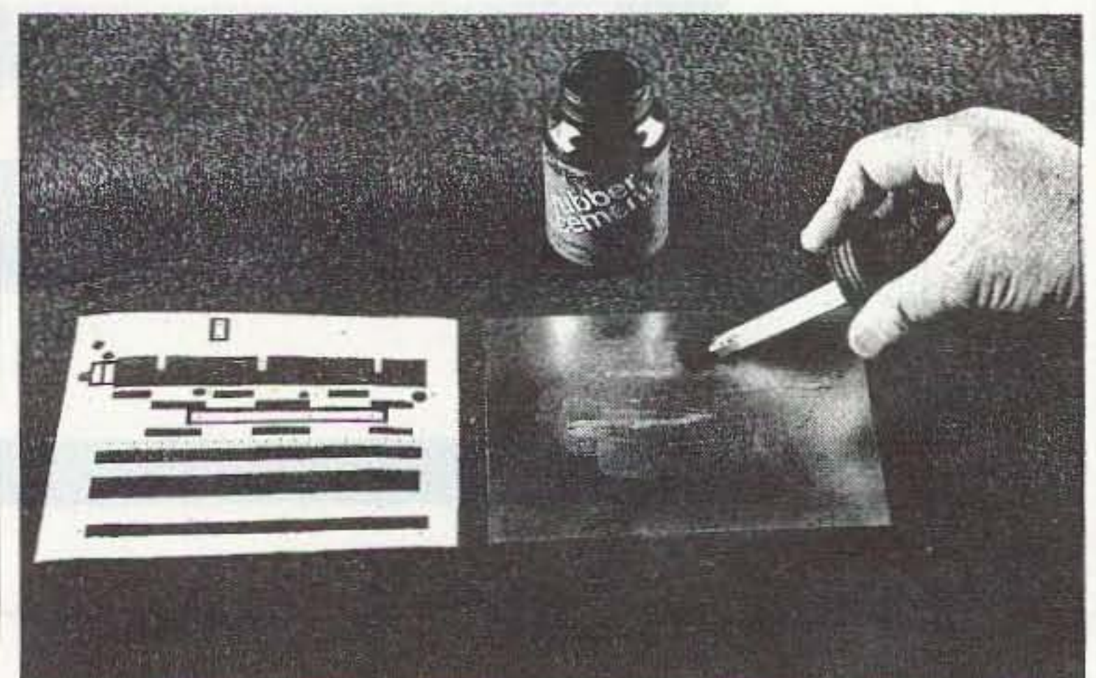
Photo B. The application of rubber cement to the copper surface.
