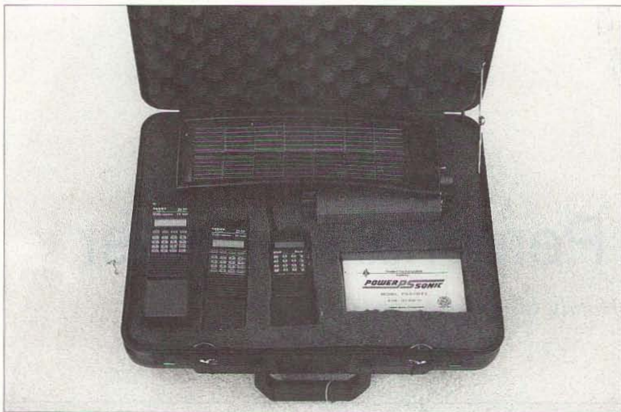
Photo B. The crossband repeater is shown with the battery, the Alinco 580 which is used as the repeater, the two Yaesu FT-470s which are the remote radios, a power supply used for charging the battery, and a solar panel.
