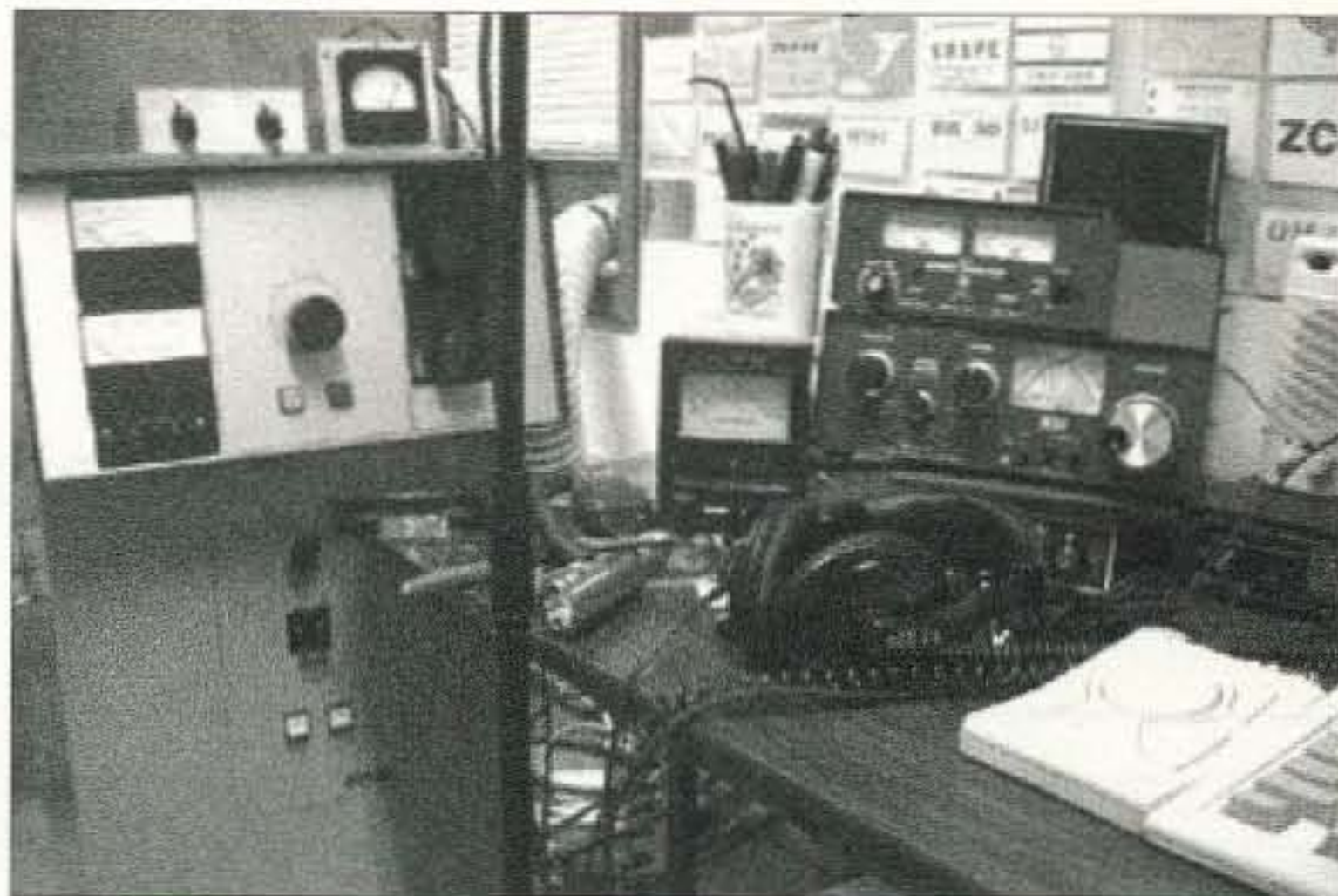
Photo C. Here is my "dB enhancer," a Henry 2k Classic X. I finally broke down and agreed with K7SS that life is indeed too short for QRP.
