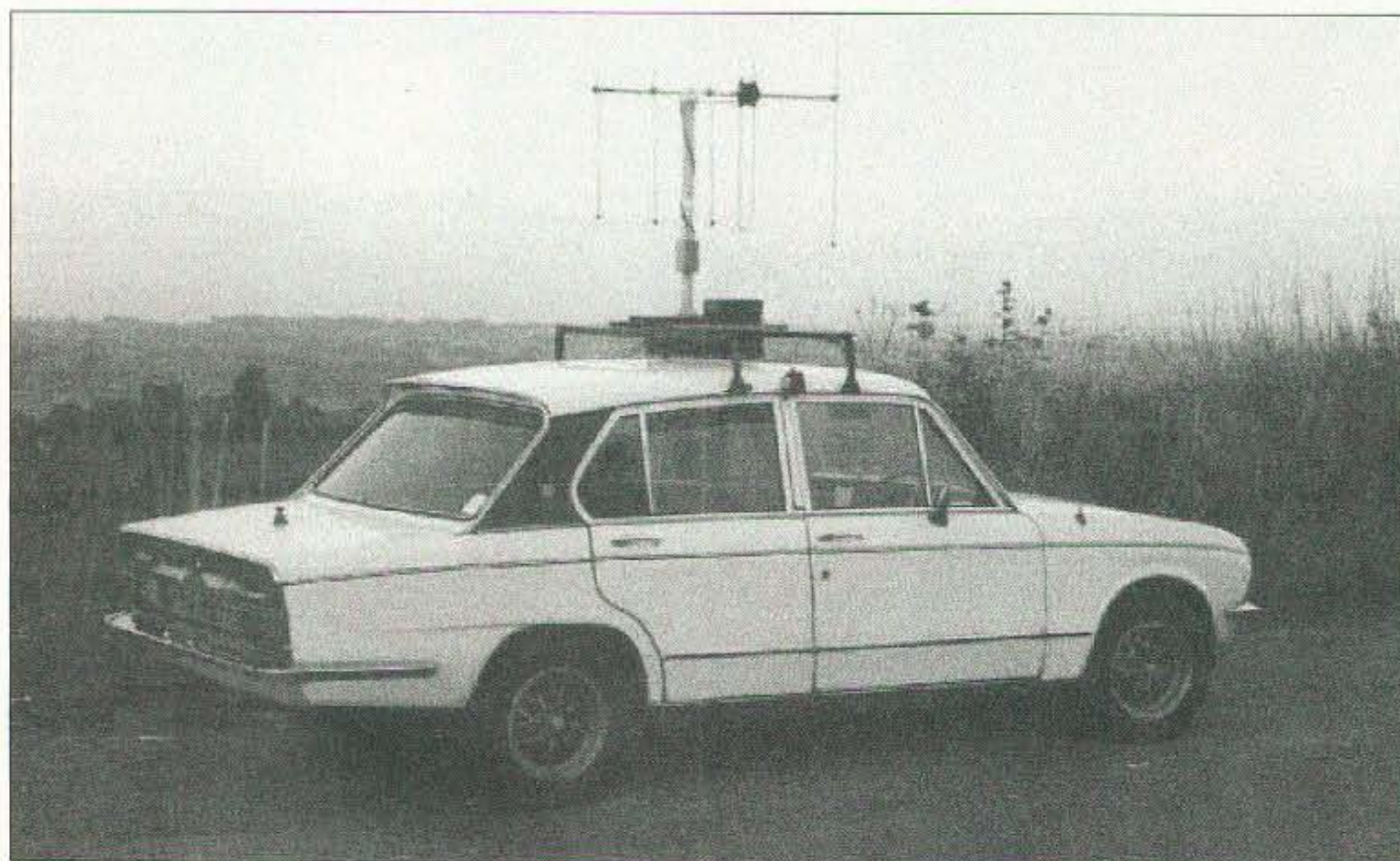
Photo D. John and Dave's foxhunting vehicle with its motorized beam at a hilltop test site. (Photo courtesy of G6UWO)
