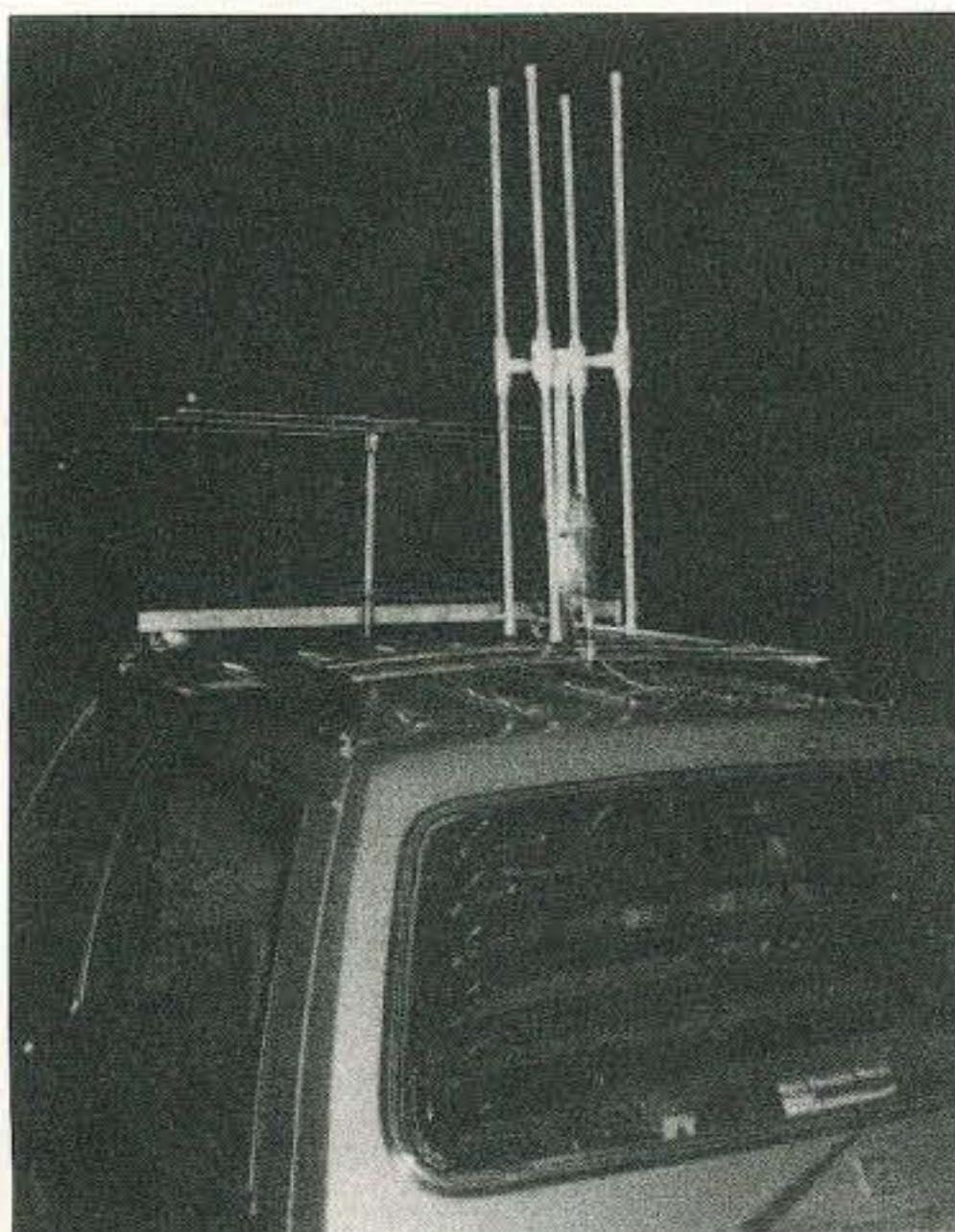
Photo A. The VK3GMZ team hunts on two meters with both a horizontally polarized beam and a modified marine doppler array. (Photo courtesy of Mark Diggins VK3JMD)
