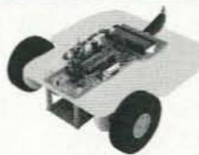
This advanced kit is an 8 x 8" differentially steered base that is excellent for carpet or tiled floor experimentation. It uses the Next Step microcontroller, a BASIC Stamp 2 controller that can use the BS2 or BS2-E (sold separately). A host PC is required to download programs to the robot. This complete kit includes the Rover, programming cable, IR proximity detector, bumper switch kit, and line follower kit.
