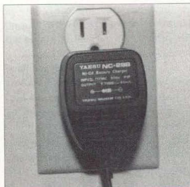
**Photo B.** A wall-wart used as a battery charger for a Yaesu handheld radio.
