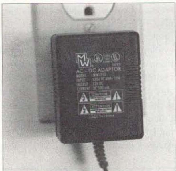
**Photo A.** A typical "wall-wart" power supply.
