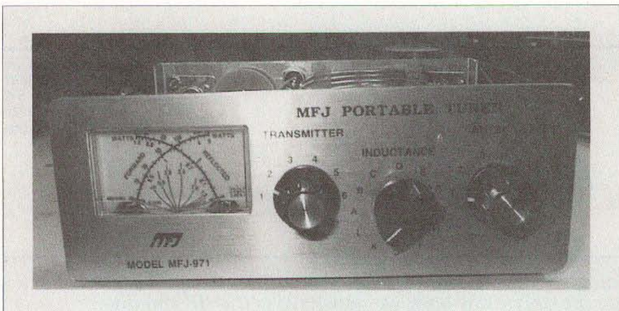
Photo B. A portable antenna tuner is a must for field use. This MFJ 971 is ideal for camping or Field Day use.
