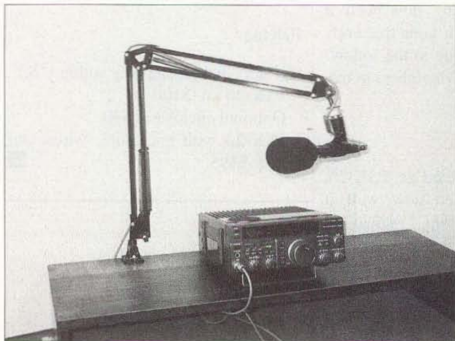
Photo A. The modified architect's lamp holding a Yaesu MD-1.
