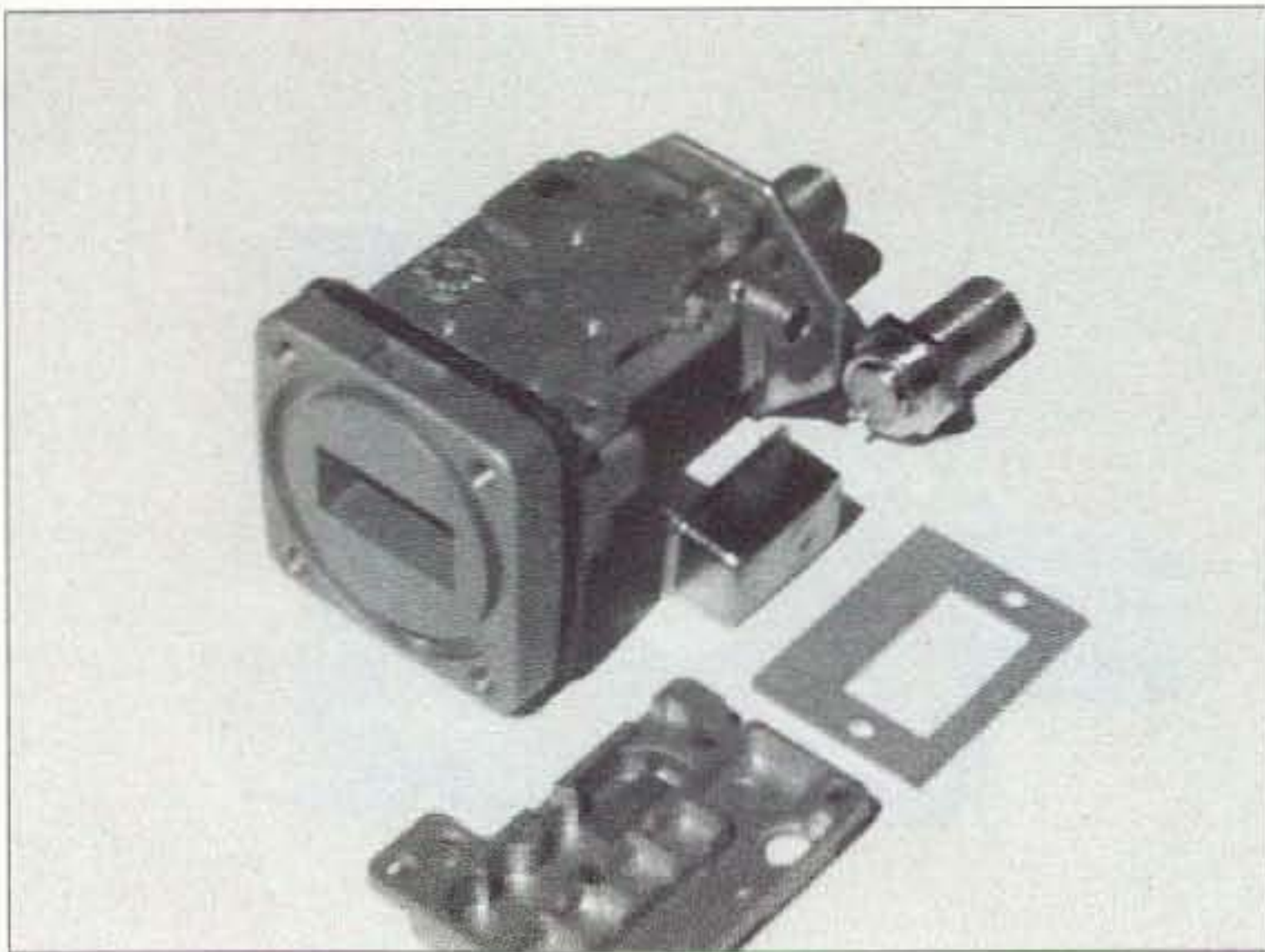
Photo C. Full side view of the Channel Master LNB.
