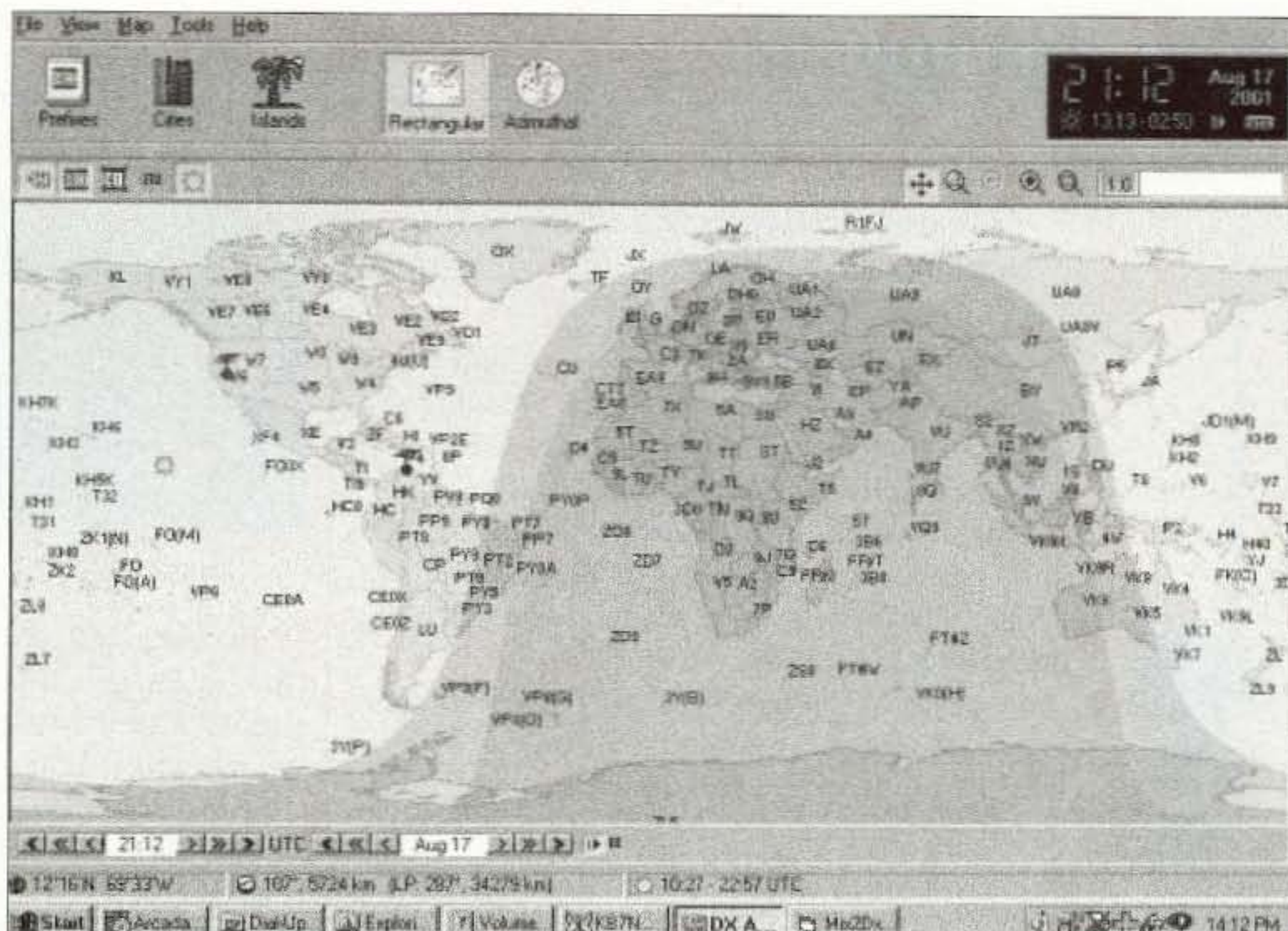
Fig. 2. DxAtlas in action. This is the flat world view of the world atlas. Also available is an azimuthal layout with your station located in the middle and the rest of the world revolving around you. Your choice — you can change it instantly back and forth. The overall size of the panel can be reduced to fit along side your MixW display or you can have them overlap. This view is shown over top and completely covering the MixW 2 display. If you do it this way, you can switch back and forth with the task bar buttons at the bottom. The KB7NO location is indicated by the antenna planted to the left of the W7 in the western U.S. When I double-clicked the PJ2 station in the receive pane in MixW, an antenna showed in the very northern part of South America. By moving the cursor to that point and clicking the mouse the program calculated beam headings and distances in the info box above the task bar. This was taken about 2 p.m. local time and you can spot the location of the sun by the bright (yellow) spot about 1,500 miles SW of the home QTH. You can see the sunrise-sunset indicator covering Europe, Africa, and most of Asia. There are several options for lookup on prefixes, countries, cities, etc., I did not wish to confuse the display with clutter. DxAtlas integrates nicely with MixW 2 with the patch shown by the button at the right of the task bar (Mix2Dx) that can be downloaded free. See text.
