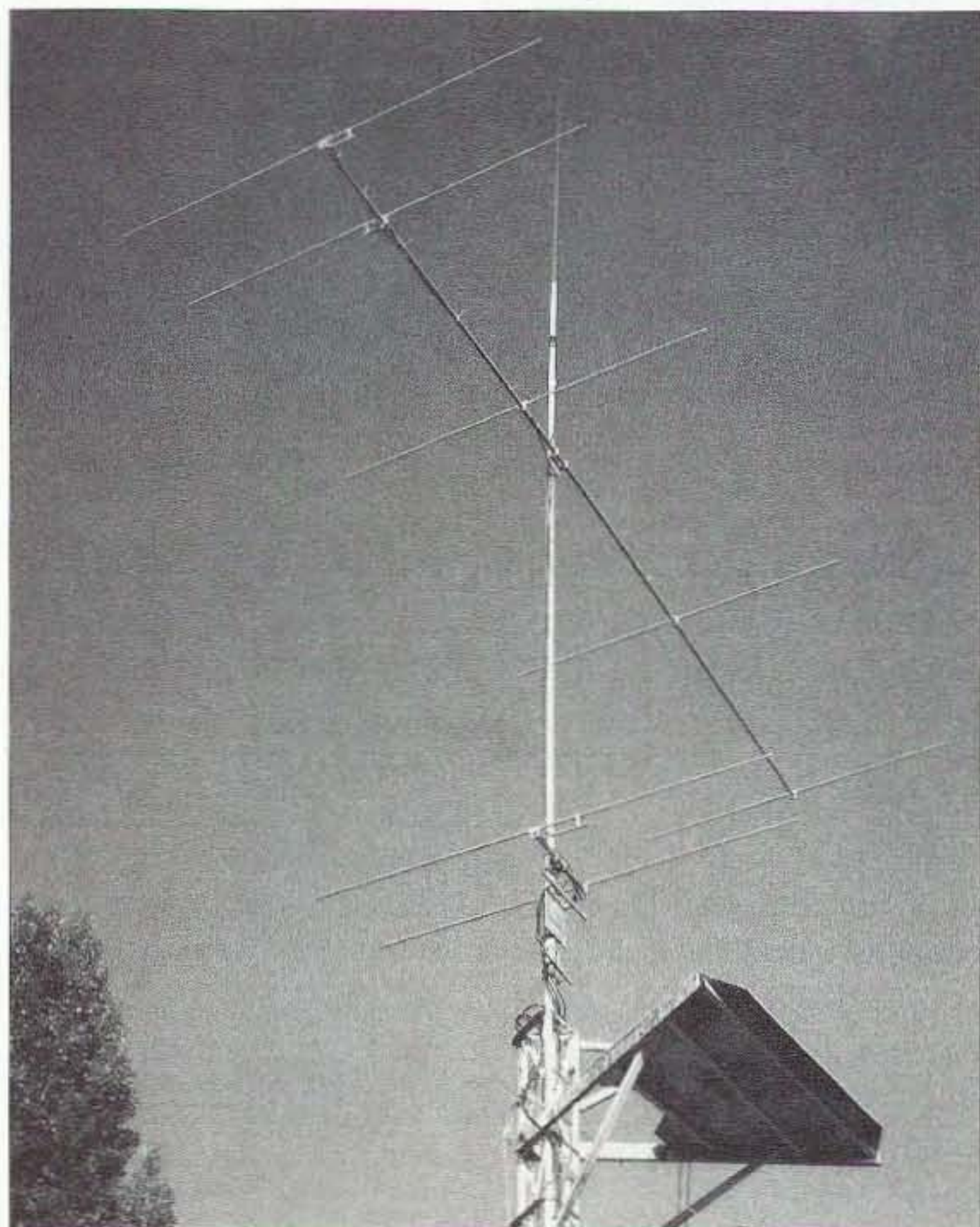
Photo D. 5-over 2-element 6m Raibeams with 1/2-wave vertical on top used as a listening antenna. These two beams can be selected individually or both together in phase. Various configurations are being tried to obtain different angles of radiation individually or phased together, or differences in polarization to create different angles of radiation to compensate for polarization shift.
