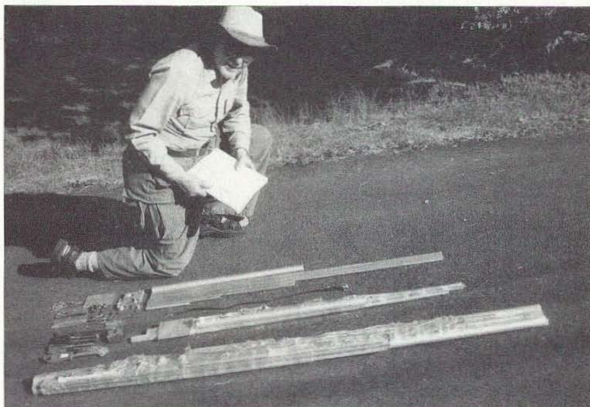
Photo A. The 2x2-element and 5-element Raibeams came neatly wrapped in one box. One 2-element is unwrapped. The bag of hardware and tools I added are shown. These were assembled and installed in one afternoon.
