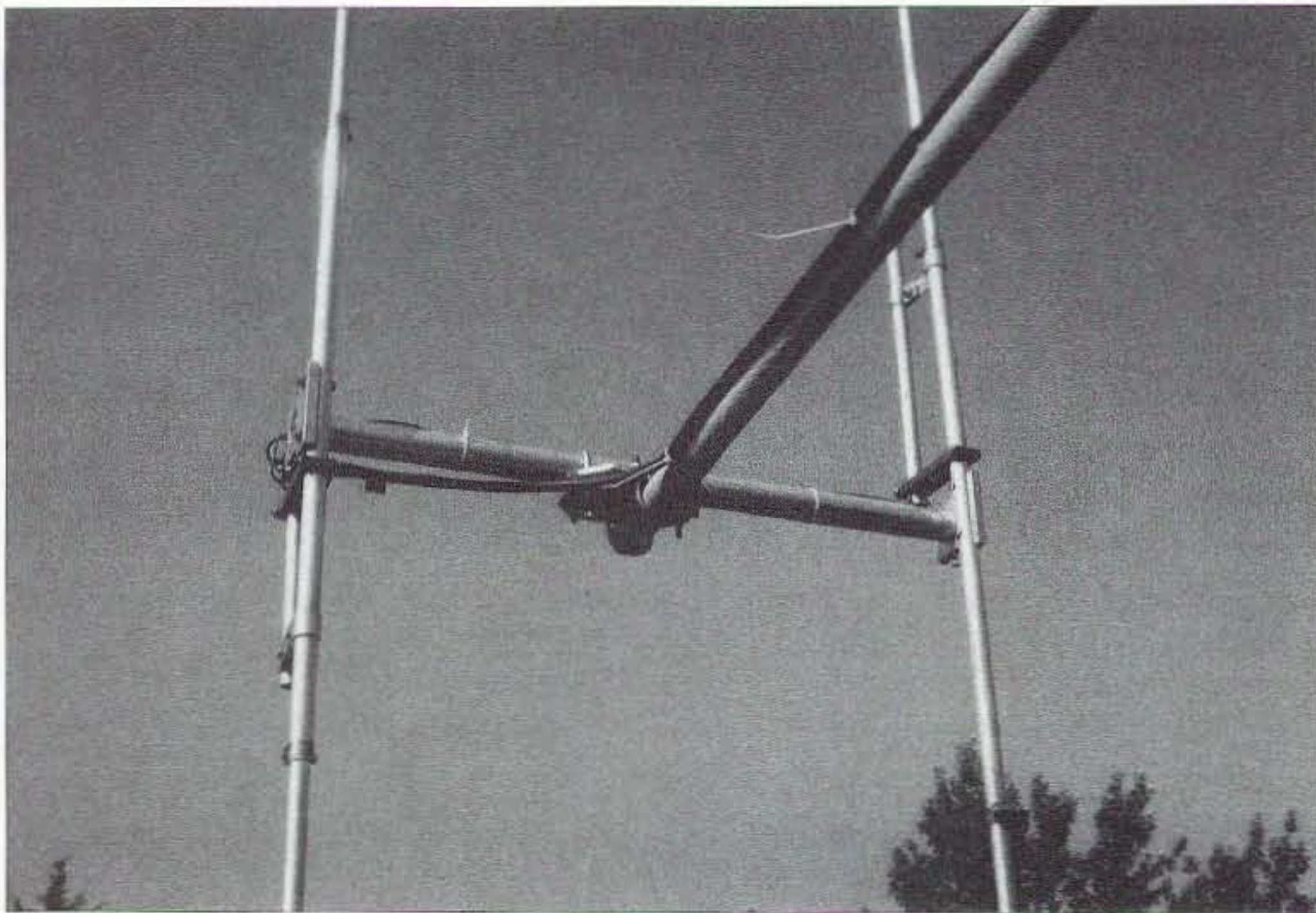
Photo C. 2-element 6m Raibeam. Both elements are driven, have very good patterns, weigh just 3 pounds each.
