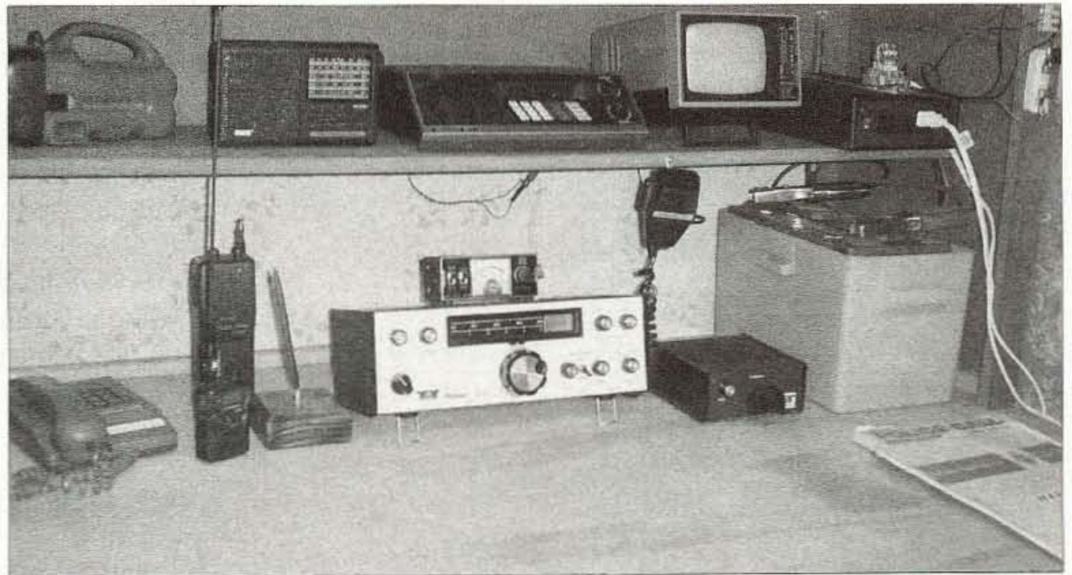
Photo B. The emergency station: The Argonaut, HTs for 2 meters and CB, a scanner, 4" television, all-band receiver and 600-watt inverter, all powered from a 12-volt deep-cycle battery. The Microwind keeps it charged and ready!
