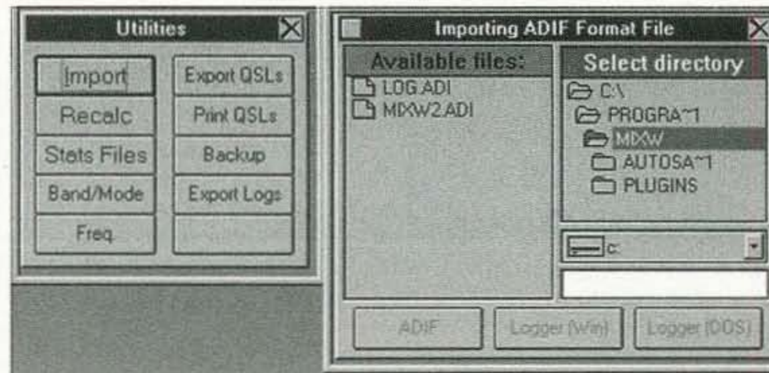
Fig. 2. Logger import — These are the windows referred to in the article concerning importing an ADIF log into Logger. The "tree" referred to in the article is shown to the right. This may be the only place, if you are unfamiliar with file structure, that will offer resistance. In this case, the highlighted MixW directory or folder is where Logger will seek an ADIF file and post any of these files it finds to the immediate left window. See article for procedure.
