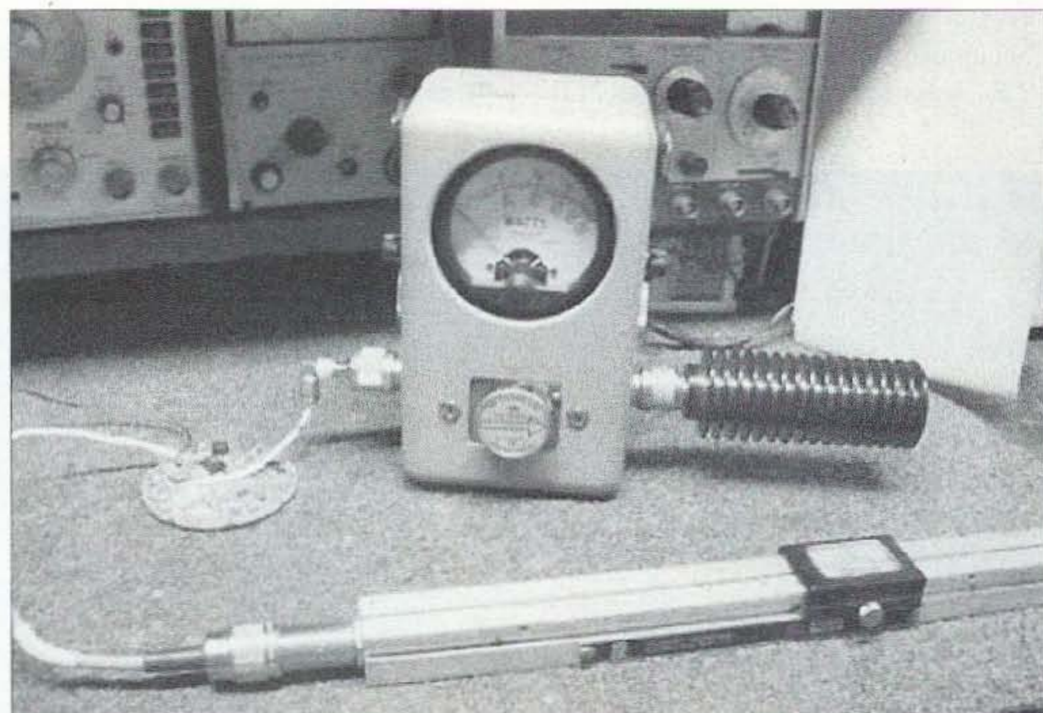
Photo C. The test and evaluation setup. Nothing complex, just the drive source for low power tests with the Wavetek 2001A sweeper set at 1296 MHz zero dB RF drive for first cut test. Detector is the Bird model 43 power meter. Line terminated into a 50 ohm DC to a 12 GHz 40 watt coaxial termination.
