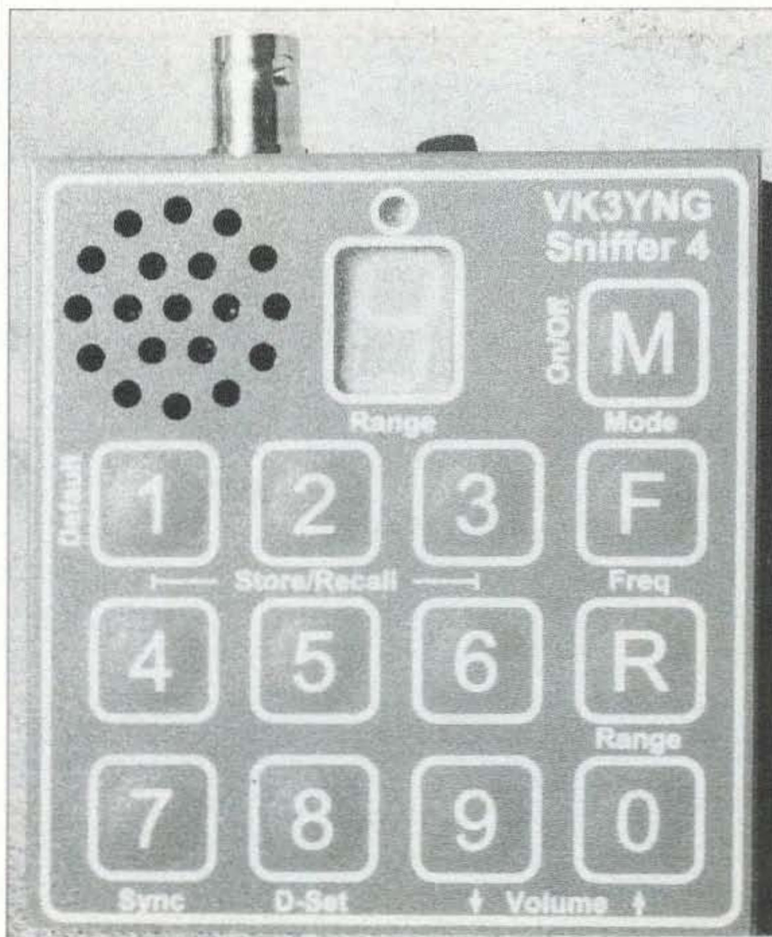
Photo C. Sniffer 4 is built into a rugged epoxy case with a membrane keypad to make it relatively impervious to rain. But you have to take out four screws to change the batteries. (Photo by Joe Moell KØOV)
