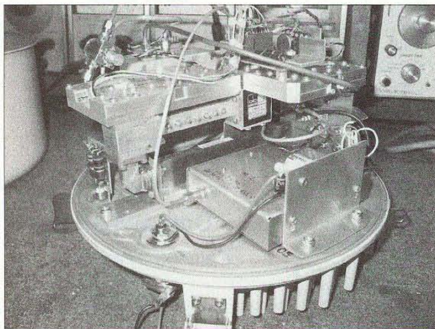
Photo A. Side view of Pecom 24 GHz converter. Waveguide circulators shown with left top transmitter board, right receiver board, and bottom center IF synthesizer at 2640 MHz in aluminum container. Main system controlled by 1/2 frequency LO at 10560 MHz synthesizer. Conversion by Sam K6VLM.
