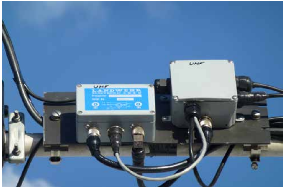
Figure 5: Photo showing the UHF Polarity relay box and the UHF preamp mounted on a panel attached to the cross boom. This arrangement minimizes the loss between the antenna and the preamp.
