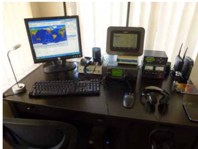
Figure 7: A complete station that can be operated locally or remotely and is XYL (W8ZJB) approved. The 12 VDC switching power supply and UPS are under the desk.
