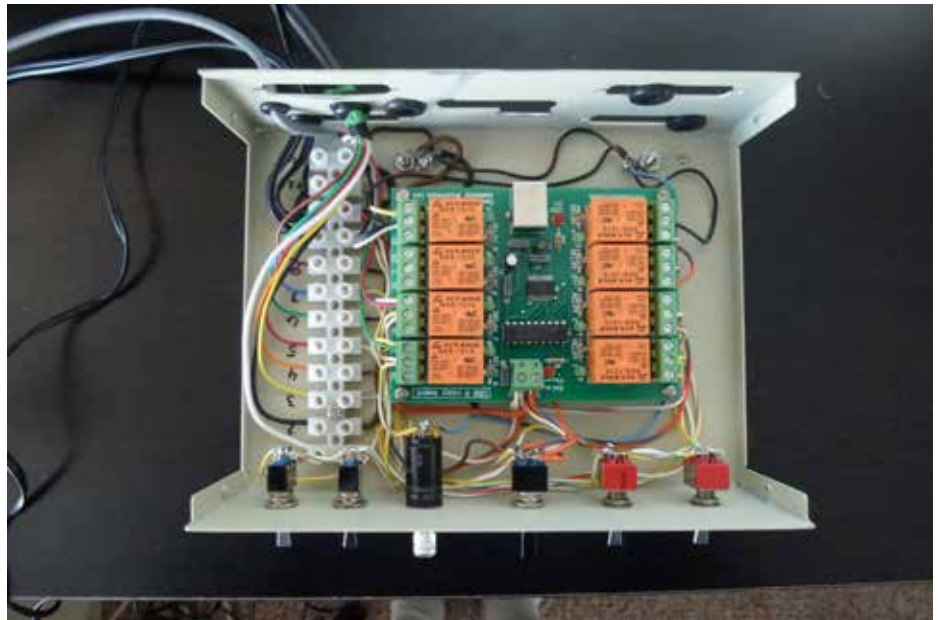
Figure 6: Denkovi USB relay control board used to control functions such as polarity, preamp, radio/rotor AC power etc. Software is provided to customize the control/appearance on the screen. Switches can be used when operating locally.
