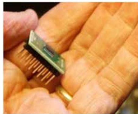
Figure 4: ADS7828 A/D converter mounted on adapter board.
