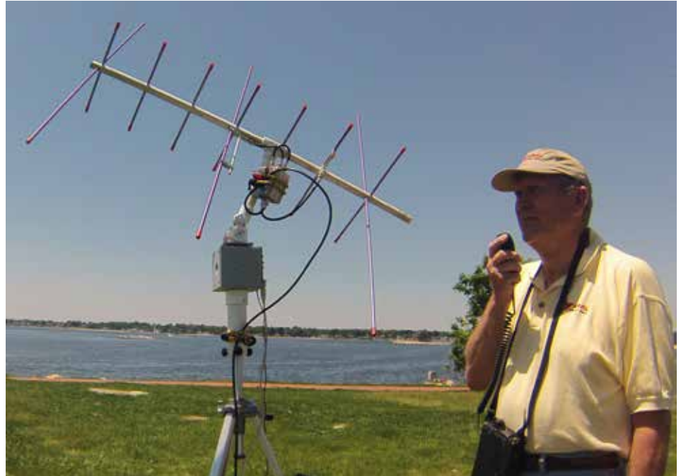
The author shown with his original WRAPS rotator project described in the January 2014 QST . This article shows how to add the capability to modify WRAPS with two beams and add the capability for circular polarization.
