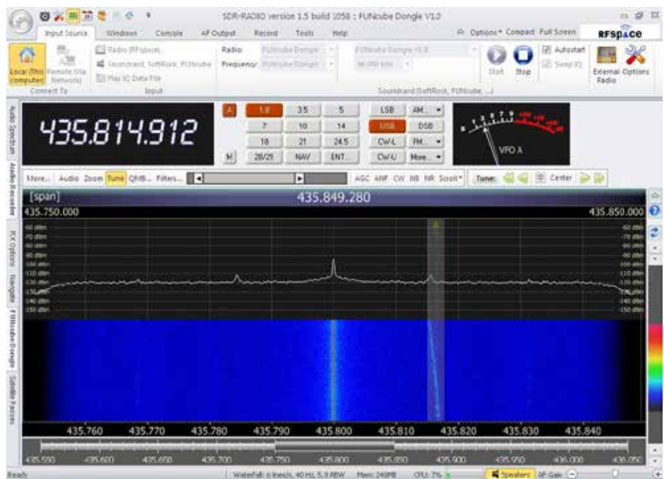
Hector’s second configuration using the FUNcube Dongle and SDR-Console software.
