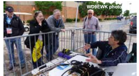
Michael, KD8QBA, shown explaining the satellite station prior to a satellite pass. The dual-FT817 radio configuration is visible. One radio was used for the uplink and the second radio was used to receive the downlink providing full-duplex operation.
