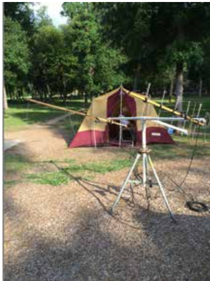
Photo 4: The 2 meter tape measure yagi that saved the day at K8MR.
