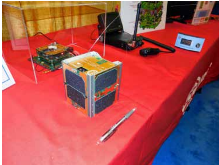
The AMSAT engineering area this year once again included an updated engineering model of the FOX-1A satellite along with a working model of the satellite's internal housekeeping unit. This engineering prototype was also transmitting greetings from FOX-1A to passersby who tuned their HTs to 145.920 MHz.
