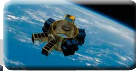
Spaceflight's SHERPA will deploy multiple cubesat payloads on-orbit
