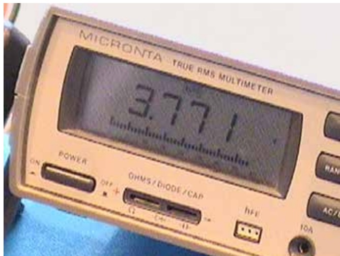
Photo 7 – The Fox-1 Cam view of the DVM during a measurement of the battery voltage
