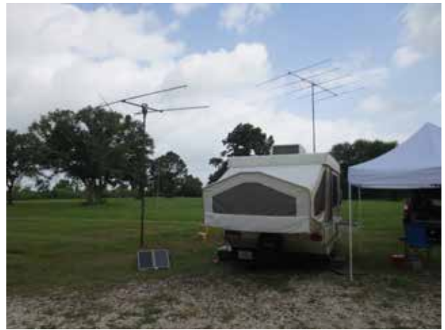
Photo 15: Satellite antennas on the left and the 6M Yagi on the right at W5MSQ.
