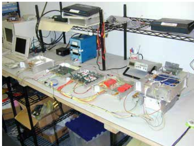
Photo 1 - AO-51 "flat sat" model under test
