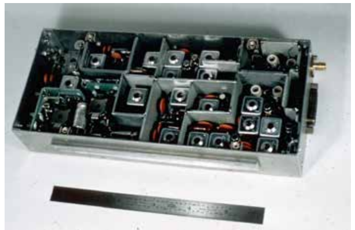
Completed module of the 2-to-10 meter transponder.
