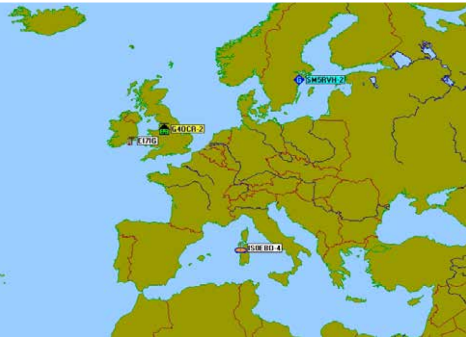
Figure 4. Image capture from UI-View32, 1st April 2014 showing EI7IG and IS0EBO Internet gates in the Republic of Ireland and Sardinia and the author's own station. A packet addressed to EMAIL was received at both remote stations and gated to the Internet, reaching the author's work email address within a few minutes
