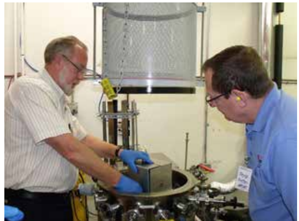
Fox-1A shown under preparation for thermal-vacuum testing with (L-R) Steve, the Qualtest operator, and Jerry Buxton, N0JY.
