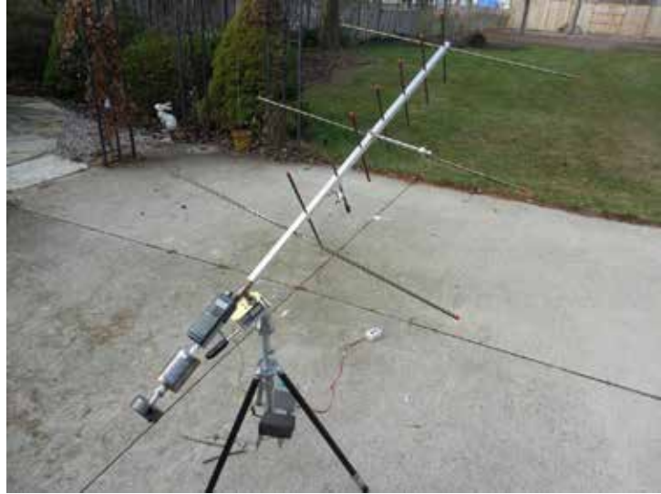
Figure 1. Earth station shows fully operational earth station with radio mounted on bracket and attached to motorized Gizmo with control box
