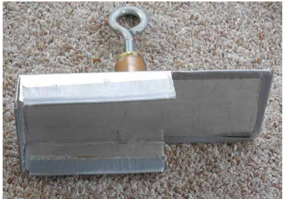
Figure 7. Simple bracket made from 0.025 aluminum sheet bent in a vise
