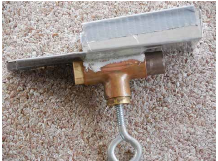
Figure 8. Radio bracket with Gizmo type of attachment to put it on counterweight shaft.
