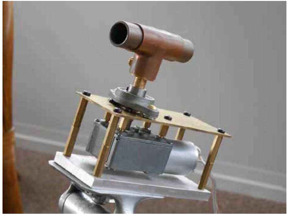
Figure 5. Motorized Gizmo showing worm gear 12 volt motor and 8 mm pillow block for extra support
