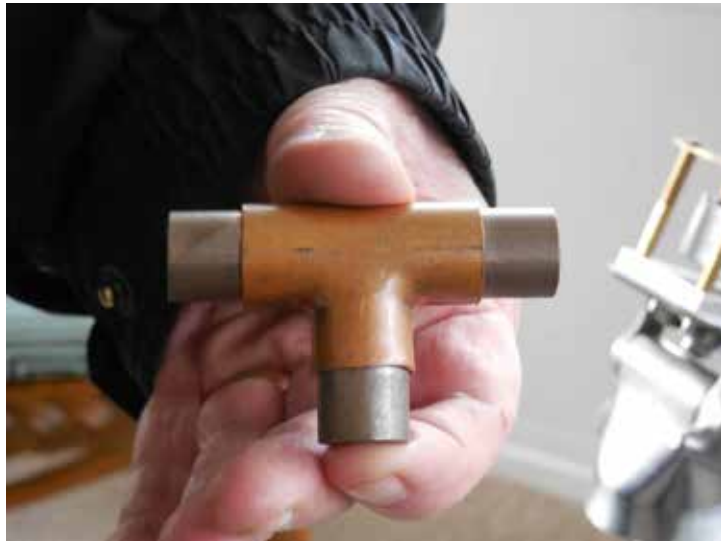
(left) Figure 2. Original Gizmo with bronze bushings
