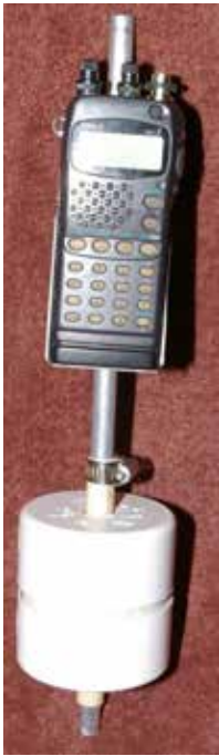
Figure 4. Radio and counterweight mounted on main shaft before assembling and mounting on tripod
